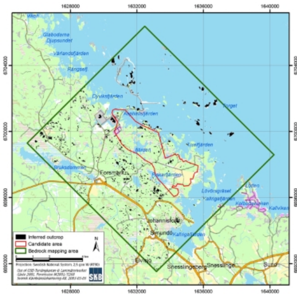
Figure 5-1. Inferred outcrops and sites where the Quaternary cover is less than 50 cm thick.
