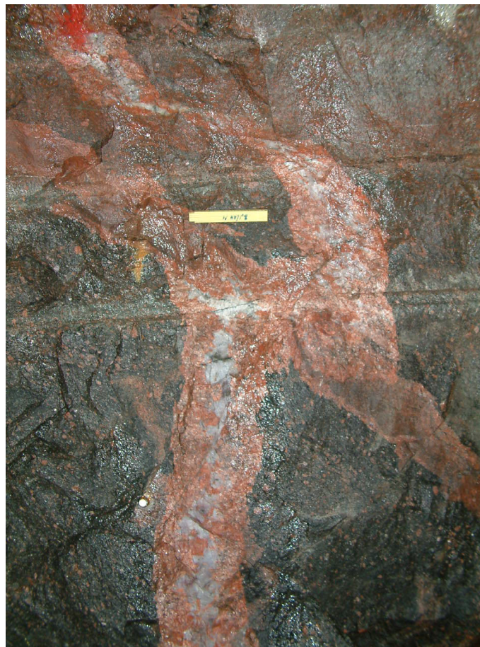
Figure 6: Pegmatite dike crosscutting a fine-grained granite. Host rock is unaltered Äspö diorite.
