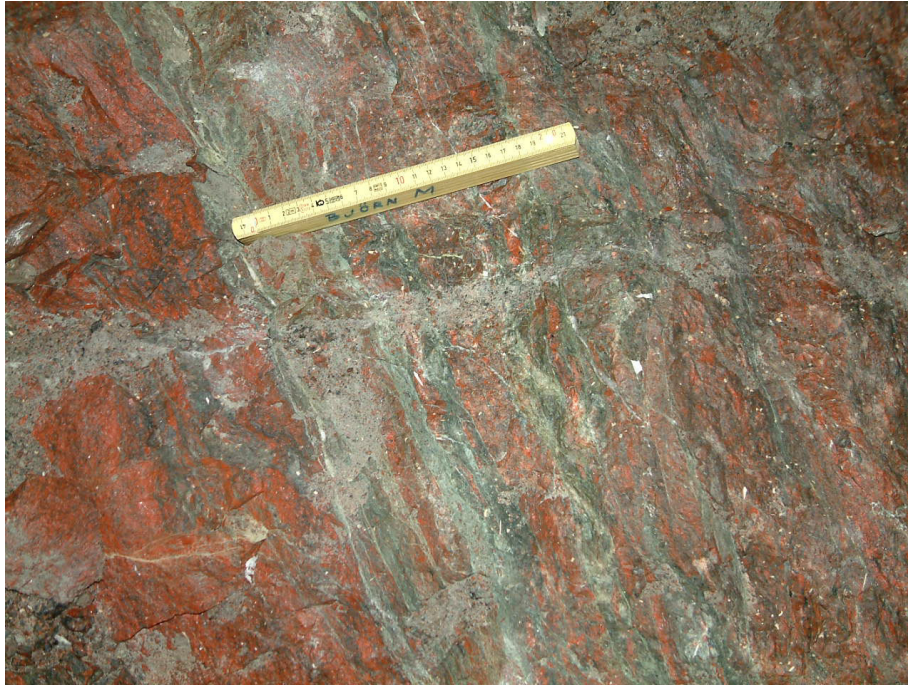
Figure 5: Mylonite in TASQ. This rock has originally been a Äspö diorite, as seen in the transition from mylonite to fresh rock.
