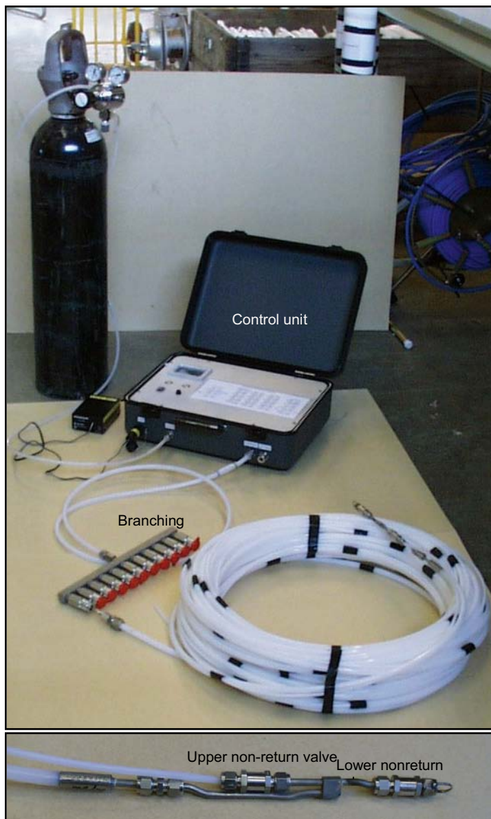
Figure 2-7. Control unit with branching and one pair of pumping tube connected. The smaller picture shows the Y-connection with upper and lower non-return valve.
