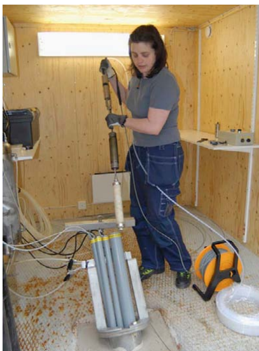
Figure 2-9. Lowering of equipment in the water standpipe in order to pump water from the borehole section. From the bottom: filter, small inflatable packer and pump.
