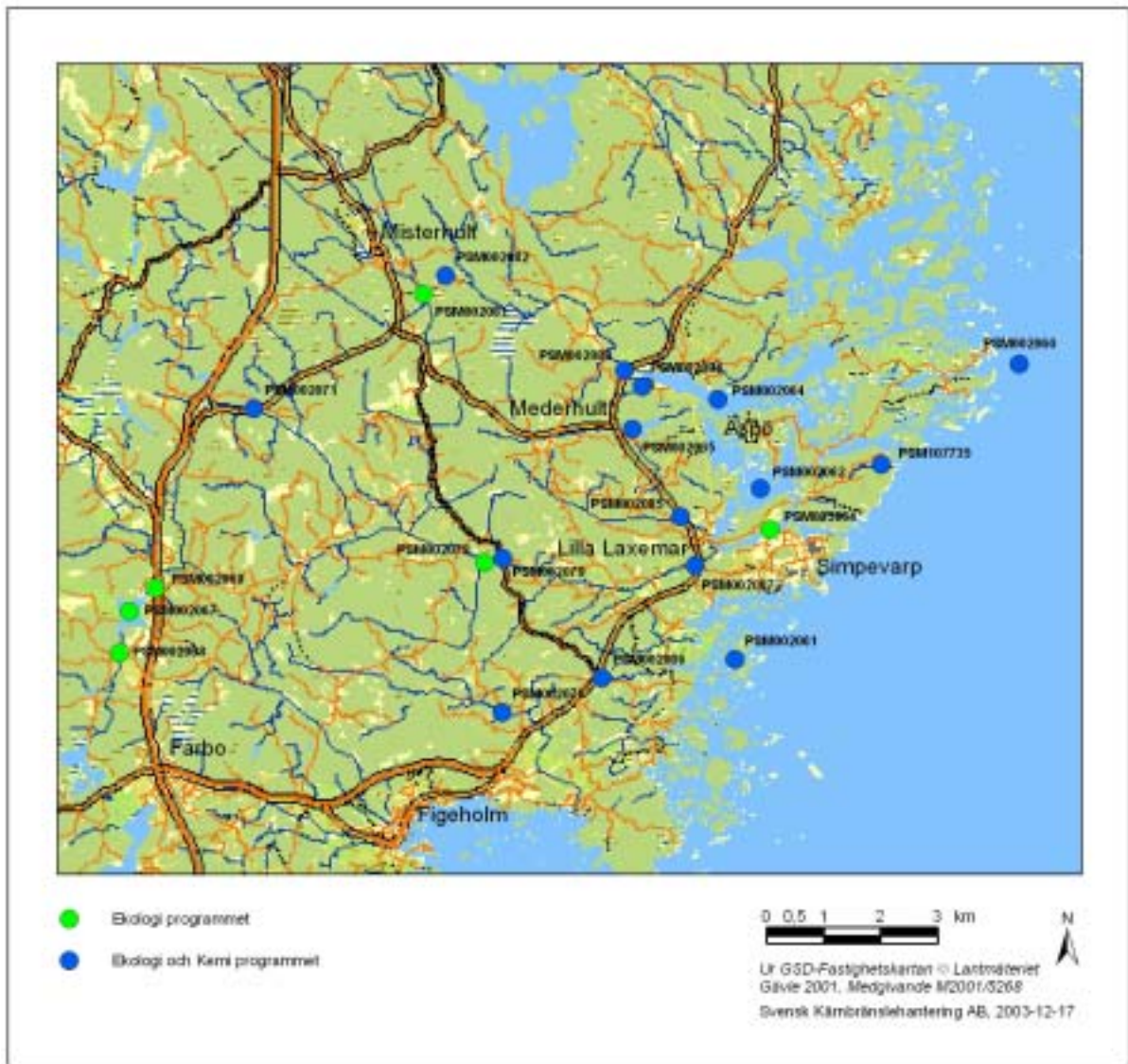
Figure 5-3: Surface water sampling locations at Simpevarp.
