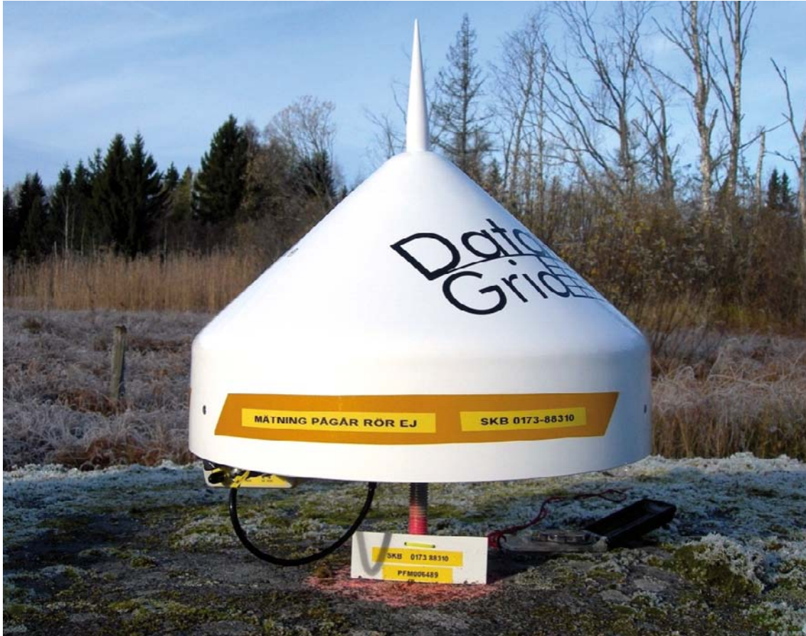
Figure 3-1. Sample station with choke ring antenna and GPS receiver mounted to the lower left. The station in this picture is PFM006489, but all sites have identical hardware (and firmware). They are mounted on a short steel rod anchored in the rock for good mechanical and thermal stability. However, the low mounts increase the demand on the GPS environment. The antenna radome and pin are designed to protect the active components of the antenna and discourage birds and other small animals from lodging on the antenna. A second cover provides additional protection between measurement campaigns.
