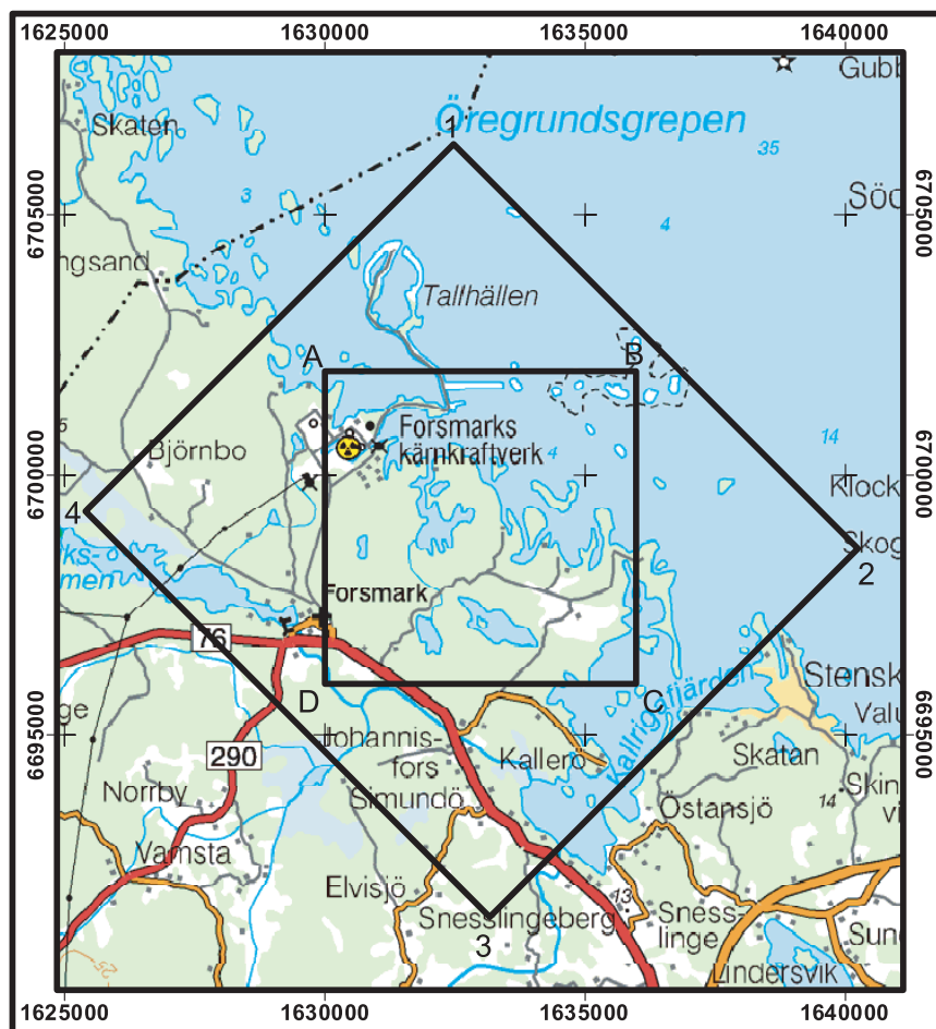
Figure 1-1. Area covered by geophysical measurements from helicopter. Measurements are performed along north-south lines in the large diamond shaped area and along east-west lines in the smaller square area. The position of the DC cable can be seen in Figure 2-2.
