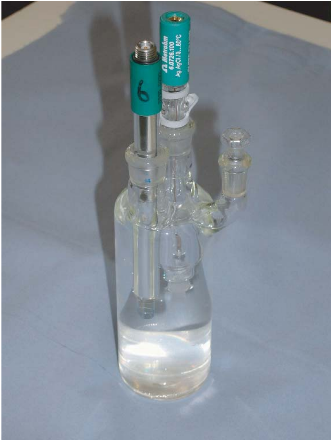
Figure 2-1. Photograph of cell used for testing effect of di-butyl-phthalate on test solution.
