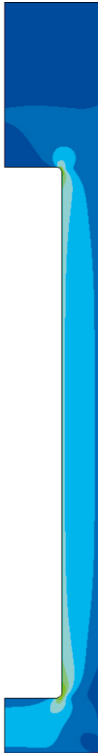
Figure 9-7. Degree of mobilized strength Q_r in the buffer after 100,000 years creep in case 1 ( \sigma_s = 7 \text{ MPa} ) and in case 8 ( \sigma_s = 80 \text{ kPa} ). No backfill. Observe the difference in scale.
