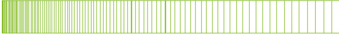
Figure 6-24. 10 m element mesh with 100 elements for the modelling of long small pipes in bentonite. Axial symmetry around a vertical axis 1 cm left of the mesh.
