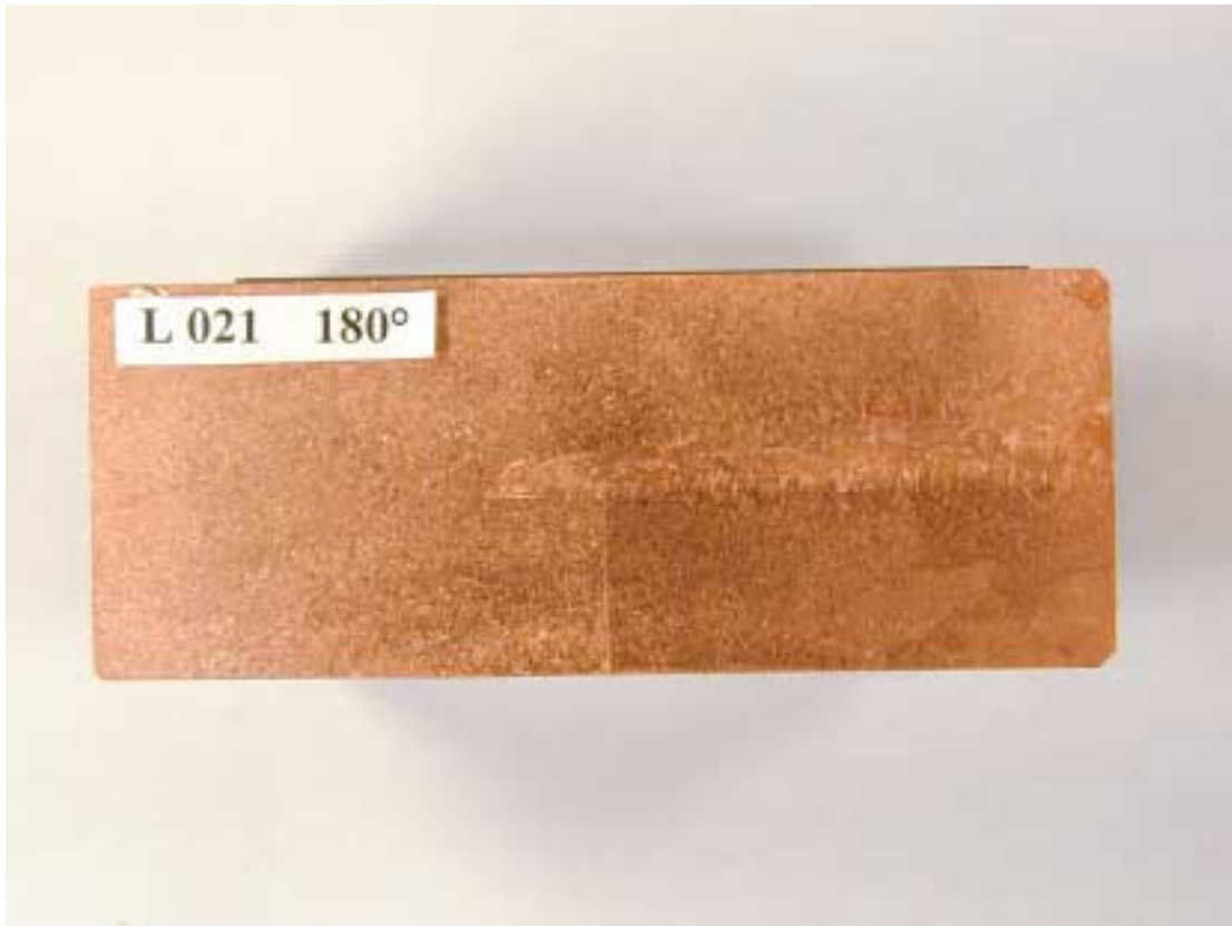
Lid weld no 21: Tip radius 1,2 mm Cathode: HCC1 Q1=1,165A/ Q2=1,470A
