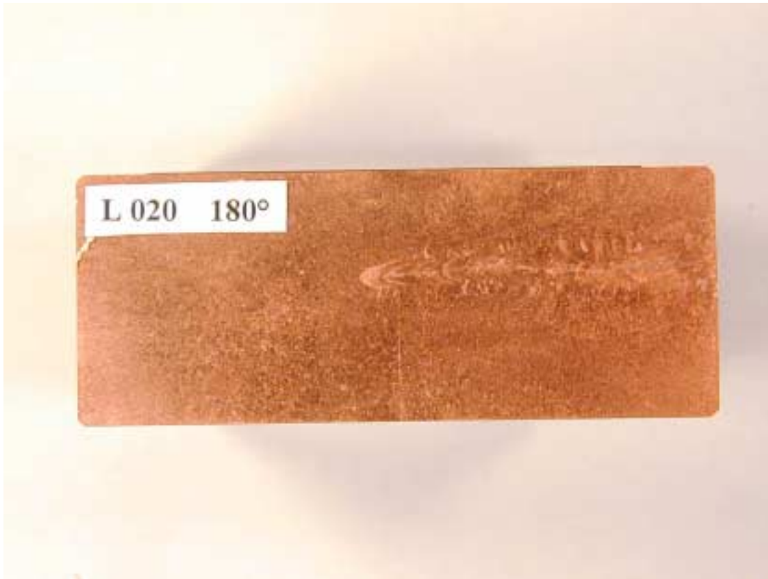
Lid weld no 20: Tip radius 1,0 mm Cathode: HCC1 Q1=1,195A/ Q2=1,470A
