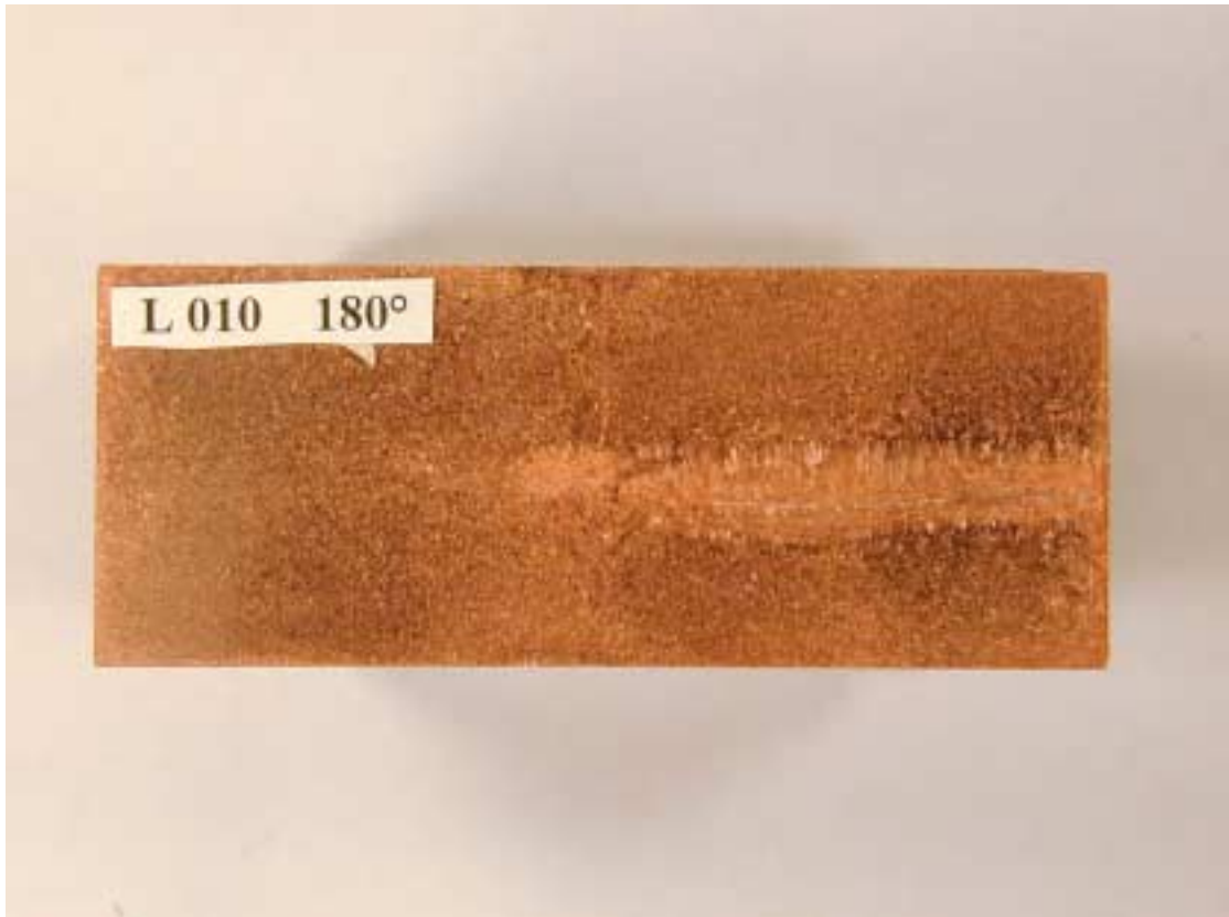
Lid weld no 10: Tip radius 1,8 mm Cathode: HCC1 Q1=1,200A/ Q2=1,450A
