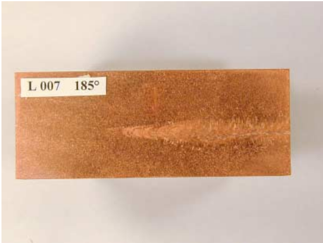
Lid weld no 7: Tip radius 1,6 mm Cathode: HCC1 Q1=1,200A/ Q2=1,500A
