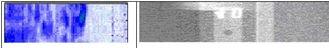
Figure 11: Ultrasonic C-scan of slope in region 0–2,3° of weld 14. Figure 12: X-ray image of slope in region 0–2,3° of weld 14.
