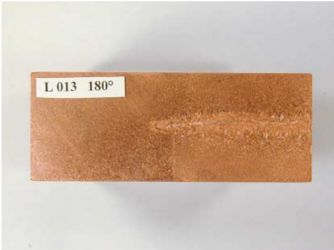
Lid weld no 13: Tip radius 1,8 mm Cathode: HCC1 Q1=1,195A/ Q2=1,415A
