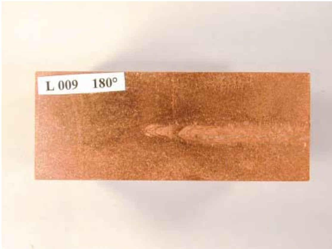
Lid weld no 9: Tip radius 1,8 mm Cathode: HCC1 Q1=1,200A/ Q2=1,450A
