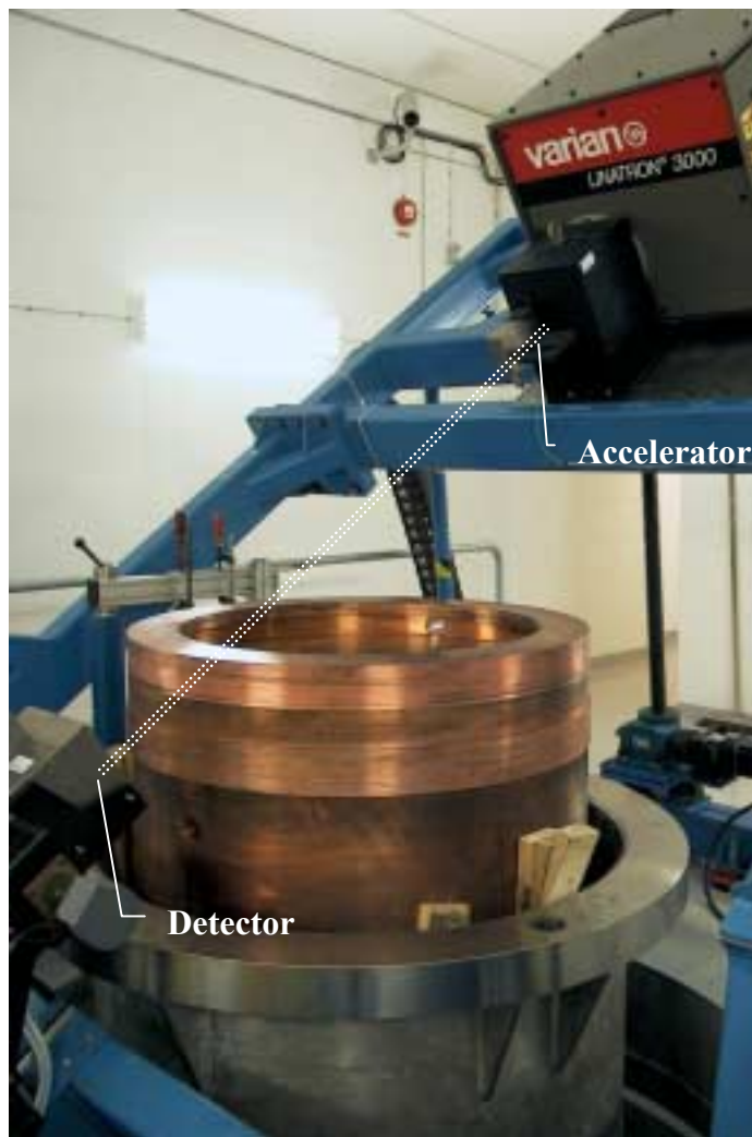
Figure 3: X-ray equipment for inspection of the electron beam welded lid.
