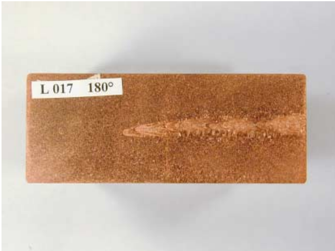
Lid weld no 17: Tip radius 1,2 mm Cathode: HCC1 Q1=1,195A/ Q2=1,410A
