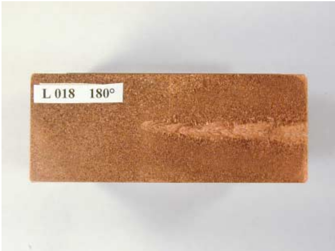
Lid weld no 18: Tip radius 1,4 mm Cathode: HCC1 Q1=1,195A/ Q2=1,410A
