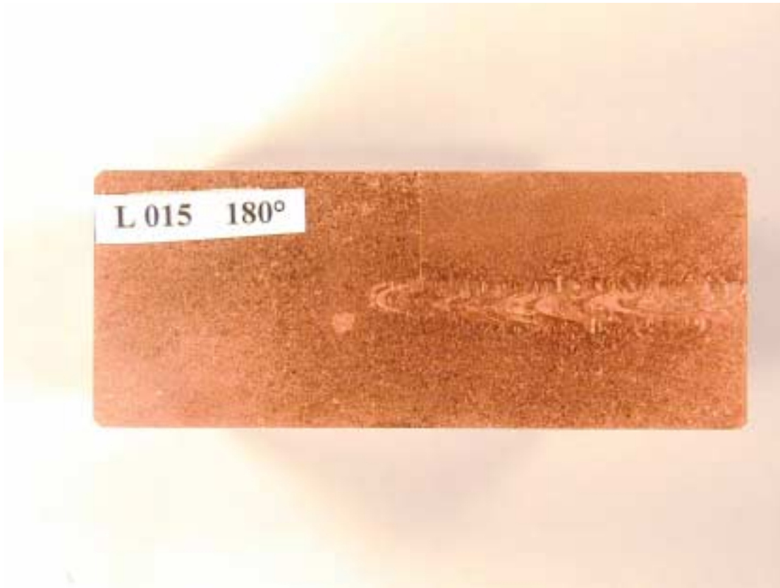
Lid weld no 15: Tip radius 1,8 mm Cathode: HCC1 Q1=1,195A/ Q2=1,410A
