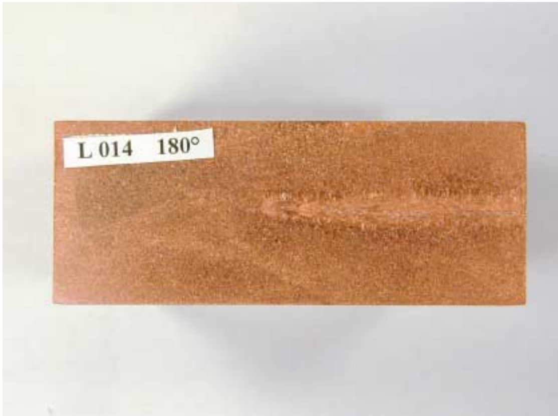
Lid weld no 14: Tip radius 2,0 mm Cathode: HCC1 Q1=1,195A/ Q2=1,410A
