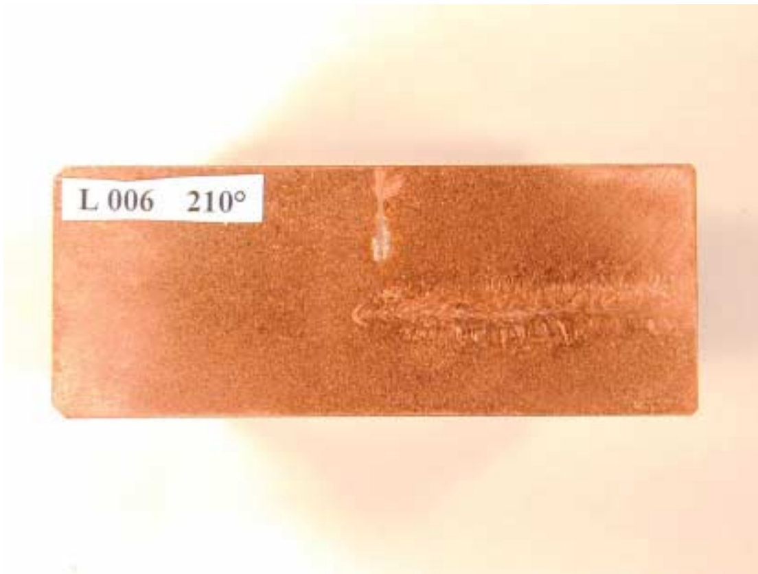
Lid weld no 6: Tip radius 1,5 mm Cathode: HCC1 Q1=1,200A/ Q2=1,450A
