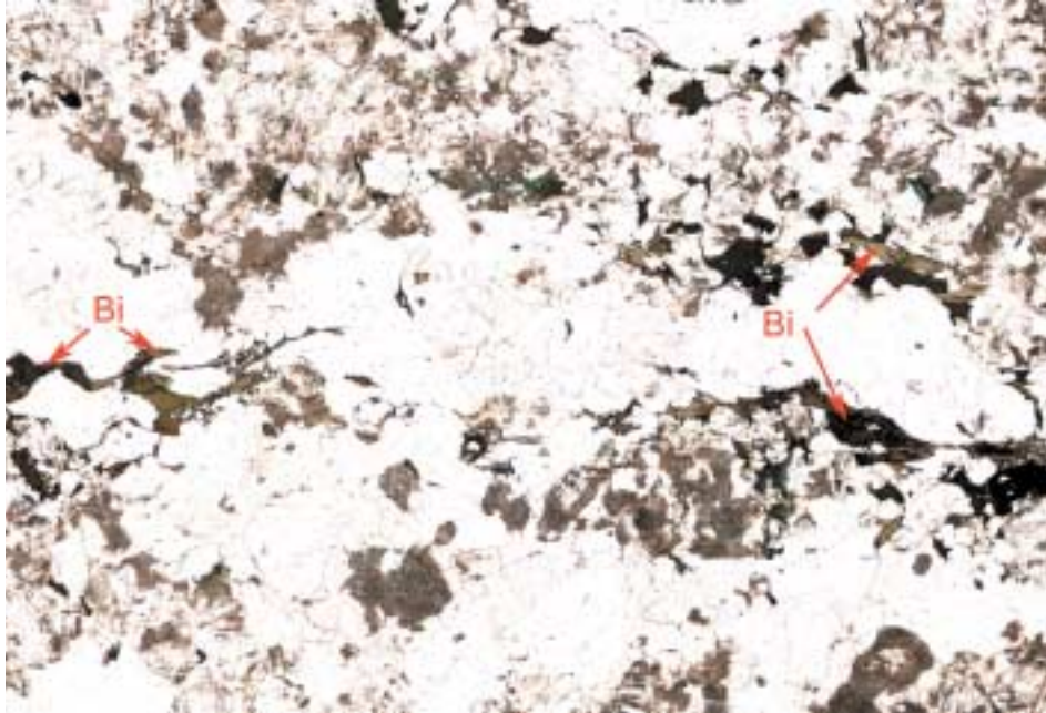
a) Ductile deformational fabric defined by elongate quartz domains (clear, 2–3 mm thick areas), feldspar domains (plagioclase feldspar, partly with a “dusty” or “stained” appearance), and oriented grains of biotite. Width of view = 17 mm.
