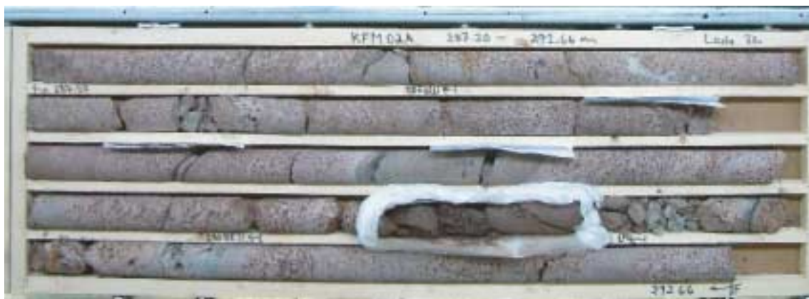
Figure 1-2. Photographs of the KFM02A drillcore showing well-preserved (a, upper picture) and strongly altered (b, lower picture) metagranite. Note the incoherent section in amphibolite at c 291.0–291.5 m. Photographs taken by Alf Sevastik.
