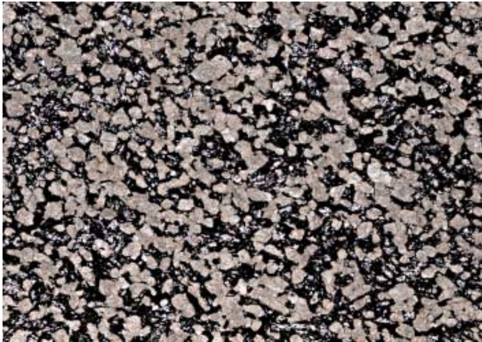
a) Overview shows that the altered amphibolite consists of stained plagioclase feldspar and opaque-looking aggregates with interstitial quartz. Width of view is c 20 mm.
