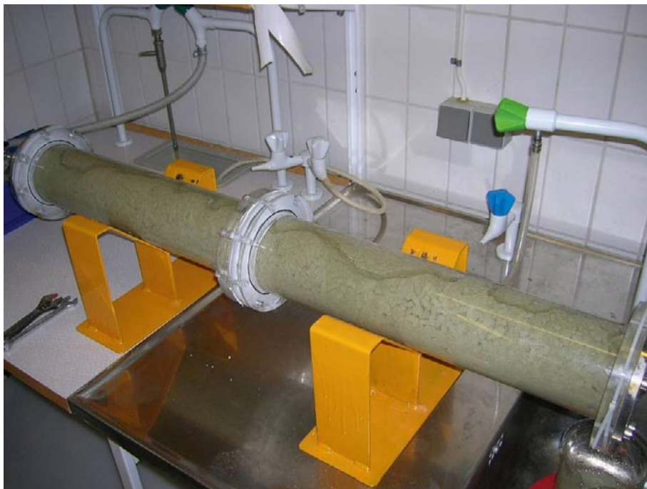
Figure A5-2. The water is flowing in one channel situated at the top of the test tube.
