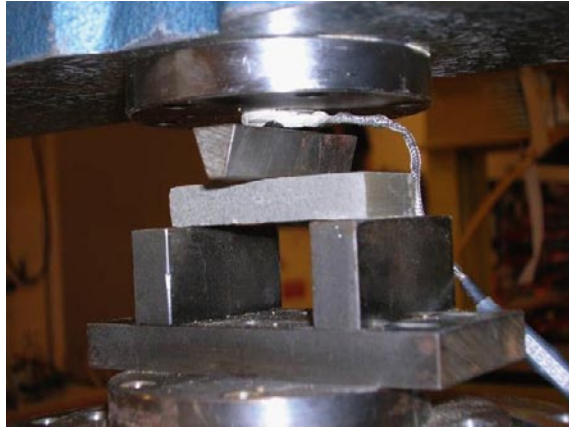
Figure 5-8. Test arrangement for determination of the tensile strength.
