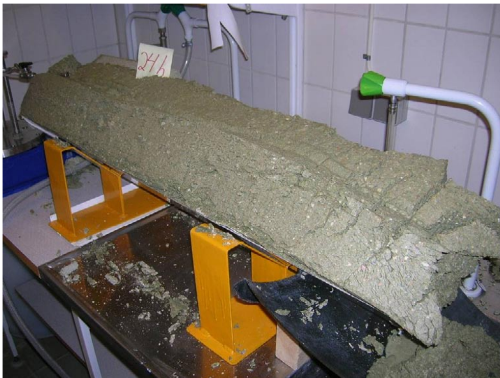
Figure A2-2. Block erosion test with 0.01 l/min and 1% salt in the water. It was not possible to measure erosion depending on the fact that with this rather low water flow the blocks had time to suck up all water; swell and prevent all flowing of water. The result was the same for the test with 0.01 l/min and 3.5% salt in the water.
