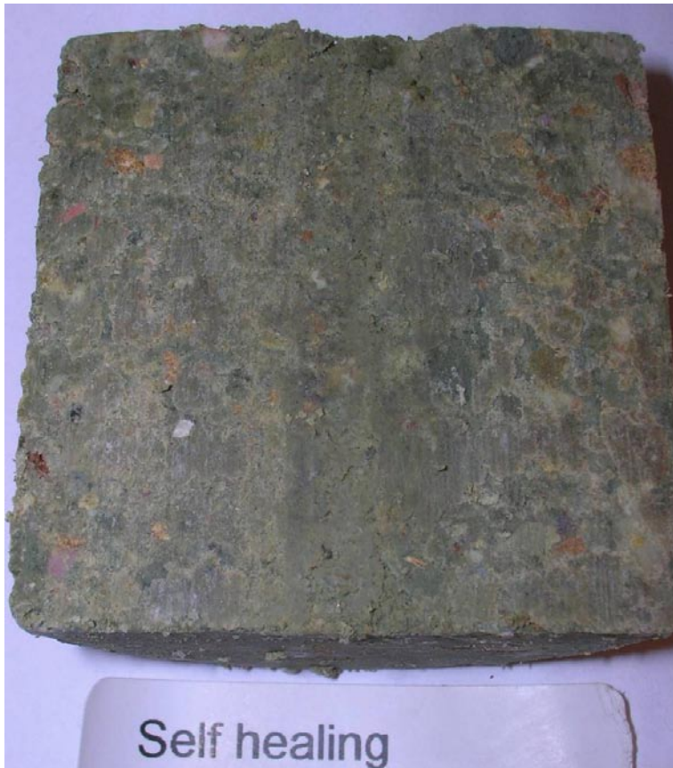
Figure 8-3. After finishing the tests the specimens were cut in the middle along the cylinder. Note that it is still possible to see tracks from the drilled hole. The photo shows the sample with a dry density of 1,345 kg/m 3 and saturated with water with 1% salt.
