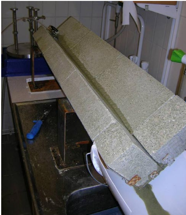
Figure 7-2. The blocks were placed in a steel profile. A constant water flow was applied in one end and the amount of eroded material in the other end was measured. The photo shows the start of the test with a water flow of 0.1 l/min and with water containing 3.5% salt.
