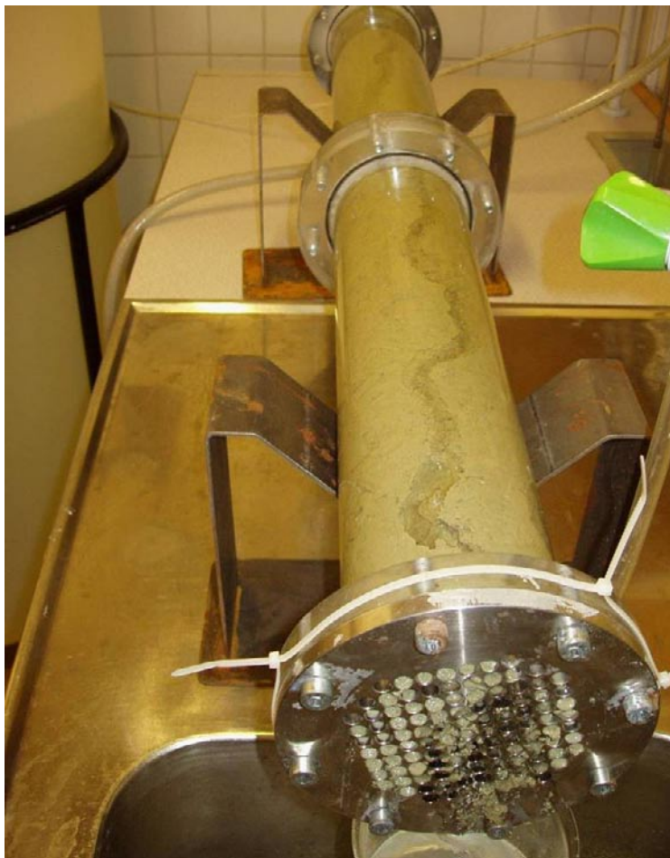
Figure A3-2. After a few hours, all water is flowing in one clear channel.
