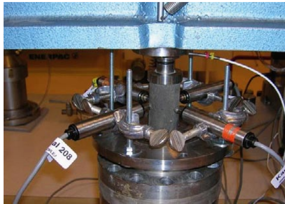
Figure 5-4. Test arrangement for determination of Young's modulus and the Poisson's ratio on pre-compacted backfill specimens.
