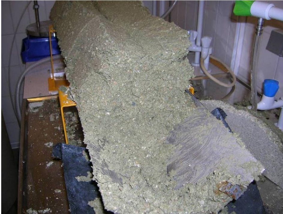
Figure A2-3. Block erosion test with 0.01 l/min and 1% salt in the water. A picture of a cross section shows that all bentonite was wetted. The result was the same for the test with 0.01 l/min and 3.5% salt in the water.
