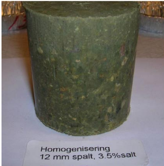
Figure 9-2. Photos taken after dismantling of the specimens. The former pellets filled slot can easily be seen but the width after homogenization is very difficult to determine.
