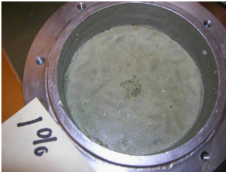
Figure 8-6. Picture of the specimen saturated with 1% salinity in the water. The photo is taken during dismantling. The drilled hole can still be seen. The hole is filled with gel with higher water content than the surroundings.
