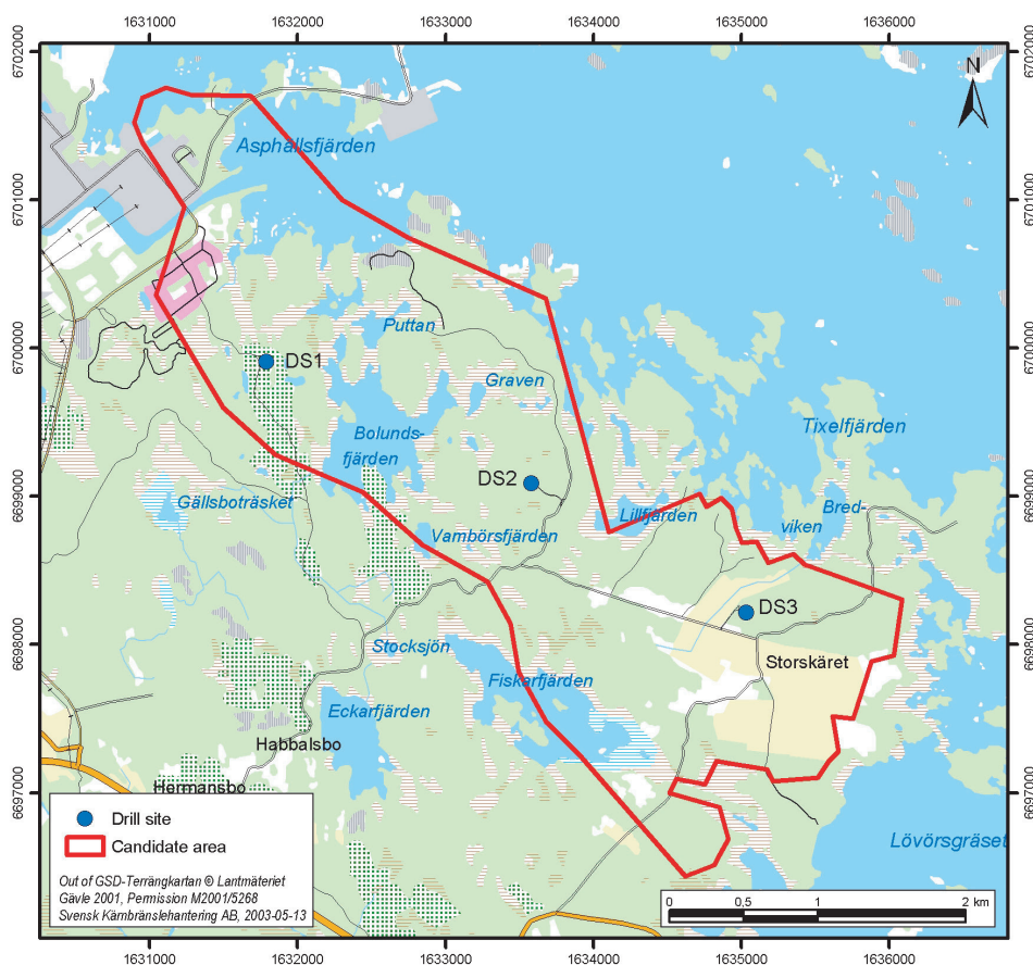
Figure 1-1. The investigation area at Forsmark including the candidate area selected for more detailed investigations. The drillsites for the earliest drilled deep cored boreholes are marked with blue dots. Borehole KFM01A is situated at drillsite DS1.
