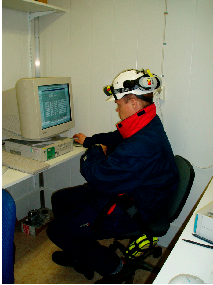
Figure 3-1. All pressure transducers are connected to the HMS system. In the G-tunnel there is a computer in the HMS system where logging frequencies easily can be changed.
