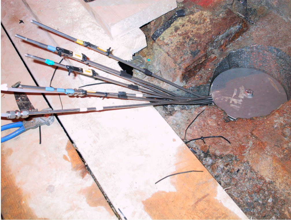
Figure 2-16 Tunnel-floor borehole covered with steel plate.
