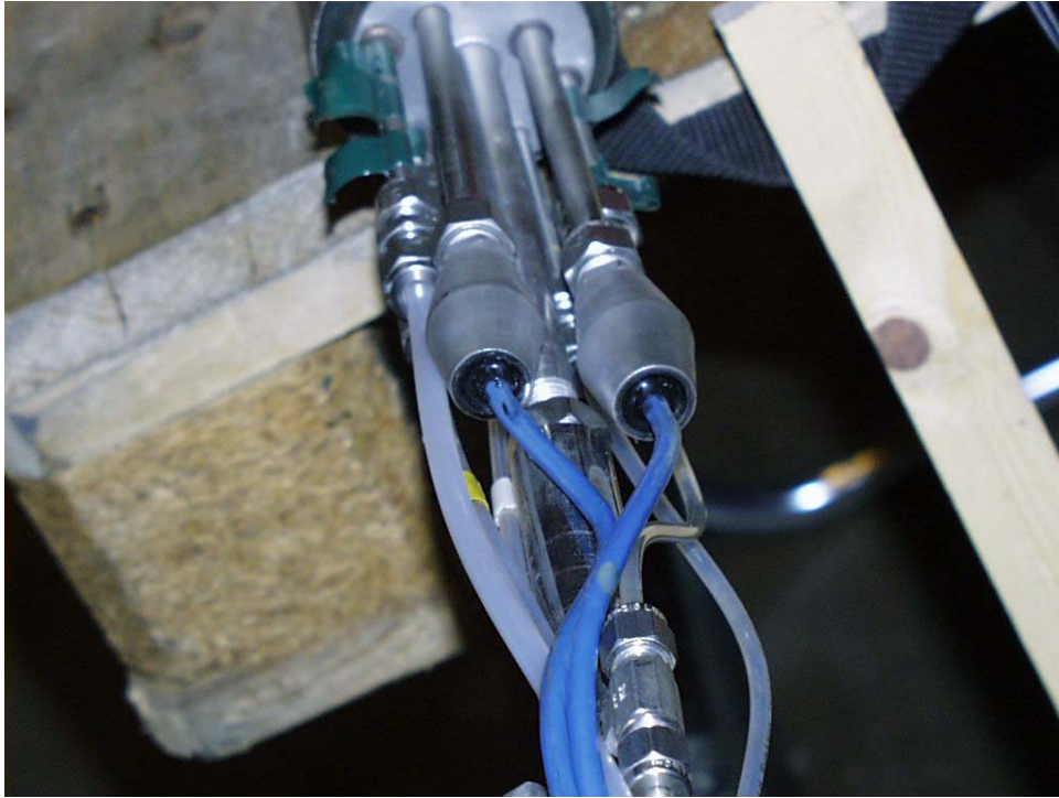
Figure 2-8 Air- and water-tight cable coupling from strain gauge. The sealing compound was PDM EMC-697 70 shore A.
