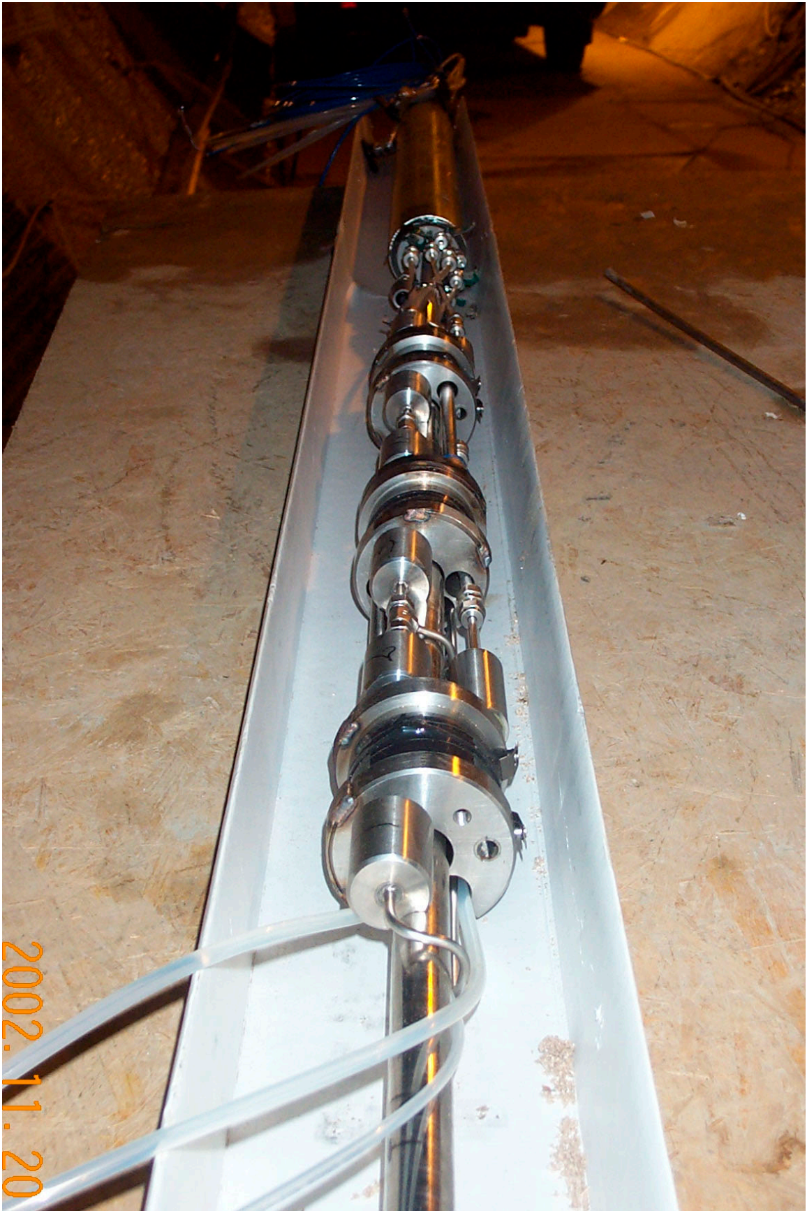
Figure 2-5 Hydro-mechanical equipment mounted on a centre rod between two packers.
