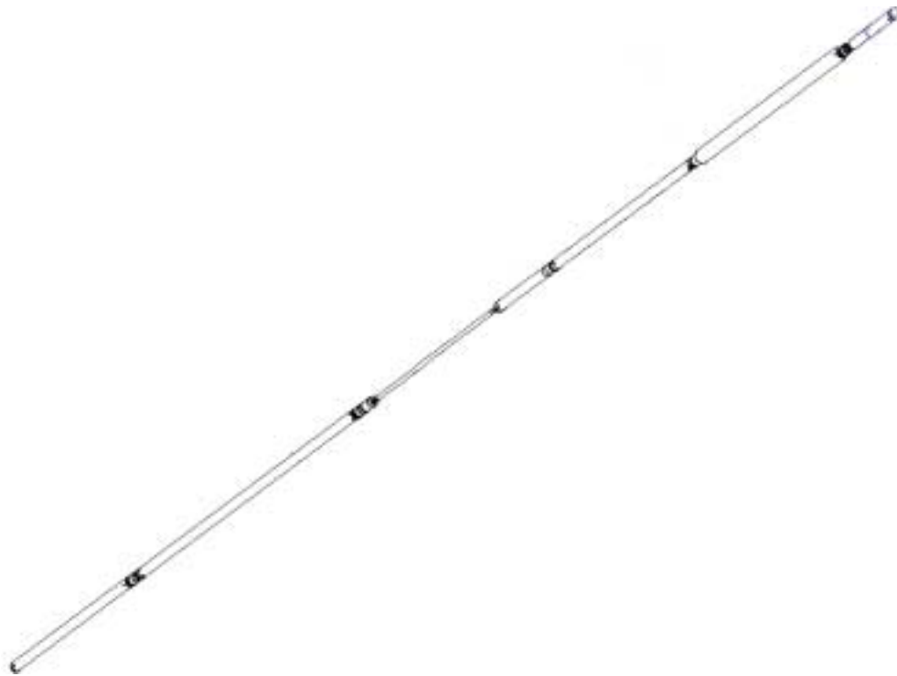
Figure 3-2. Example of a borehole antenna.
