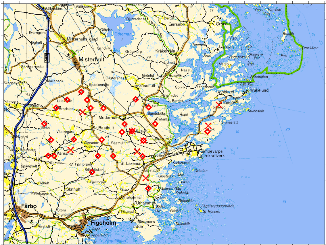
Figure 1-1. Locations of points for vertical electrical soundings (◊) and points for anisotropy measurements with X-configuration (x) according to the activity plan (AP PS 400-02-14).
