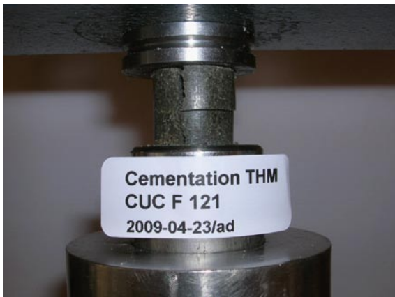
Figure 6-10b. Failure surface of sheared specimen of MX-80 and density of 2,030 kg/m 3 . The specimen was exposed to 200°C.
