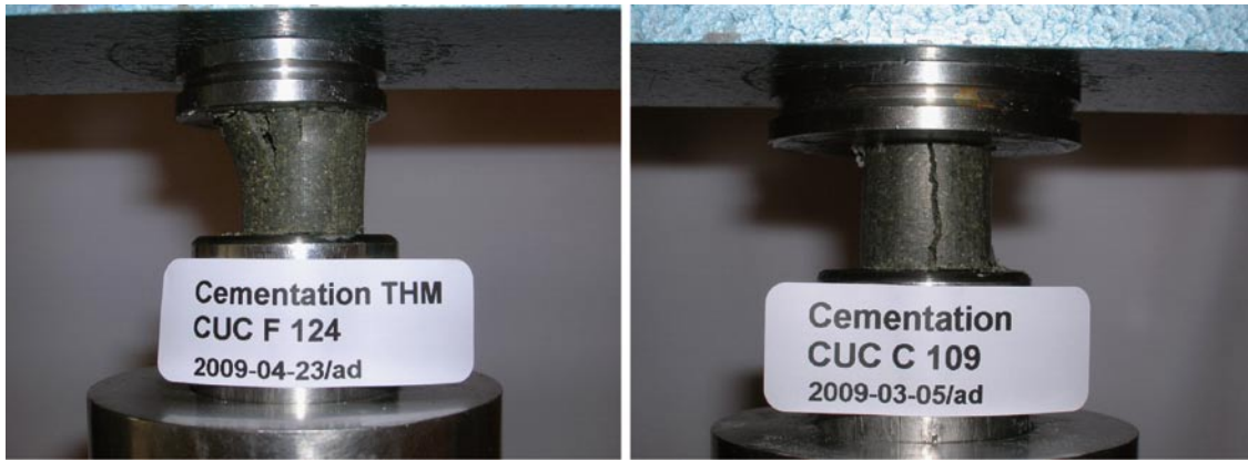
Figure 6-10a. Failure surfaces of sheared specimens of MX-80 and density of 2,070 kg/m 3 . The specimens were exposed to room temperature (left) and 150°C (right). (The photo to the right is also shown in Figure 6-2b).
