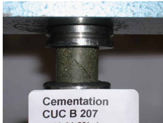
Figure 6-2a. Example of an ordinary shear failure and the corresponding failure surface.
