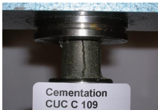
Figure 6-2b. Example of a brittle failure and the corresponding failure surface.
