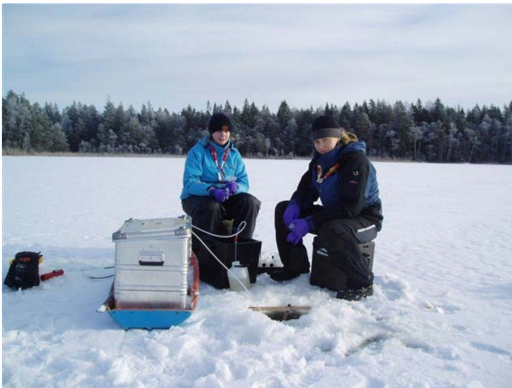
Figure 4-5. Sampling from the ice-covered lake, Eckarfjärden (PFM 000117). The peristaltic pump system is kept in an isolated trunk together with bottles of warm water to prevent freezing.
