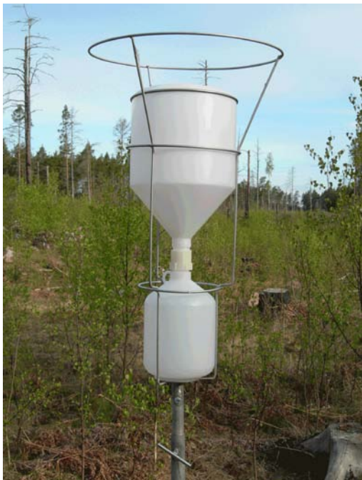
Figure 5-3. Precipitation sampler, summer setup. Two sampler setups were used simultaneously in order to increase the collected volume of the precipitation.
