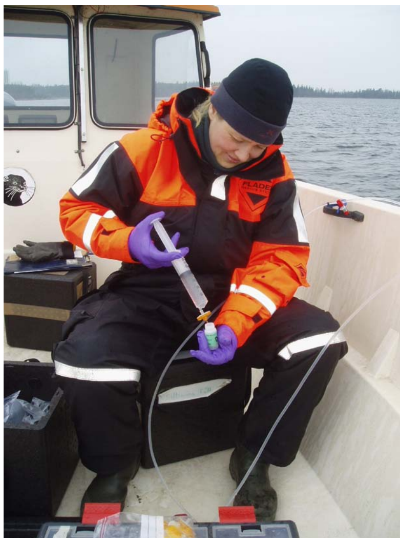
Figure 4-2. Filtering of sample portion in the field.
