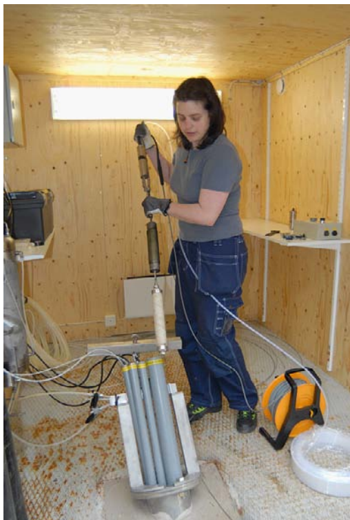
Figure 2-4. Lowering of equipment in the water stand-pipe in order to pump water from the borehole section. From the bottom; filter, small inflatable packer and pump.
