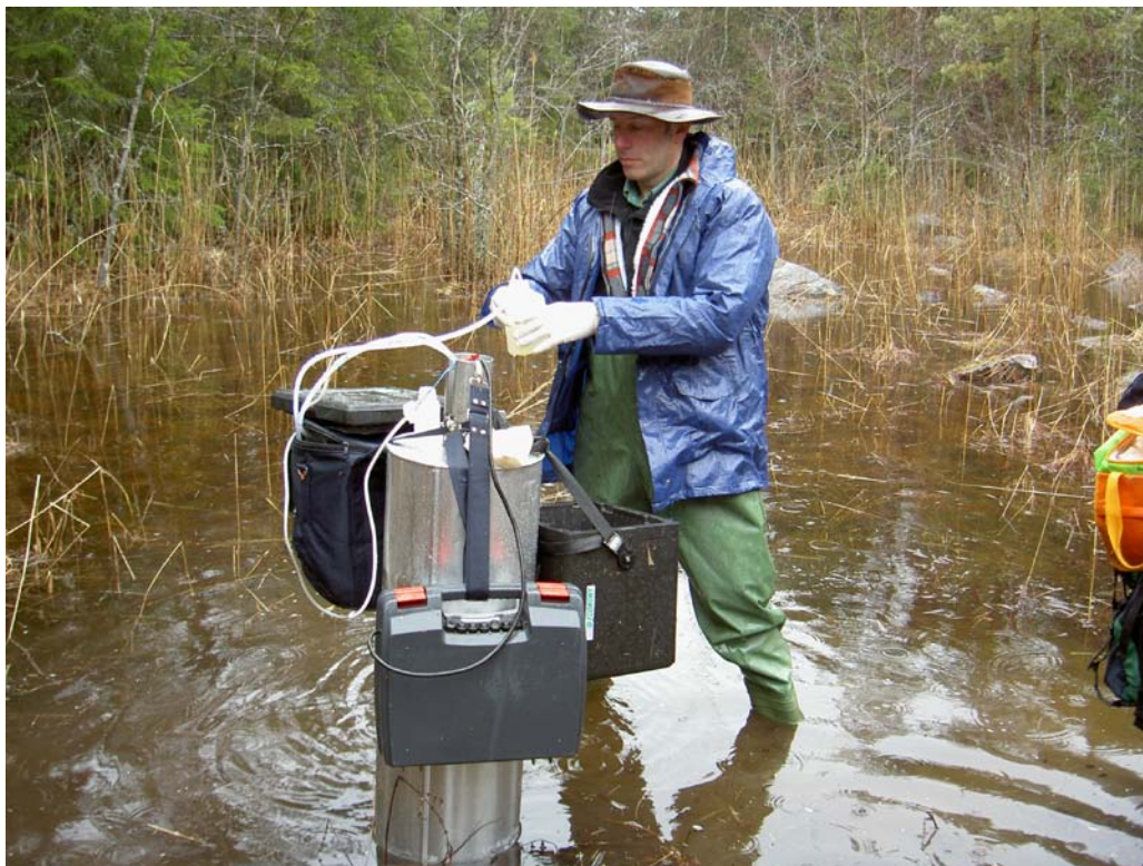
Figure 3-11. Sampling of near surface groundwater in pipe SFM0037.
