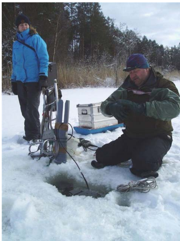
Figure 4-12. Sonde measurements on the ice-covered lake Norra bassängen (PFM000097).
