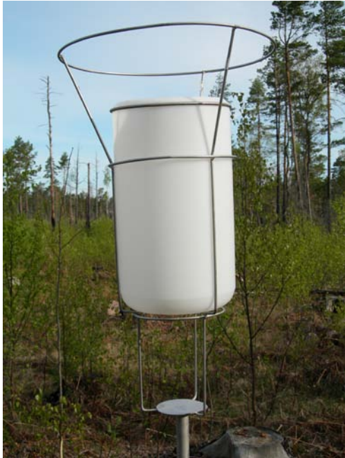
Figure 5-2. Precipitation sampler, winter setup. Two sampler setups were used simultaneously in order to increase the collected volume of the precipitation.
