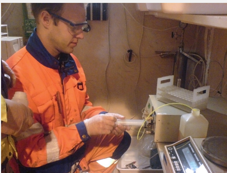
Injection of tracer in fracture.
