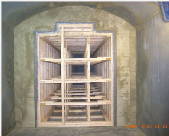
Test set-up for the deposition tunnel in half-scale.
