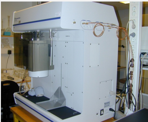
BET-analyser for determination of specific surface areas of geological materials.
