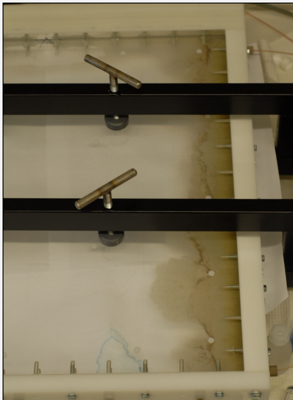
The expansion of bentonite into an artificial fracture.
