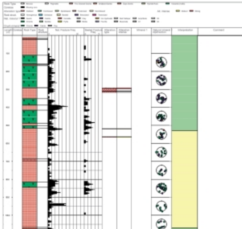
Figure 4-12. WellCad log of KLX01 showing lithology, fracturing and alteration along the borehole used in the Laxemar methodology test /Figure 3-8 in Andersson et al, 2002a/. The classified rock segments are shown as coloured boxes in the interpretation column.
