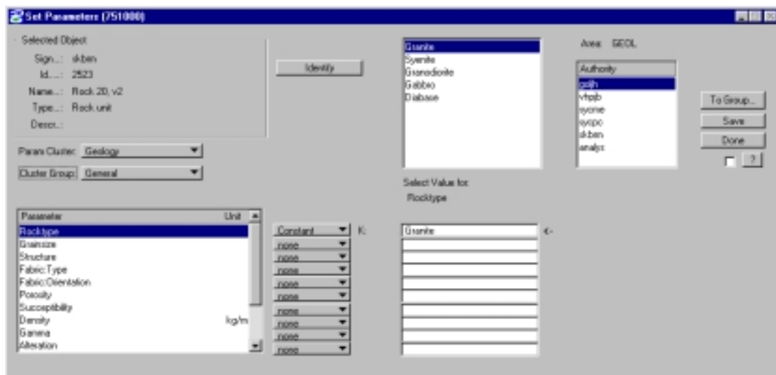
Figure A3-6. Dialogue window for the assignment of properties to objects in RVS, in this example for the object type “rock unit”. The dialogue contains sub-dialogues in order to be able to describe, in this case, rocks in detail, as well as dialogues for stochastically defining fracture patterns.
