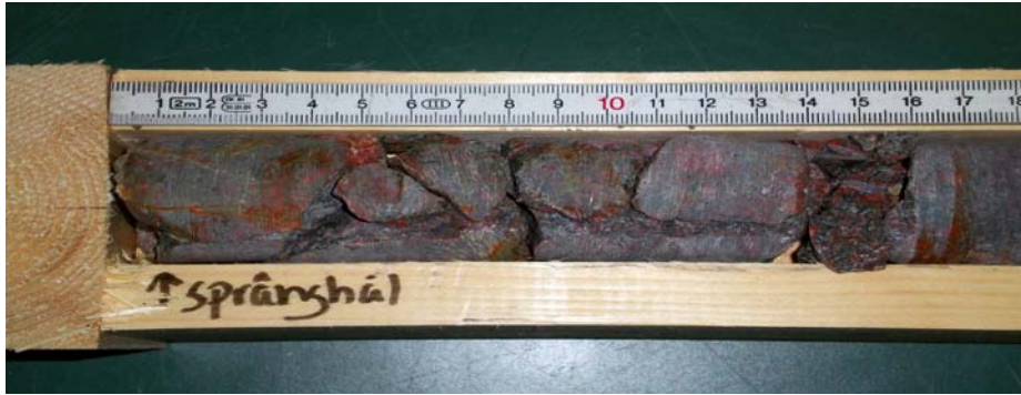
Figure 5-4. A close-up of the damaged part closest to the charge borehole, the first 16 cm.
