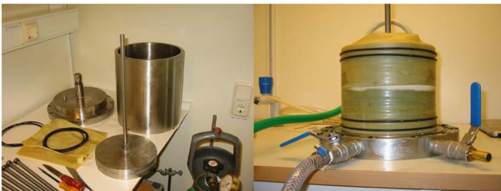
Figure 4-2. To the left is the triaxial cell permeameter and its different parts and to the right is a sample placed on the bottom plate. The sample is surrounded by double rubber membranes and a total of four o-rings.
