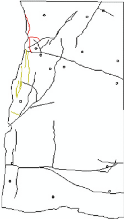
Figure A5-1. Digitized slab surface with fractures, 36B-05. Natural fractures are black.
