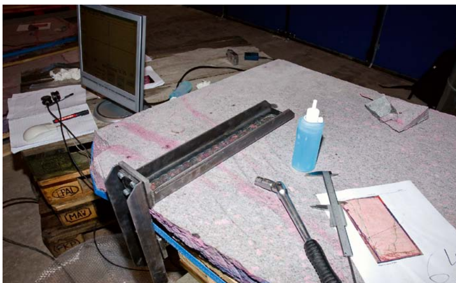
Figure 7-2. The steel frame placed on the slab so that the sensor and the receiver of the compression wave are fixed, both in relation to the scan line and to each other.
