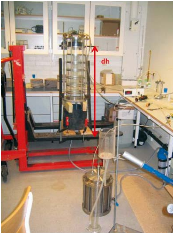
Figure 4-1. Equipment used for testing rock samples from the Q- and S-tunnel. The red vertical line represents the fall in pressure, dh , through the sample.
