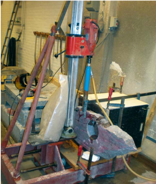
Figure 5-1. Drilling of smaller samples from slab BC.
