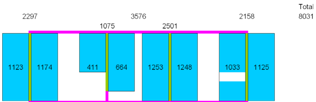
Figure 3-15. Figure shows the number of deposition hole positions in total, and by sub area. Sub division in accordance with Figure 3-11.
