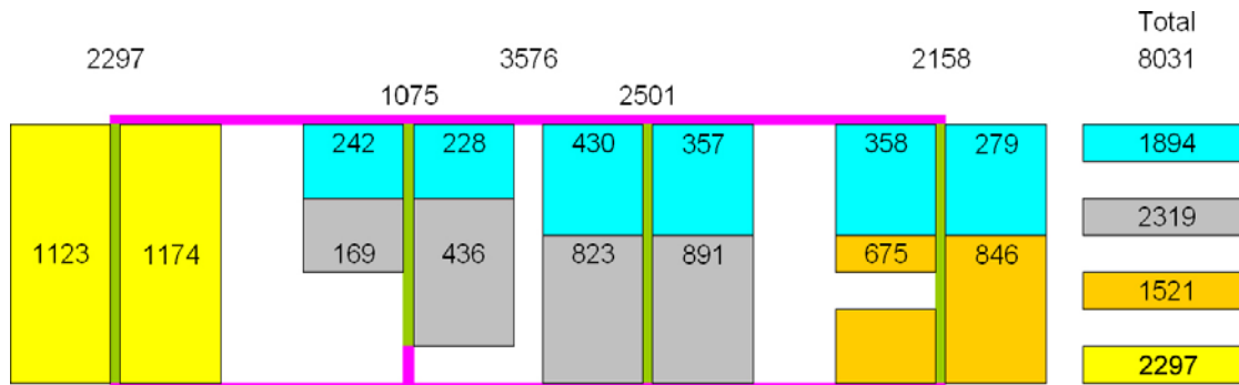
Figure 3-17. Figure shows the number of deposition hole positions by fracture domain. Sub division in accordance with Figure 3-13.
