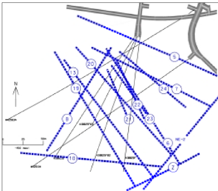
Figure EX-1. March 2000 hydrostructural model. Plan view of interpreted deterministic structures at Z=-450 masl.
