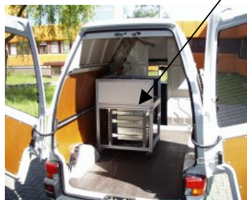
Figure 2-7. Equipment for Laser-Induced Breakdown-Detection (LIBD) of colloids (upper picture). The equipment is installed in a van in order to allow mobility and on-line measurements (lower picture).
