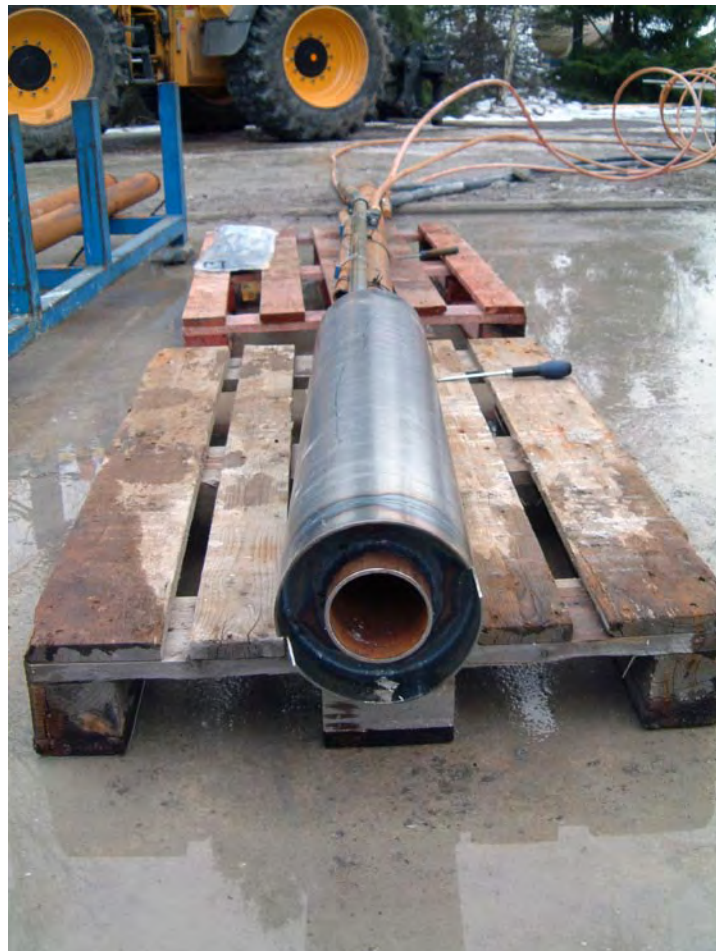
Figure 5-5. The air-lift pumping system.
