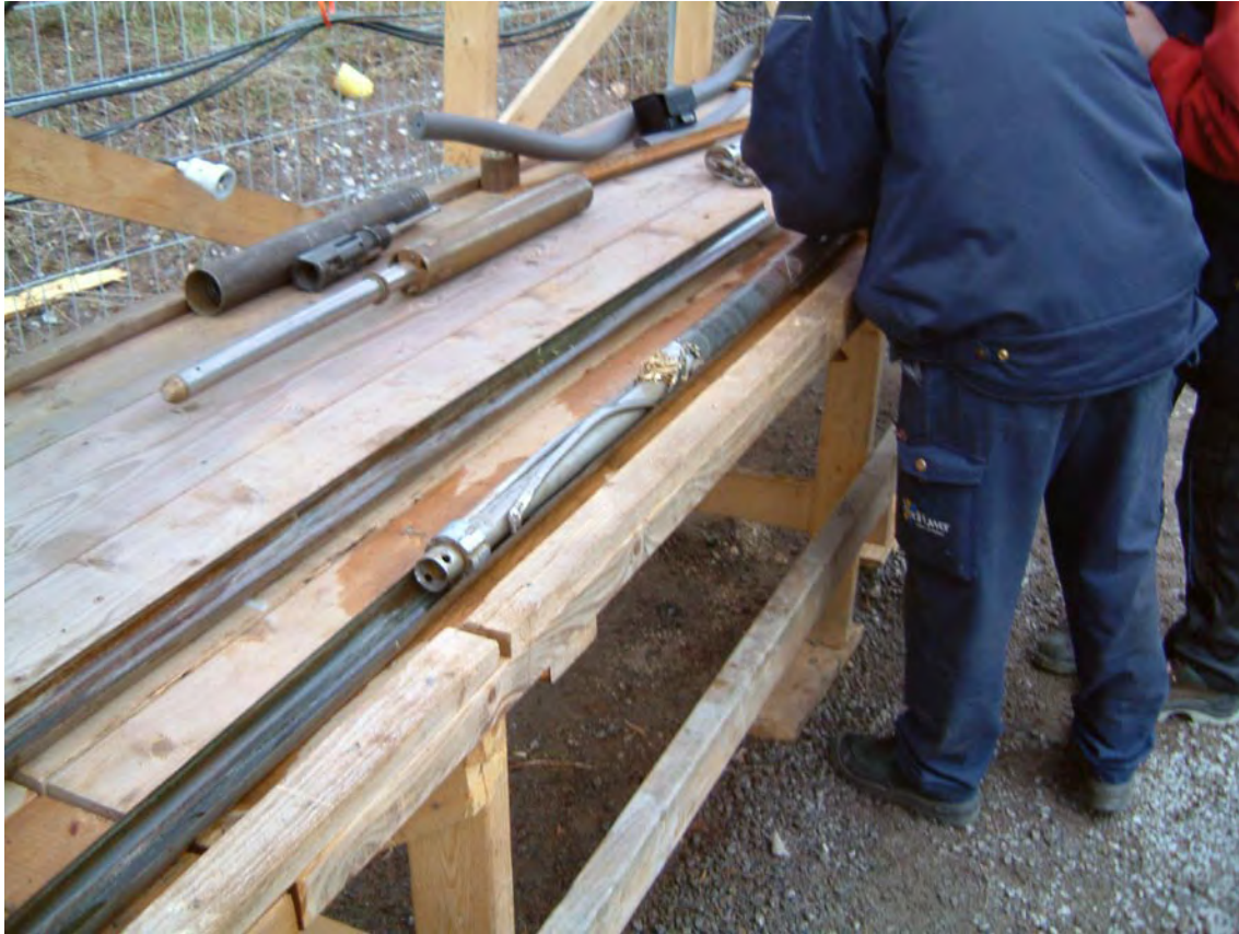
Figure 5-9. The Borre overcoring equipment.
