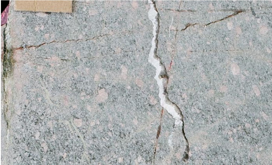
Figure 6-13. Block section with fractures with and without mineral fillings.
