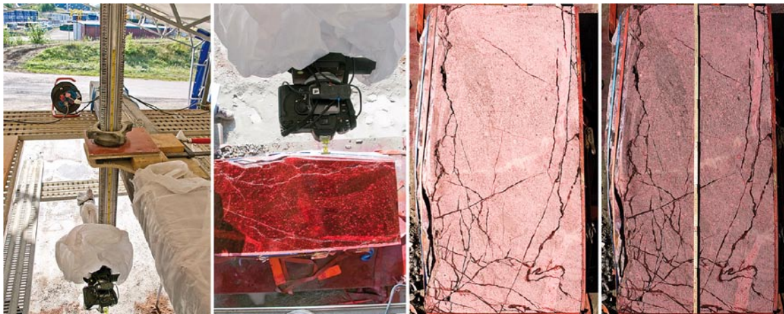
Figure 4-11. Photographing. From left to right: The camera, image from above showing camera and dyed surface, the investigated surface photographed without and with a reference scale.
