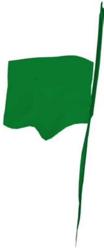
Figure 7-16. The fracture on the left is only detected on one side of the intersecting fracture, resulting in a gap between the fractures.
