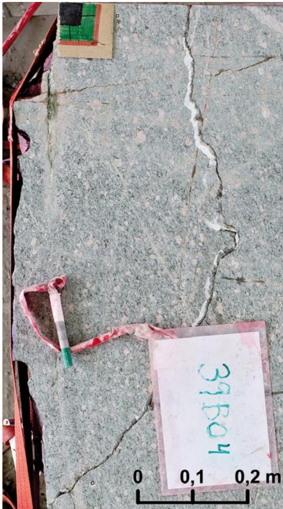
Figure 2-8. An open, 2 cm thick fracture filled with calcite in block 39. Note half-casts on left side of slab.
