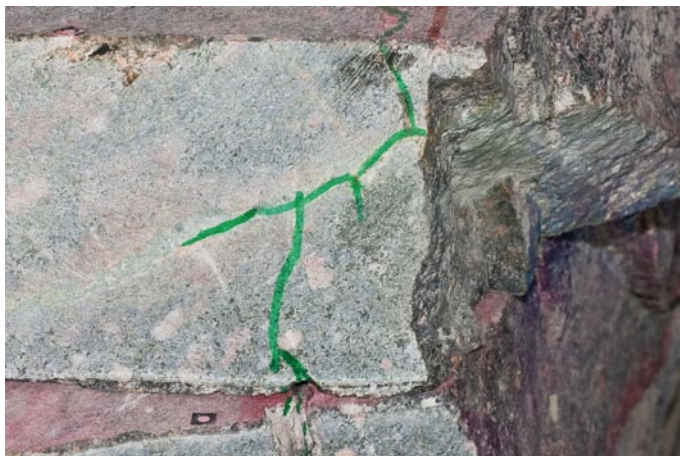
Figure 6-18. Detail of case 1. A blast fracture which comes from above meets an intersecting fracture, jumps to the side and continues.
