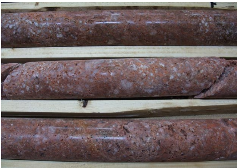
Figure 5-2. Quartz dissolution in the borehole interval 440.4–478.4 m.
