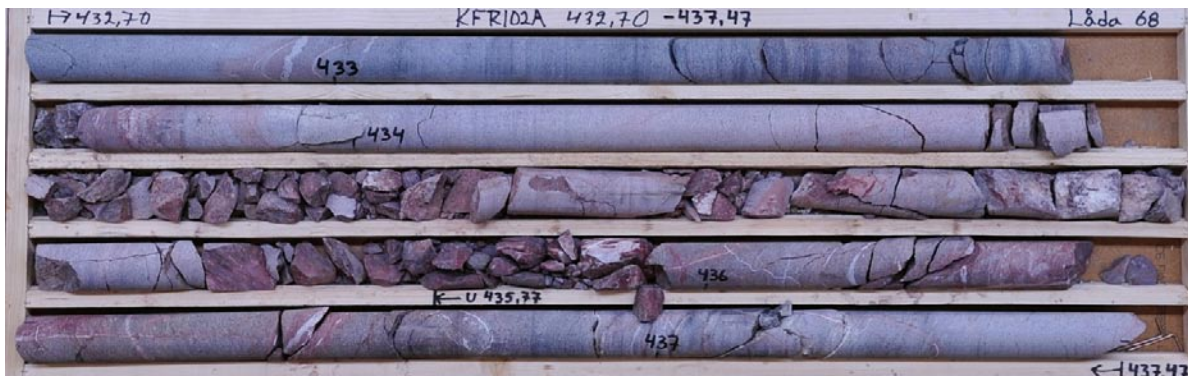
Figure 5-4. The major crush in KFR102A at 434.65–435.90 m.
