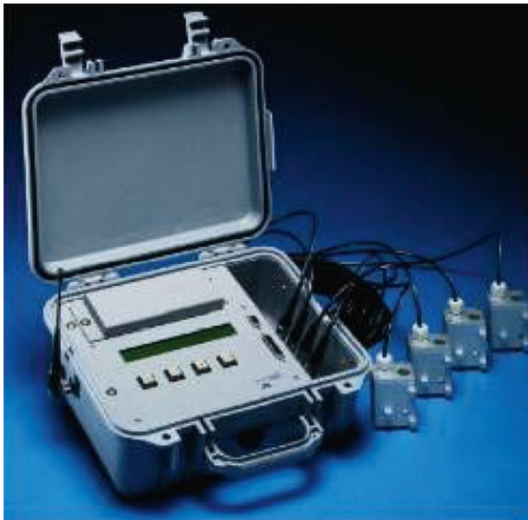
Figure 3-1. Recording unit Ava95 and geophones for vibration measurement.
