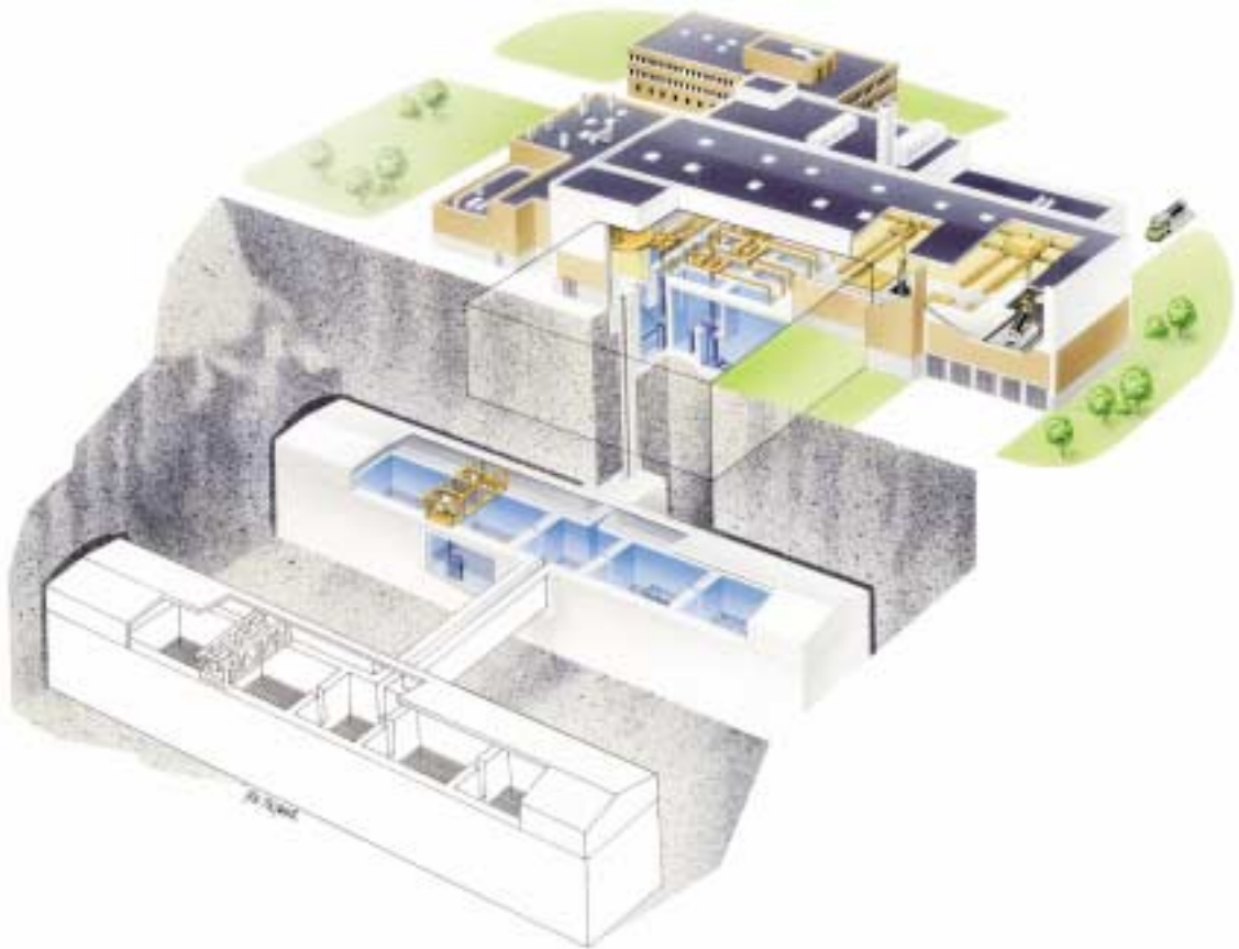
Figure 1-4. The central interim storage facility for spent nuclear fuel (CLAB 1 and 2). From /SKB, 2000b/.
