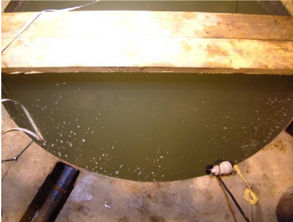
Figure 2-8. Gas bubbles on the water surface in the Lasgit hole.
