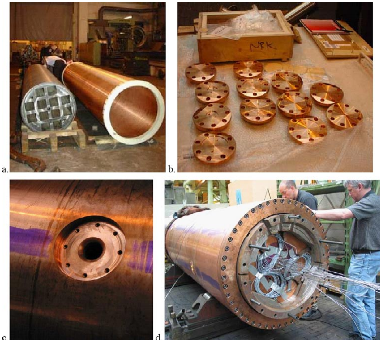
Figure 3-4. The canister as used in the Lasgit test. The canister comprises a standard KBS-3 canister, made up of a copper canister and cast iron insert (a). Twelve filters (b) are placed at three levels along the length of the canister in recesses (c). The complete Lasgit canister is shown in (d) with the filters in place and the associated pipework coming through the canister lid.
