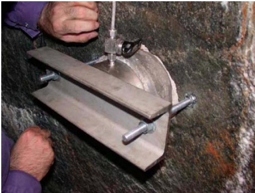
Figure 2-10. The surface packer system of BGR shown in situ ready for the start of a test.
