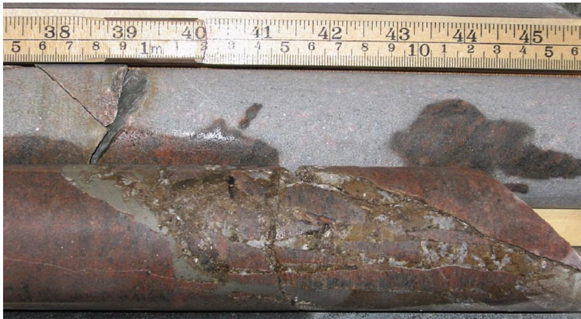
Figure 5-5. Sealed breccia in KFR102B at 69.0 m, with calcite, prehnite and probable iron hydroxide.
