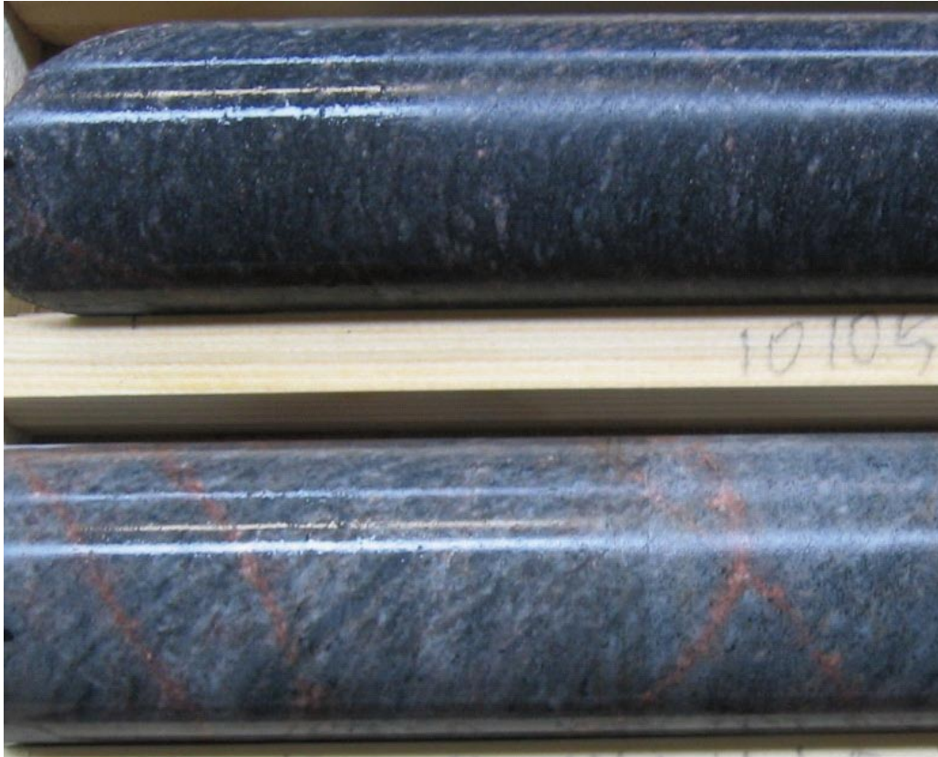
Figure 5-11. Example of high strain in metagranite-granodiorite, KFR103, ca 63 m borehole length.
