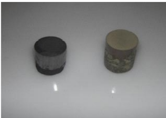
Figure 3-1. UN (left) and ZrN (right) pellets manufactured in the fuel fabrication laboratory of KTH.
