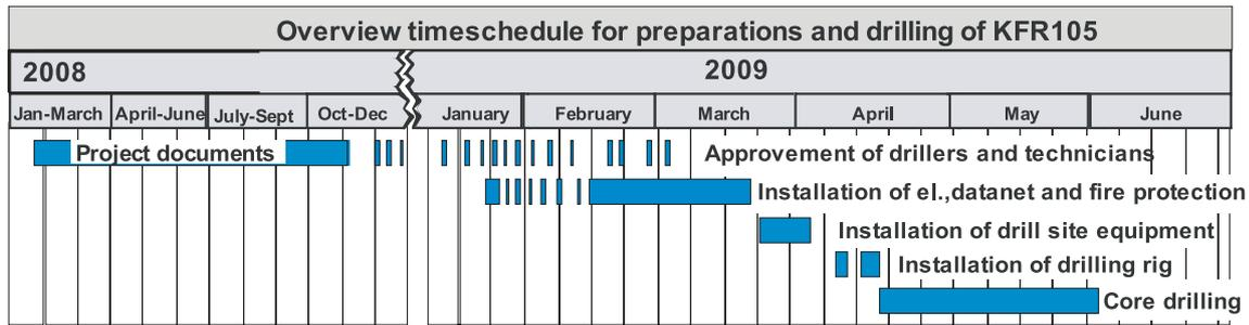
**Figur 5-1.** Overview time schedule of the preparations and drilling performance of borehole KFR105. More than a year before commencement of drilling, the initial work started in order to get approval for drilling performance during mid April to early June 2009.
