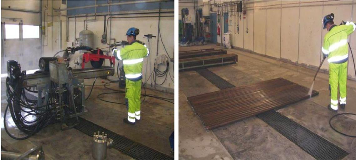
**Figure 5-11A.** To the left cleaning with hot water of the drilling machine and, to the right, of drill pipes before transportation to the underground drill site.
