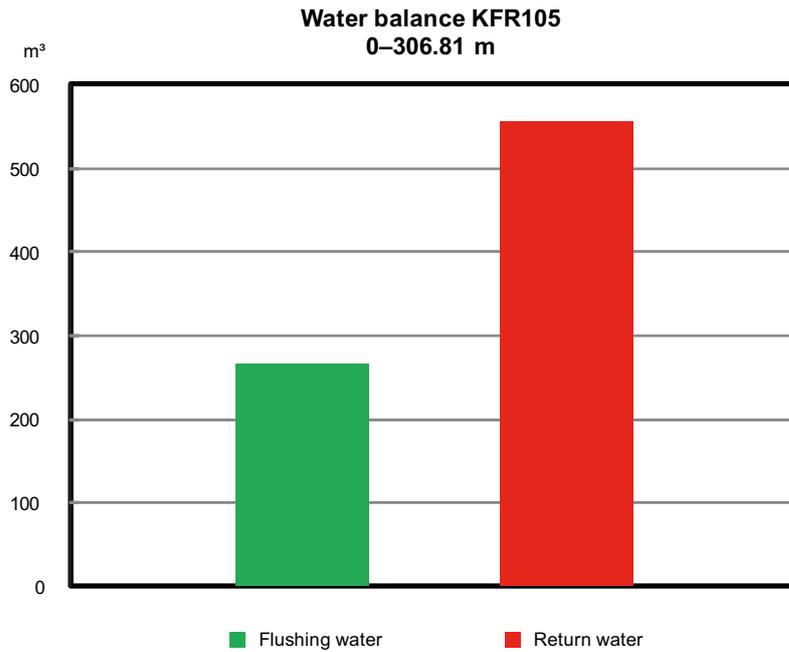
**Figure 5-15.** Total amounts of flushing water and return water during drilling of borehole KFR105. The total volume of flushing water used during core drilling was amounted to 265 m<sup>3</sup>. During the same period, the total volume of return water was 554 m<sup>3</sup>. The return water/flushing water balance is then as high as 2.09, due to constant outflow from a borehole drilled from underground and below the groundwater table.
