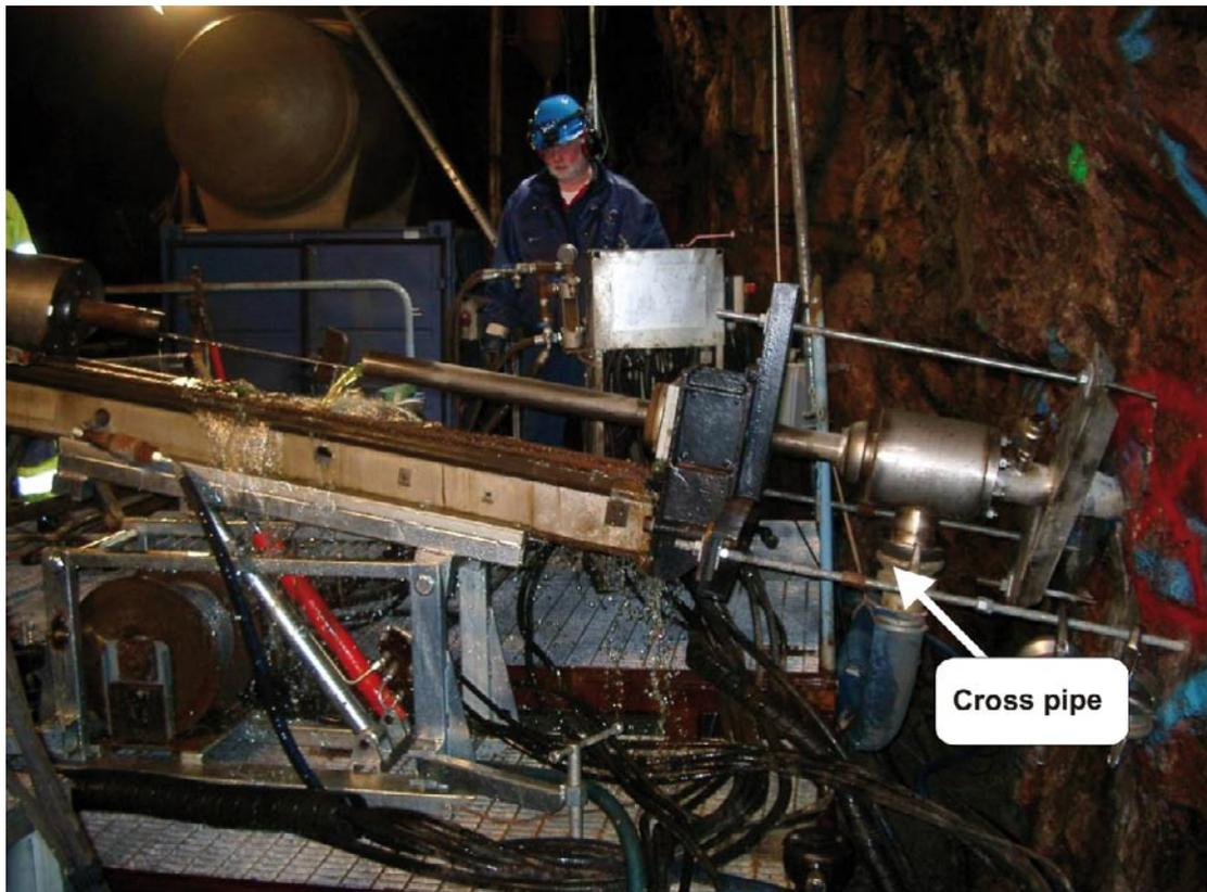
**Figure 5-16.** The figure demonstrates the driller pulling the inner tube containing 3 m drill core. During this phase of the drilling sequence the return water is evacuated from the drill rods and collected by the water-tight drill platform, from which it is pumped away for flow measurements and sedimentation of drill cuttings. During the drilling phase, the return water is forced through the cross pipe and down to the platform.
