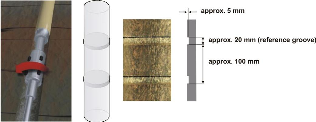
Figure 3-4. Layout and design of reference grooves.
