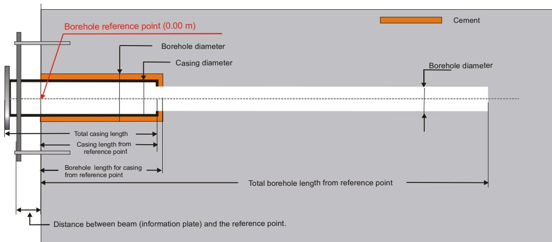
**Figure 5-6.** Schematic drawing of a cored borehole of traditional type drilled from underground. The figure shows definitions of the most important data, as reference points, lengths and dimensions used for the technical description of the borehole in this report.
