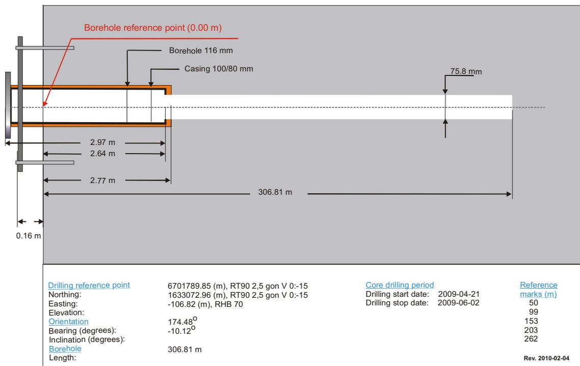
**Figure 5-10. Technical data of borehole KFR105.**
