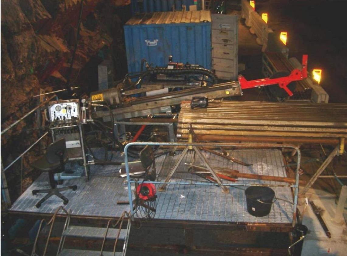
*Figure 4-2. The figure shows the steel platform in use underground.*
