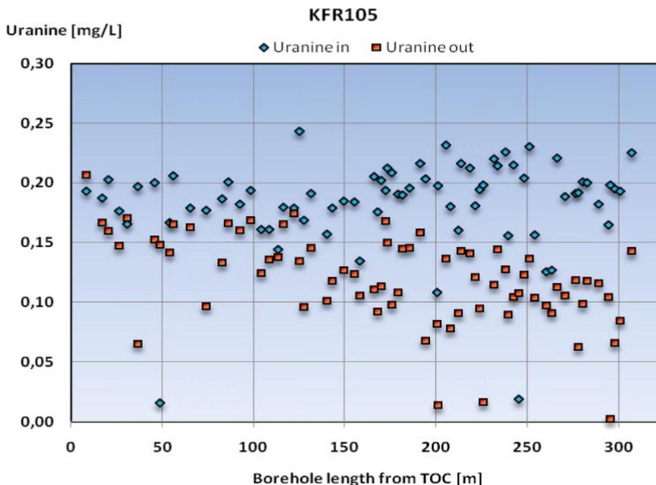
**Figure 5-17.** Uranine contents in the flushing water consumed and the return water recovered versus drilling length during drilling of borehole KFR105. Automatic dosing equipment, controlled by a flow meter, accomplished the labelling with Uranine.
