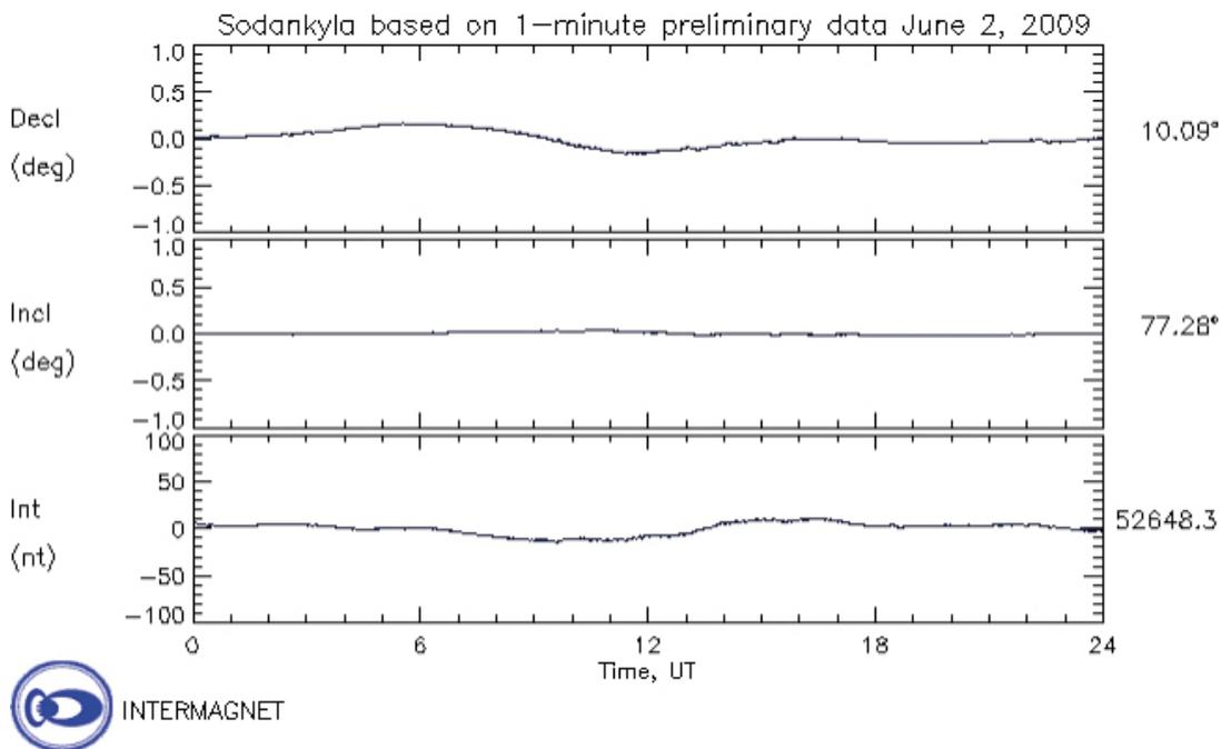
**Figure 5-24.** Magnetic field variations during Flexit surveys performed on June 2<sup>nd</sup> 2009 in KFR105.
