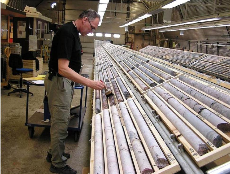
**Figure 5-21.** The core boxes were transported every morning during the drilling period to the core store-room, the so called Llentab facility. A simplified geological core mapping was performed, and afterwards all core boxes were photographed. A detailed core mapping together with analysis of BIPS-images, so called Boremap mapping, was conducted after completion of drilling.
