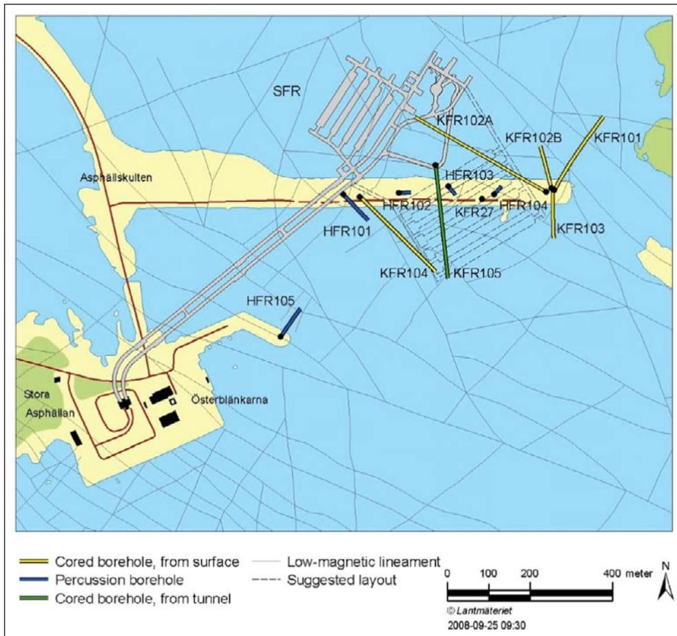
**Figure 1-2.** Overview of the SFR site investigation area with planned investigation boreholes. Also the suggested layout of the extended SFR facilities as well as low-magnetic lineaments in the area are displayed.
