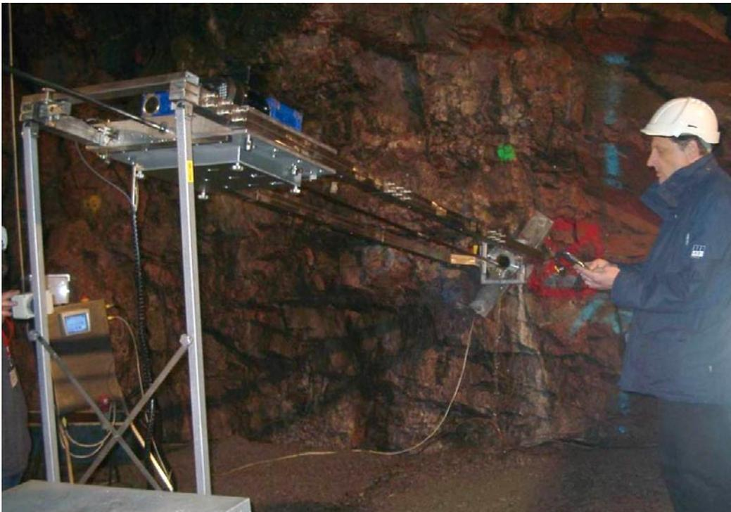
**Figure 5-22.** The figure shows the new system for insertion of different logging tools with rods to be used in non-vertical boreholes.
