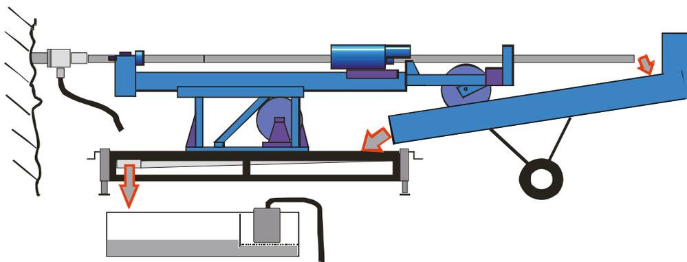
**Figur 3-3.** As an underground drilled borehole is in a state of constant hydrostatic overpressure, most of the return water discharges at TOC. Return water can also flow through the open drill rods, but was when drilling KFR105 funnelled to the drill platform which had an outlet to a collecting box for further pumping.
