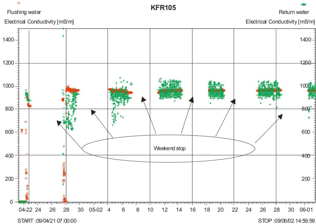
**Figure 5-18.** Electrical conductivity of flushing water (from “Nedre bassängen”) and return water from KFR105.
