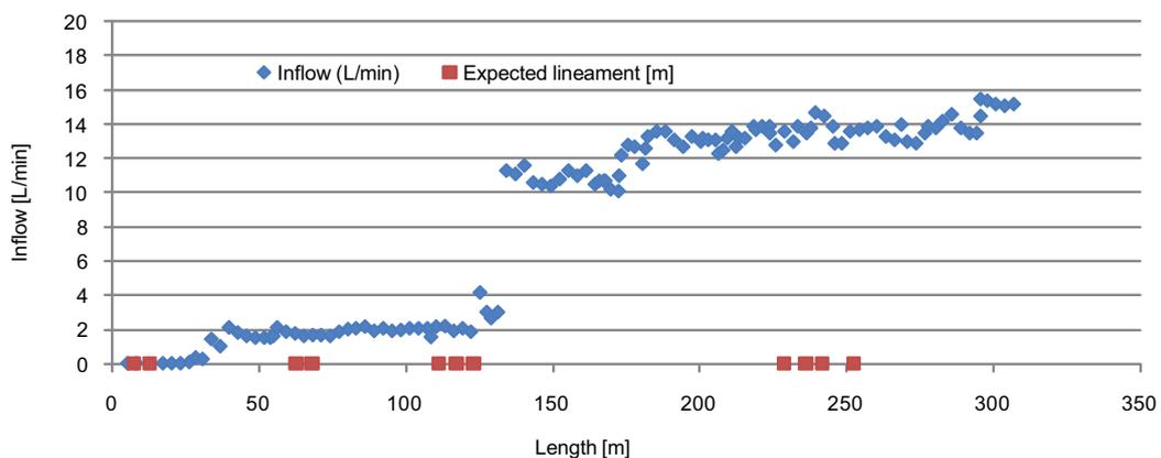
**Figure 5-19.** Accumulated inflow to the borehole measured after finished drilling but with the drill string still left in the borehole. At c. 135 m (May 11<sup>th</sup>) an increased inflow of water to the borehole is observed.
