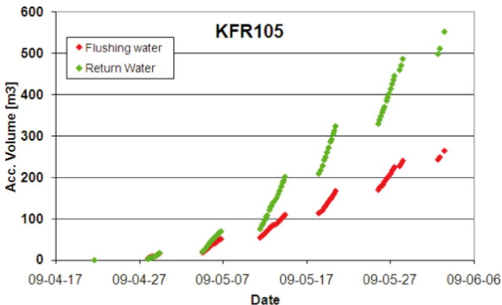
**Figure 5-14.** Accumulated volumes of flushing water (red) and return water (green) versus time during core drilling of borehole KFR105.
