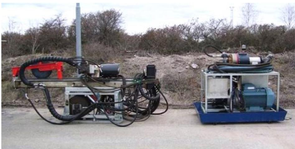
**Figure 3-1.** The Sandvik DE130 machine used for drilling borehole KFR105.
