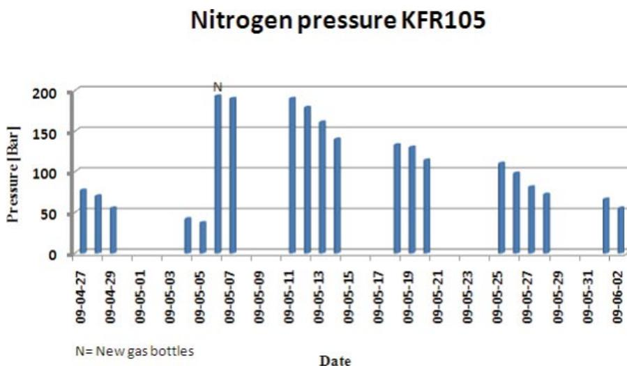
**Figure 5-20.** Nitrogen contents (measured as pressure) in the bottles for nitrogen bubbling of flushing water in KFR105A. “N” above bars equals to change of nitrogen bottle batteries.
