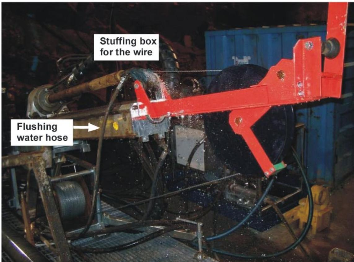
*Figure 5-7. The figure shows time consuming in-pumping of the overshot and wire for retrieval the drill core filled inner tube.*
