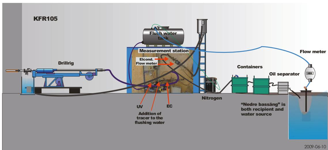
**Figure 3-2.** Schematic illustration of the flushing/return water system when drilling KFR105. The measurement station included logger units and an UV-radiation unit, and an additional flow meter measured the total incoming water. “Nedre bassängen” is located at the lowest elevation in the SFR-facility and served as the flushing water source and also as the recipient for the return water during core drilling of KFR105.
