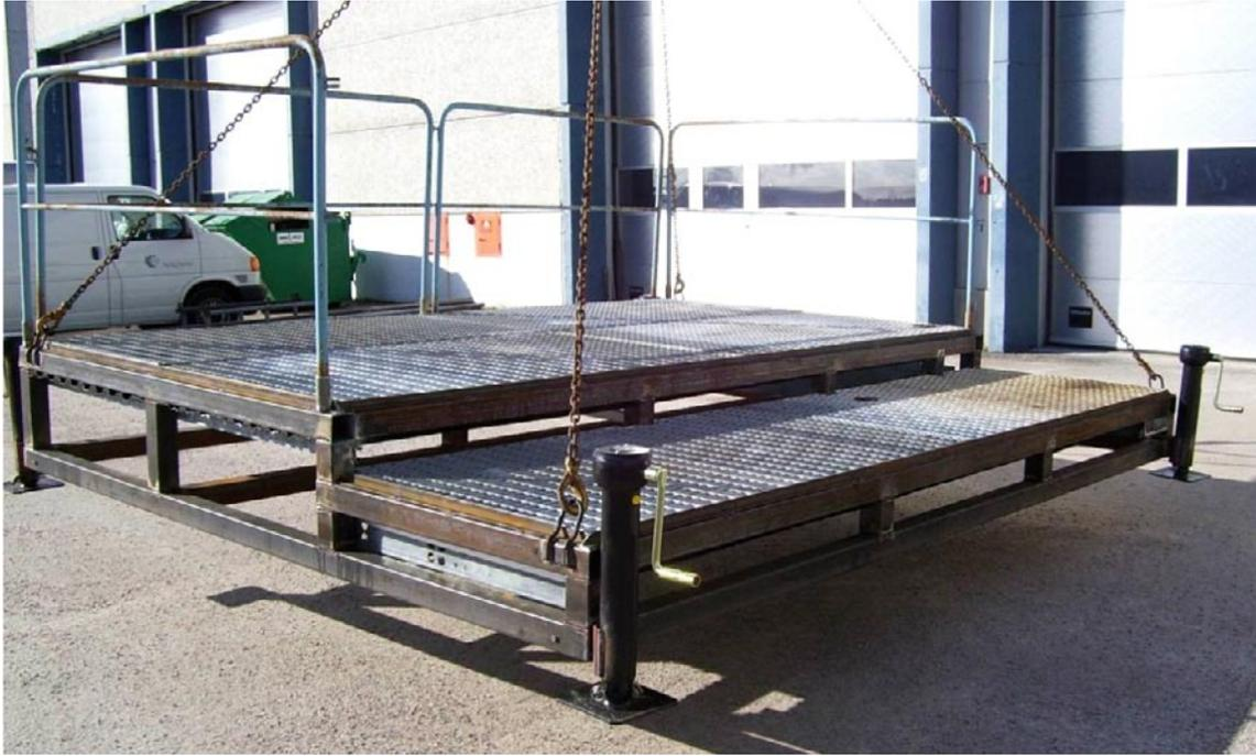
*Figure 4-1. The figure shows the empty steel platform on ground, with levelling jacks on each corner.*
