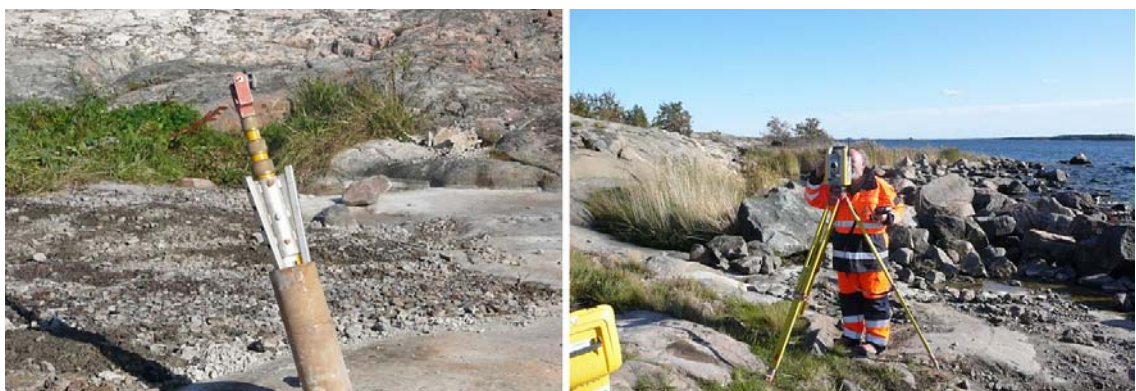
Figure 5-19. Surveying of the borehole collar coordinates and borehole orientation is crucial for calculating the borehole deviation. Lining up a borehole collar demands careful handling of the instrument as well as of the accessories. To get accurate data, the reflector must be centralized into the borehole casing. The reflector is mounted on a telescopic tube that has to be stiff when it is pulled out in order to measure the borehole orientation.
