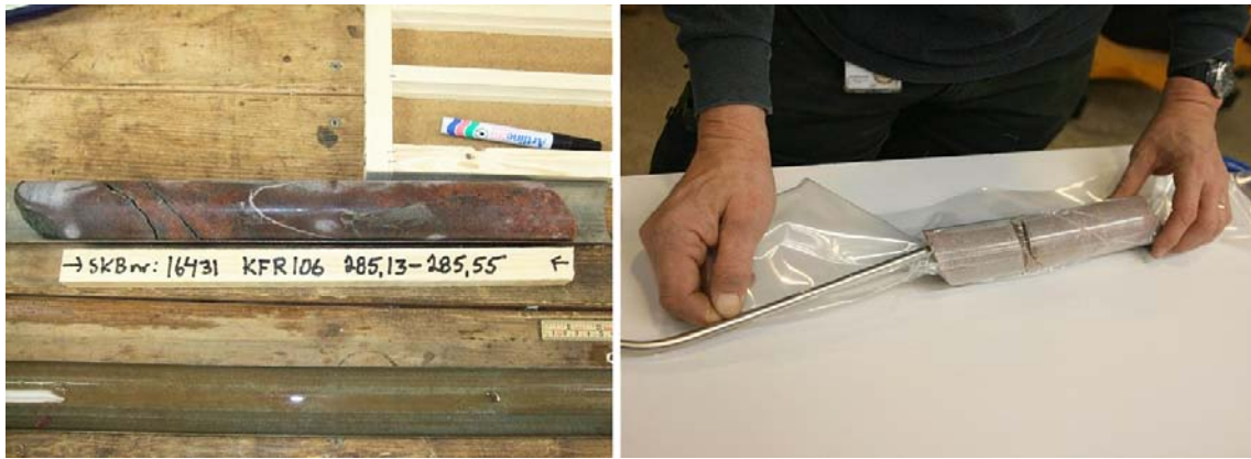
Figure 5-18. Every potential water-bearing fracture in KFR106 was sampled. The core was measured for exact borehole length and photographed. To avoid mineral oxidation, the sample was placed within three layers of plastic bags. Each layer was nitrogen filled, vacuum pumped and sealed and finally stored in a freezer at the Llentab facility.
