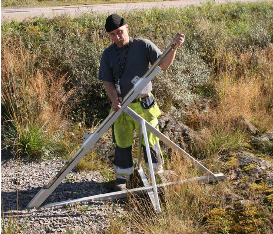
Figure 3-4. The Flexit Smart Tool is prepared for readings in the Forsmark reference stand.
