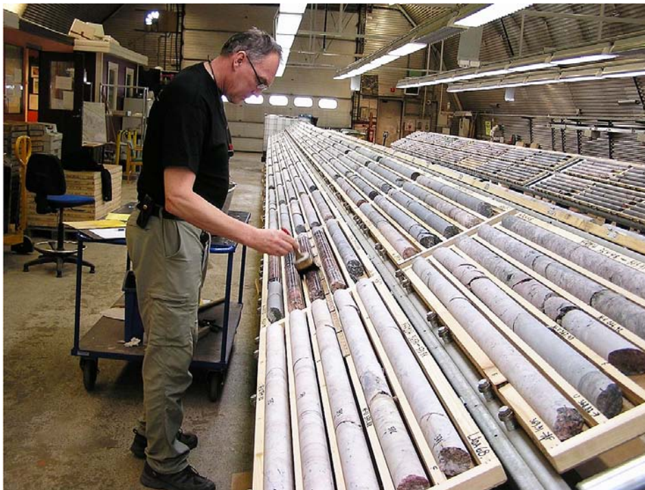
Figure 5-17. The core boxes were transported every morning during the drilling period to the core store-room, the so called Llentab facility. A simplified geological core mapping was performed, and afterwards all core boxes were photographed. A detailed core mapping together with analysis of BIPS-images, so called Boremap mapping, will be carried out after completion of drilling.
