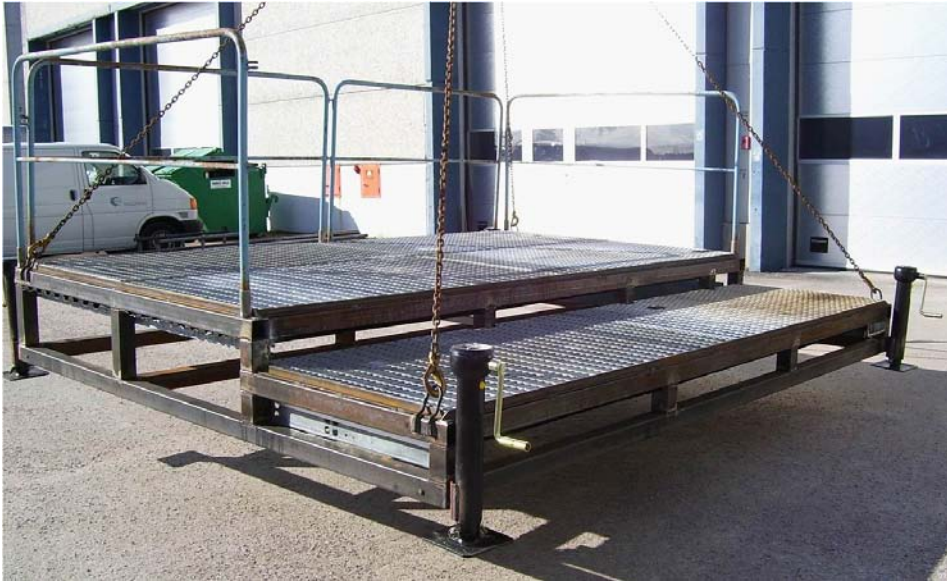
Figure 5-5. The platform, originally constructed for underground use, was modified to be used for core drilling on the islet.
