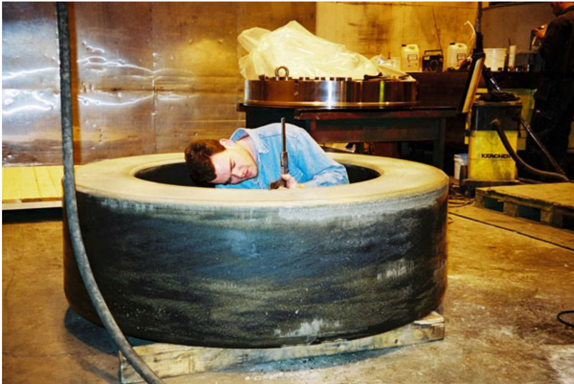
Figure 4-7. The height of the bentonite block is measured.
