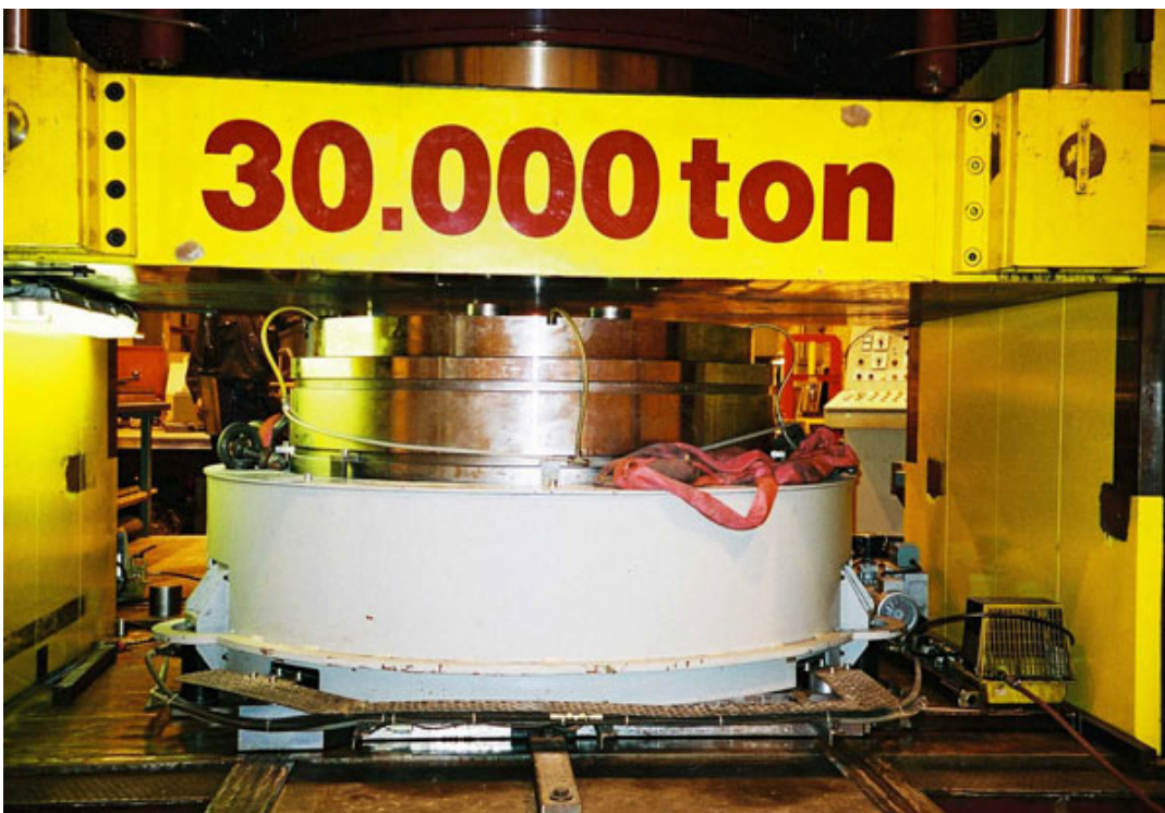
Figure 4-4. The form with the first piston placed in the press.
