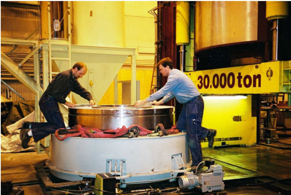
Figure 4-3. Bentonite filled into the form.
