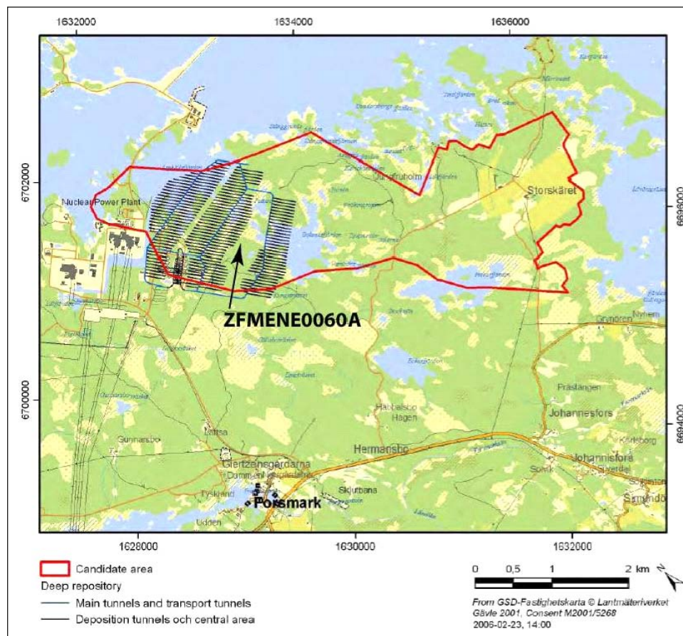
Figure 2-1. Geographical setting of the Forsmark site and location of the deep repository from design stage D1 (based on Figure 5-2 in SKB R-06-34).
