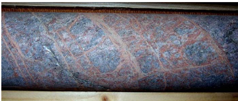
Figure 2-6. Example of a sealed fracture network from borehole KFM06A. This term "sealed fracture network" is used to describe a high frequency of sealed fractures that is commonly encountered in deformation zones at Forsmark. The core diameter is 51 mm.
