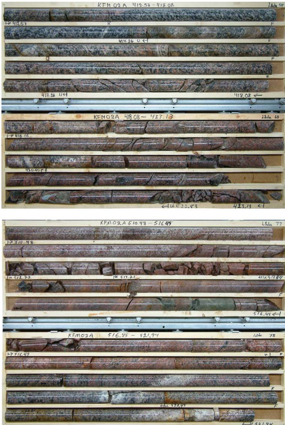
Figure 2-11. Character of deformation zones in the gently dipping set. a) Open and sealed fractures, crush zone and alteration defined by hematite dissemination and red staining along the borehole interval c. 413 to 423 m in KFM02A. This interval marks the transition from the bedrock above zone A2, predominantly in the upper drill core box, into the bedrock affected by zone A2 predominantly in the lower drill core box. b) Similar features along the borehole interval c. 510 to 522 m in KFM02A. This view shows the transition from the bedrock inside zone F1, predominantly in the upper drill core box and approximately half of the lower drill core box, into the bedrock beneath zone F1, in the remainder of the lower drill core box.
