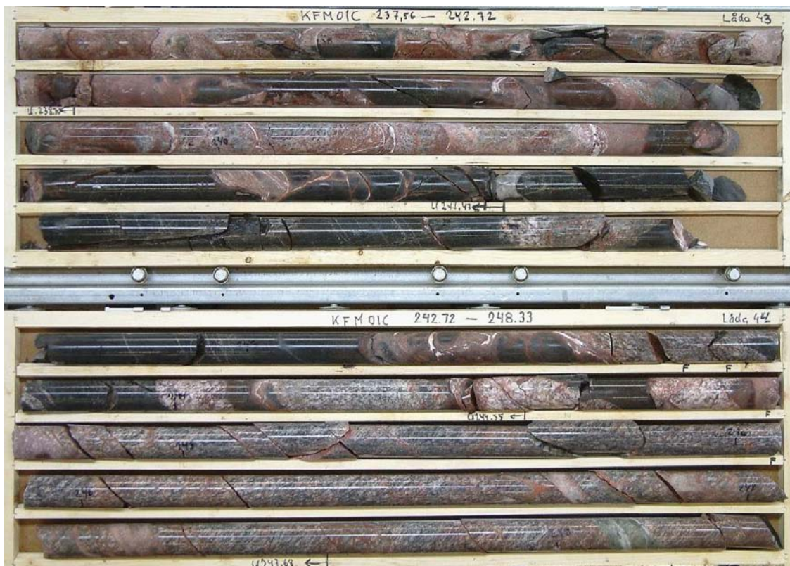
Figure 2-10. Character of deformation zones in the vertical or steeply dipping, ENE to NNE set. The photo shows the core from deformation zone ENE0060A in the interval c. 237–248 m in KFM01C showing the dominance of sealed fractures and sealed fracture networks. A fault core interval has been recognised at c. 238 m. The darker portion of the core is amphibolite. Modified from Figure 5-31 in /SKB 2008/.
