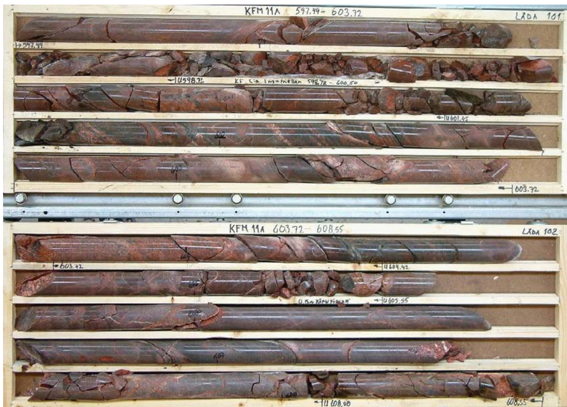
Figure 2-9. Character of regional deformation zones in the vertical or steeply dipping, WNW to NW set. Crush zones, laumontite-sealed cataclasites and networks, and wall-rock alteration defined by dissemination of hematite and red staining, along part of a fault core interval in the Singö deformation zone (WNW0001) in borehole KFM11A (borehole interval c. 597 to 608 m). Modified from Figure 5-33 in /SKB 2008/.
