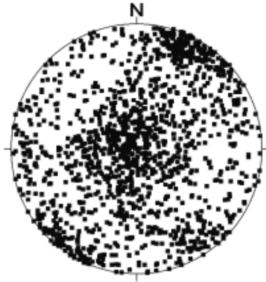
Figure 3-3. Lower hemisphere projection of poles to fracture planes in the 36 bore- and exploratory holes.
