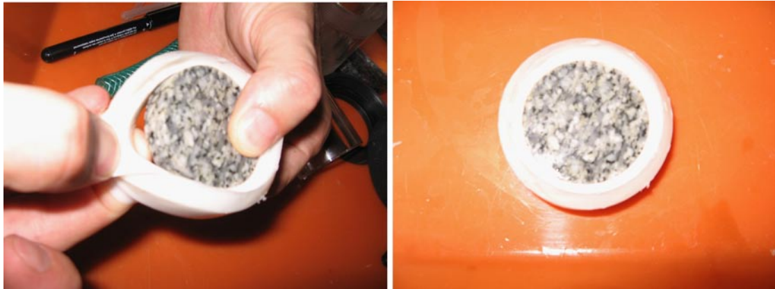
Figure 4-2. a) Fitting the sealing ring on the sample. b) The sample fitted by the sealing ring.
