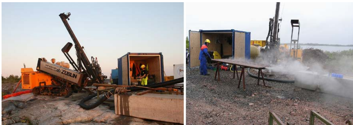
Figure 3-1. The Nemek 407 RE percussion drilling machine employed for drilling the percussion borehole HFR106. As the borehole is of chemical type, all DTH-equipment was cleaned on-site with hot water.
