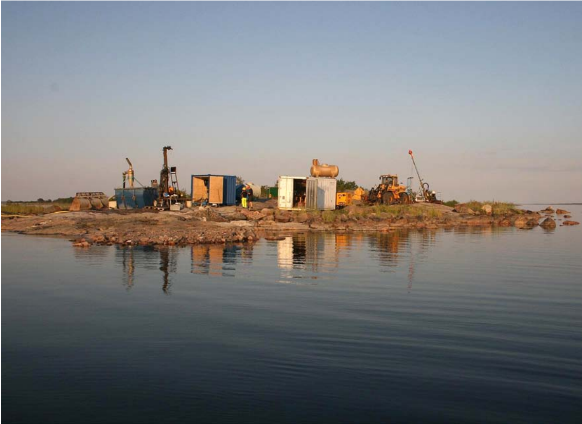
Figure 5-5. Two drilling rigs including all measurement equipment were successfully transported to the islet. To minimize the number of establishments of the flat-bottomed barge, also measurement instruments as BIPS/ radar, flow logging and air-flushing equipment were shipped to the islet during the first three weeks.
