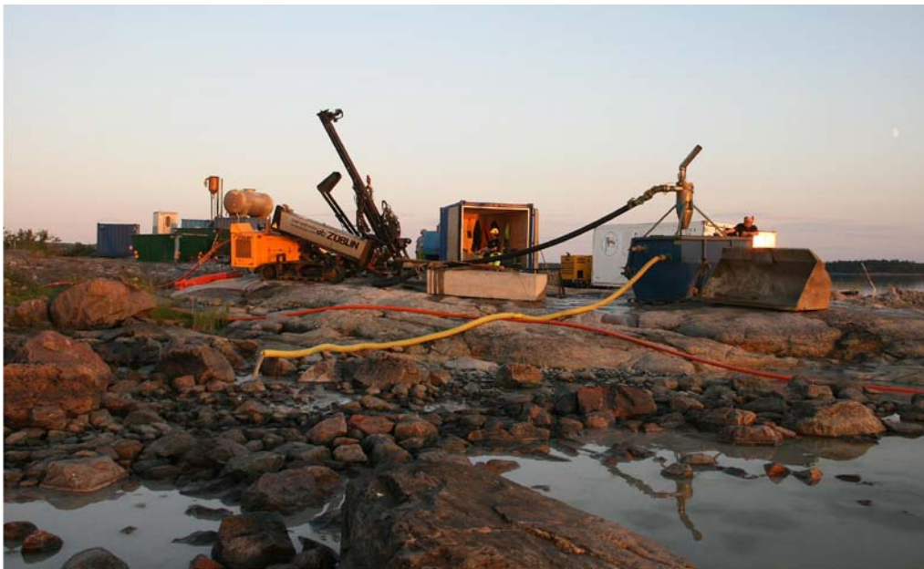
Figure 5-11. An overview of the percussion drilling of HFR106. The accumulated groundwater inflow is constantly flushed from the borehole to a container during drilling. After sampling and sedimentation in the container the water is led to the sea.
