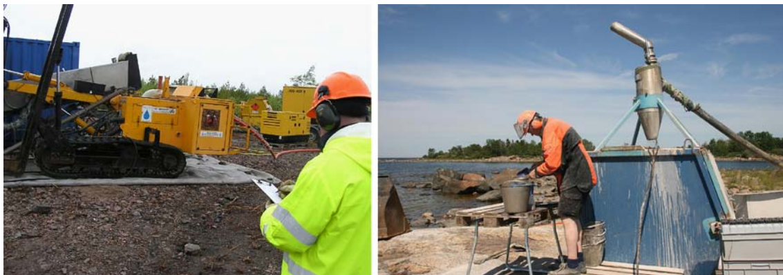
Figure 3-3. To the left, drilling penetration rate is manually measured with a stop watch, and to the right drill cuttings are sampled in a bucket of stain-less steel before placed in labeled pots.
