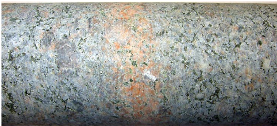
Figure 7-2. Photograph of a drill core sample with a typical, hardly visible, sealed fracture with no visible fill but with altered wall rock /Drake et al. 2006/. These fractures are presented as “No visible filling – Altered WR” in Figure 7-1 and as “NVF-AWR” in Figure 7-6 and in Figure 7-9. Drill core diameter is 50 mm.
