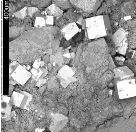
Figure 3-15. Back-scattered SEM-image of cubic pyrite crystals coating an open fracture, borehole KLX03, borehole length about 266 m.
