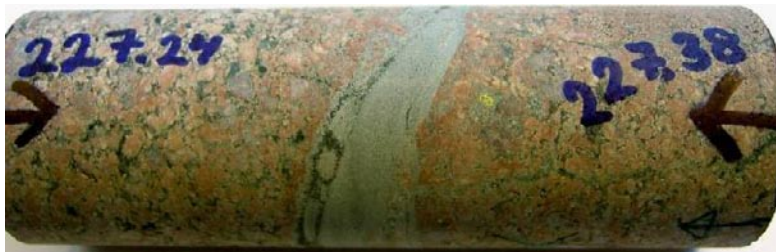
Figure 3-14. Fracture filled with prehnite. Note the red colour of the wall rock due to hydrothermal alteration. From borehole KLX07A, borehole length about 227 m. Drill core diameter is 50 mm.
