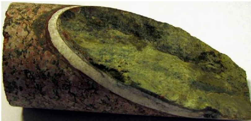
Figure 3-6. Fracture coating dominated by chlorite. The older filling is predominantly made up of calcite coated by hematite-stained adularia. KLX15A, borehole length about 570 m. Drill core diameter is 50 mm.
