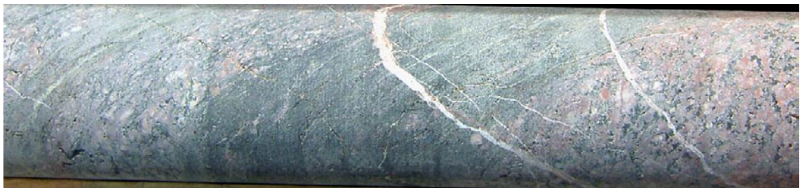
Figure 4-4. Photograph of mylonite of Generation 1 cross cut by younger fractures filled with calcite. KLX06, borehole length, about 373 m. Deformation zone ZSMEW002A. Drill core diameter is 50 mm.
