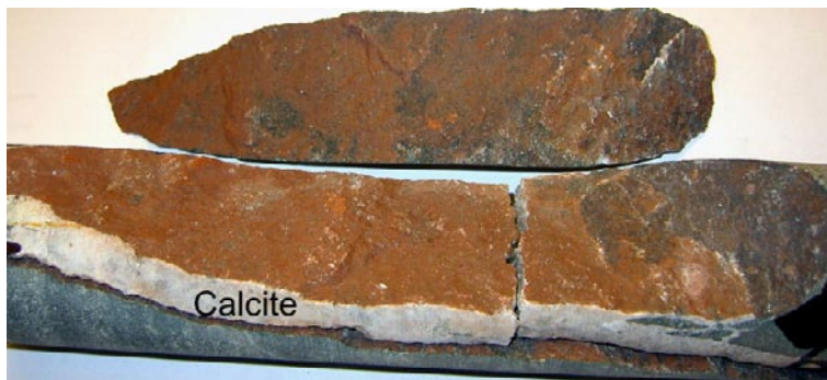
Figure 3-11. Fracture surface covered with hematite. The white fracture filling is older calcite. From borehole KLX04, borehole length about 674 m. Drill core diameter is 50 mm.
