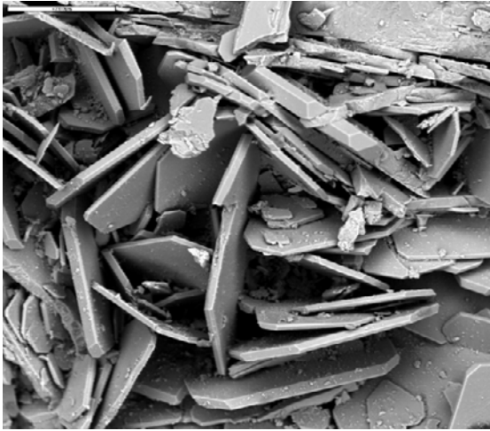
Figure 3-3. Back-scattered SEM-image of an apophyllite fracture coating. From borehole KLX03, borehole length about 970 m. Scale bar in the upper left corner is 200 \mu\text{m} .
