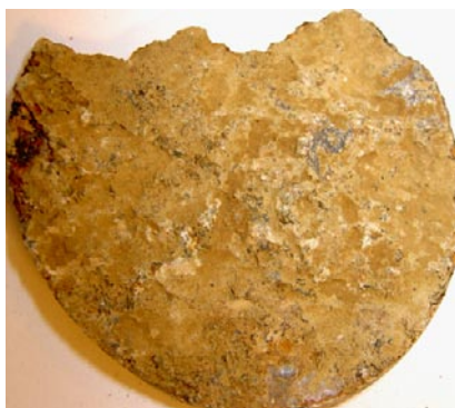
Figure 3-9. Near surface fracture coated by, for example, goethite. From borehole KLX09E, borehole length about 1 m. Drill core diameter is 50 mm.
