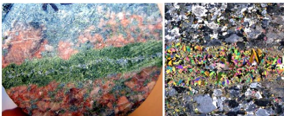
Figure 4-7. Photograph (left) and thin section viewed with crossed polars (right) of a Generation 3 fracture filled with euhedral epidote (green) with calcite and quartz (white) in the centre of the fracture. Drill core sample KLX02, 525 m borehole length. The wall rock shows heterogeneous red staining adjacent to the fracture.
