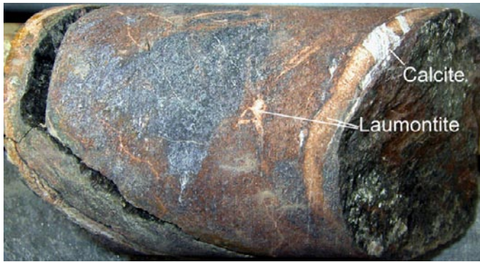
Figure 3-12. Laumontite and calcite in sealed fractures in borehole KLX06, borehole length about 400 m. Drill core diameter is 50 mm.
