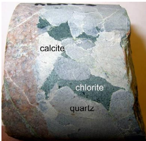
Figure 3-16. Fracture filling with chlorite (arrow), calcite (white) and quartz (grey). KLX03, borehole length about 730 m. Drill core diameter is 50 mm.
