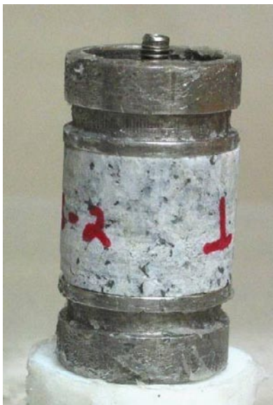
Figure 4-5. Rock core sample enclosed by end pieces of stainless steel cylinders to be used in a permeability measurement. Reproduced from /Vilks 2007b/.
