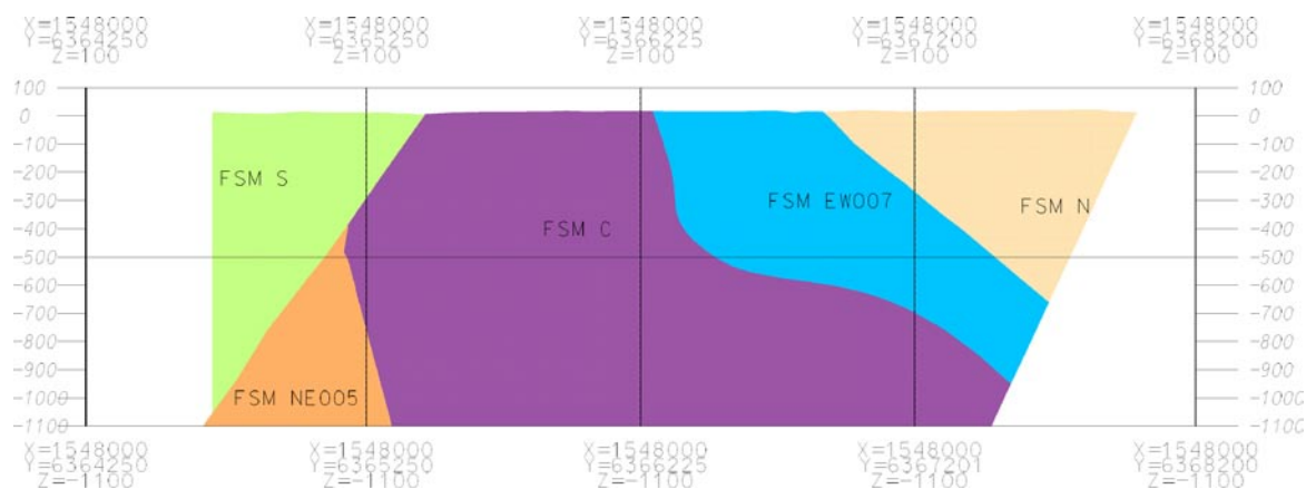
Figure 3-13. RVS cross-section, oriented north-south through the middle of the Laxemar local model volume, through identified fracture domains. Vertical section from south (left) to north at Easting's X=154,800 m. From /La Pointe et al. 2008/.
