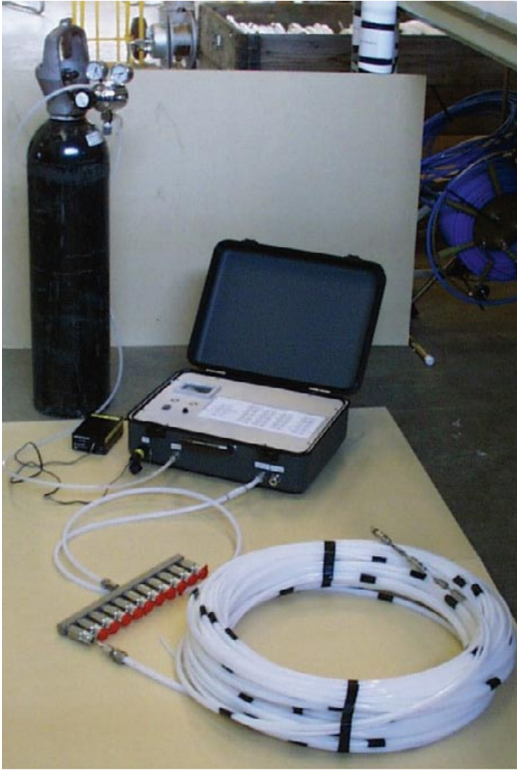
Figure 3-3. Air-lift pump equipment used in small diameter standpipes.
