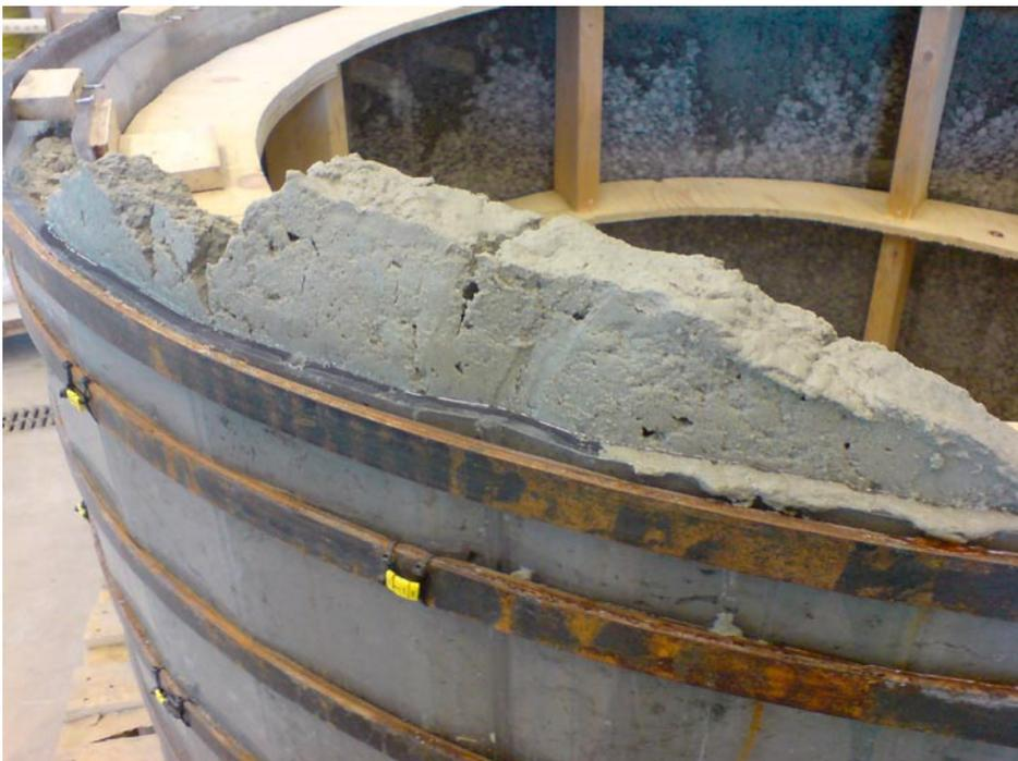
*Figure 4-16. Swelling of the bentonite above the inlet.*
