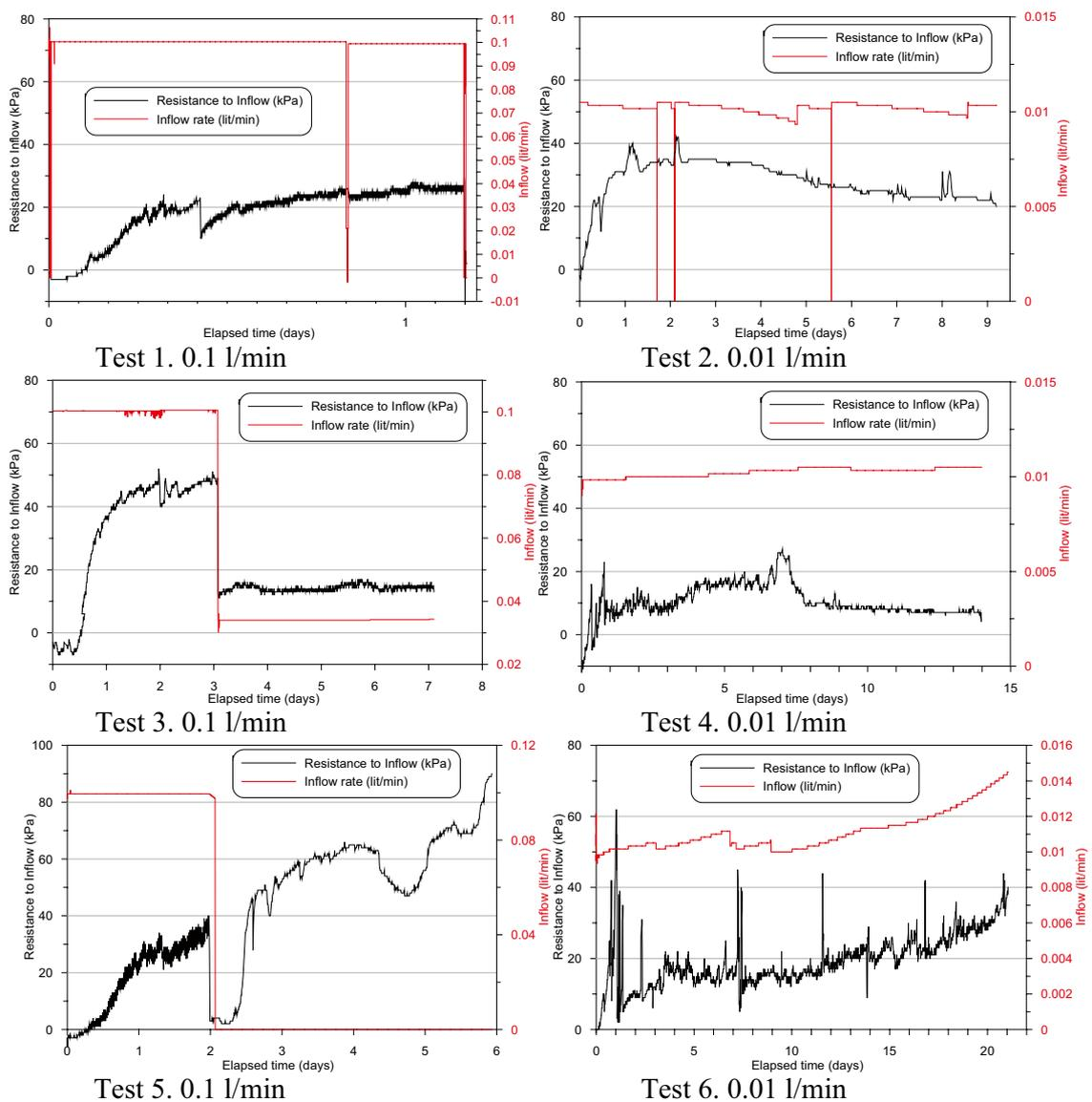
Figure 5-1. Inflow and pressure rates. Notice that the time scale differs.
