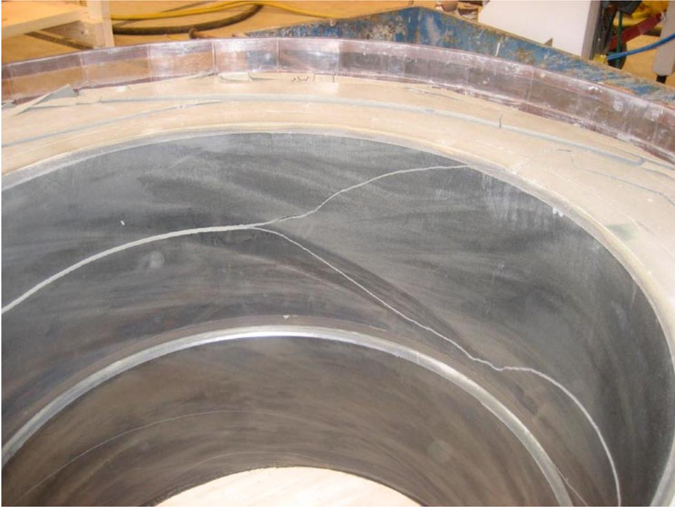
*Figure 4-24. Large cracks on the inside of the uppermost ring after 6 days.*
