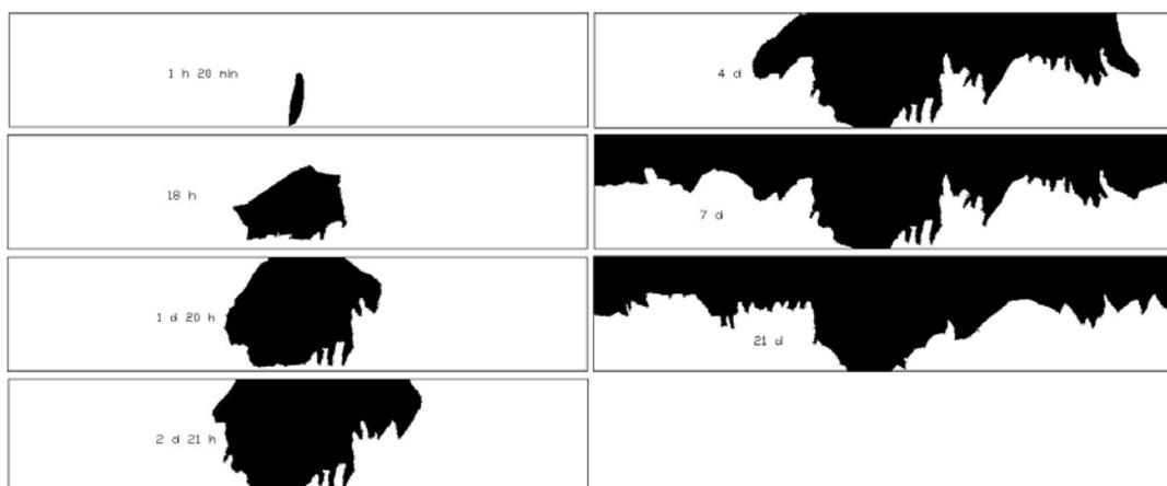
Figure 4-30. The wetting pattern in Test 6.
