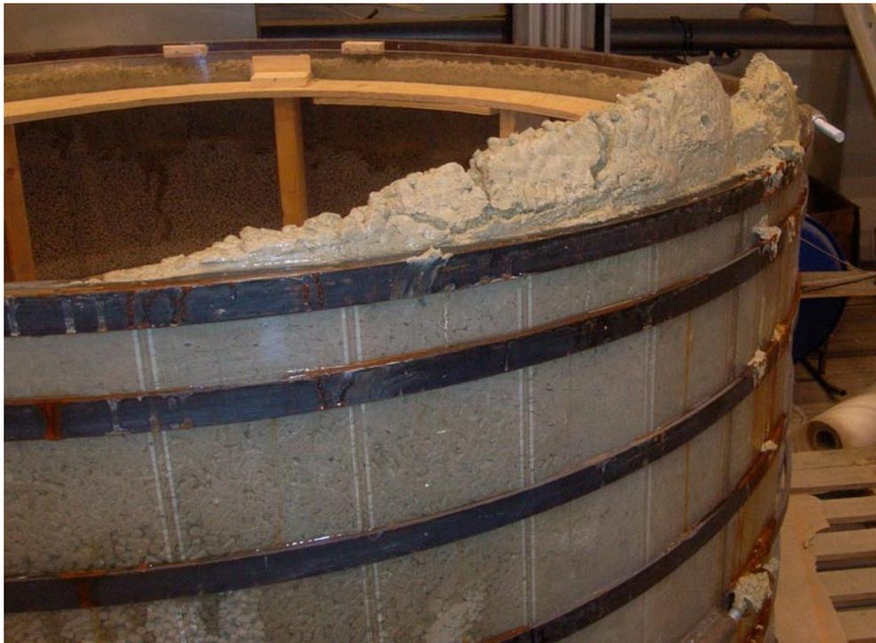
*Figure 4-6. Large swelling of the bentonite above the water inlet.*
