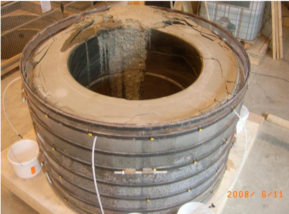
*Figure 2-8. Test with bentonite rings and pellets.*
