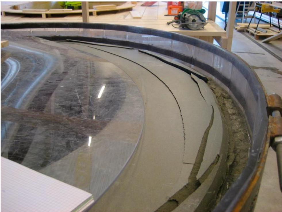
*Figure 4-23. Large cracks in the ring after 48 h.*
