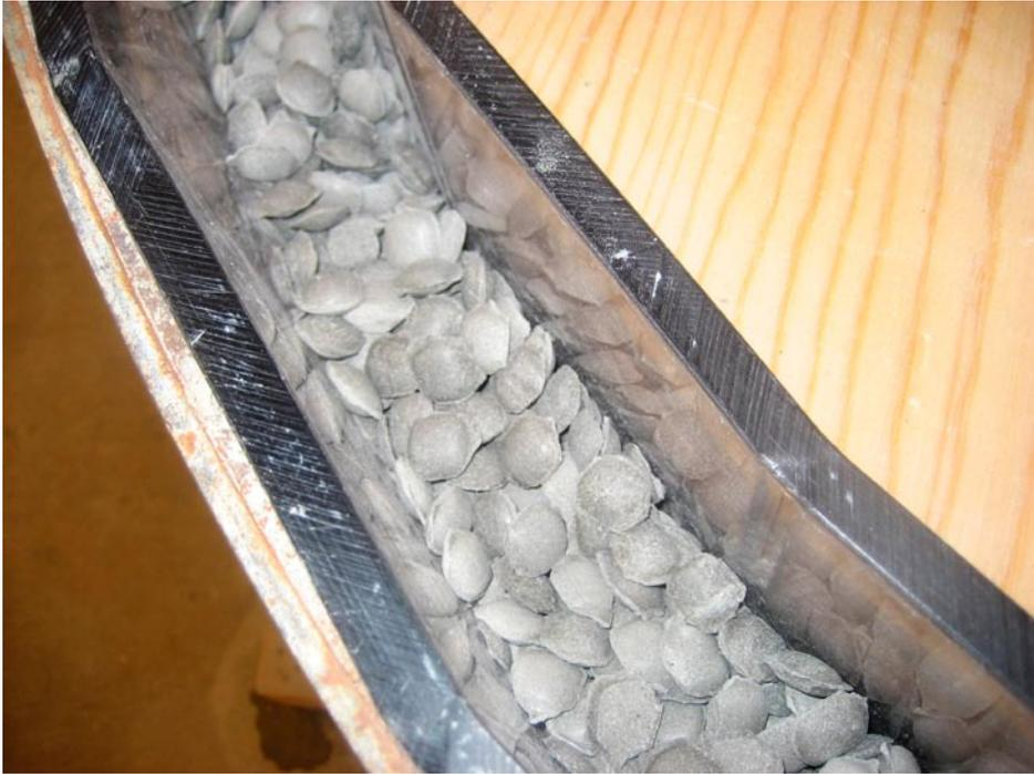
*Figure 2-7. Pellets of type MX-80 after installation. The gap is 50 millimetres in average.*
