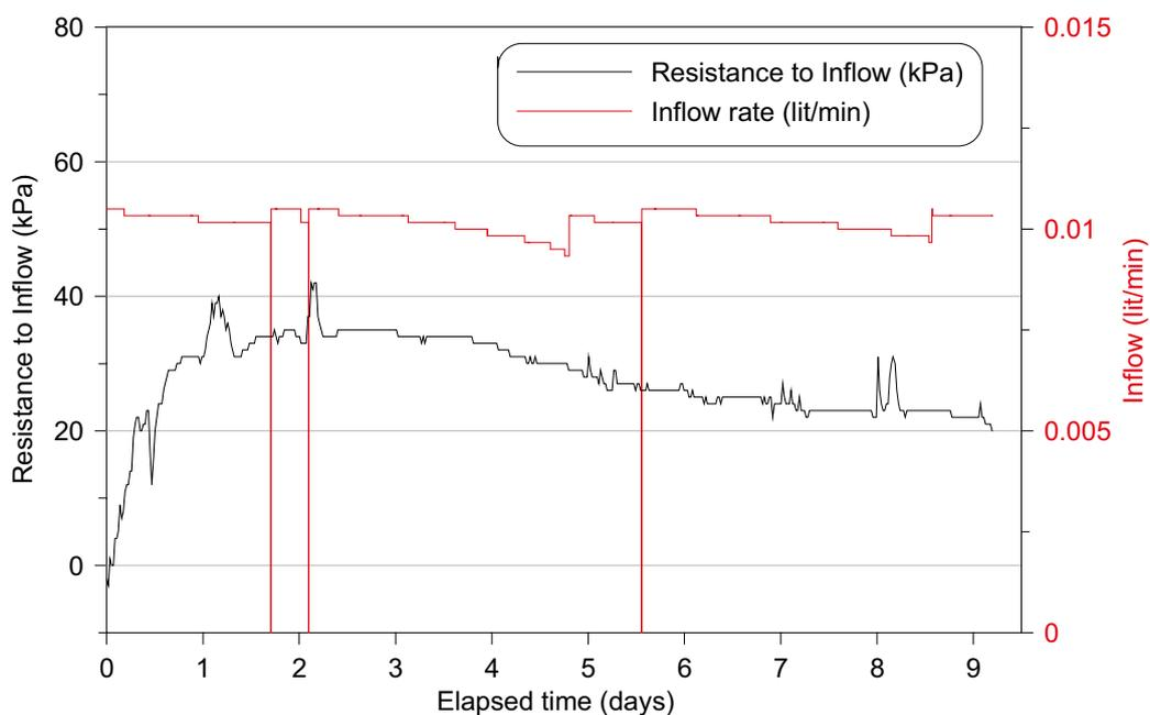
Figure 4-4. Resistance to inflow and inflow rate Test 2.
