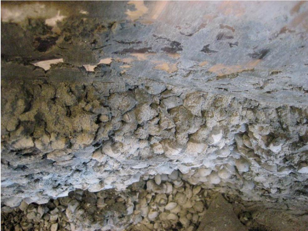
*Figure 4-40. Interface between pellets, ring and outer side of the container.*
