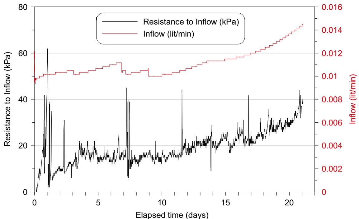
Figure 4-29. Resistance to inflow and inflow rate Test 6.
