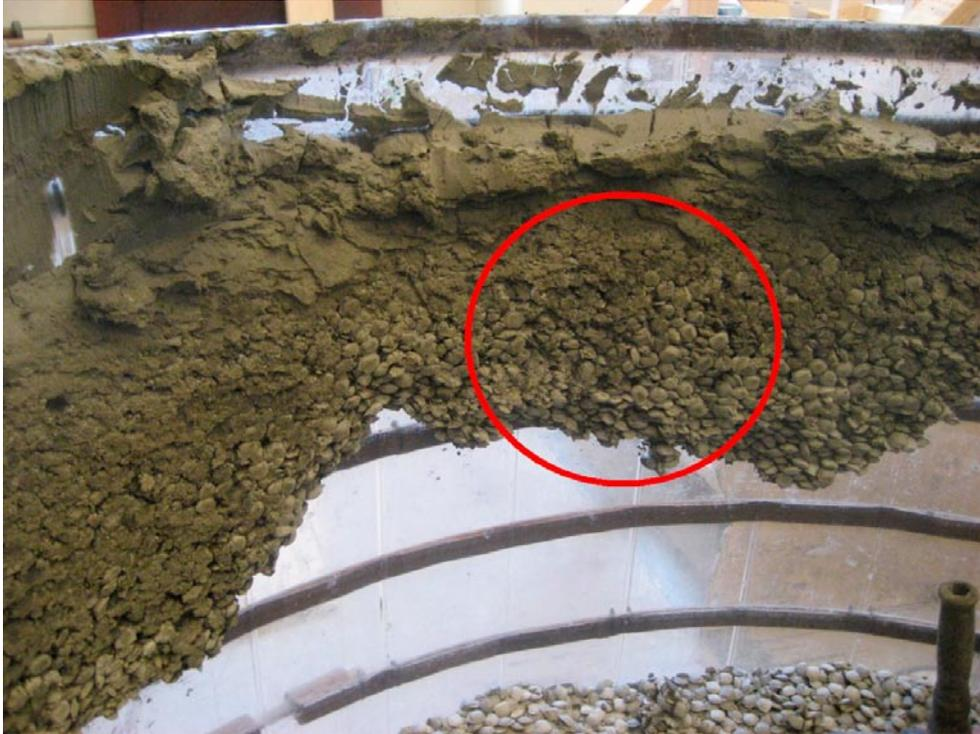
*Figure 4-42. Insider of the container with most of the pellets dry.*
