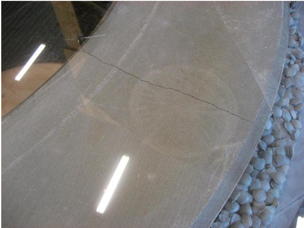
*Figure 4-21. Initial cracks in one of the bentonite rings.*
