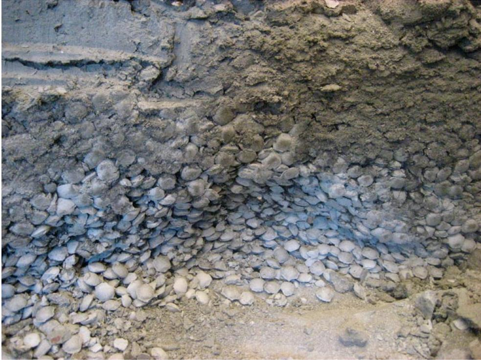
*Figure 4-38. Intact dry pellets and pellets slurry above.*
