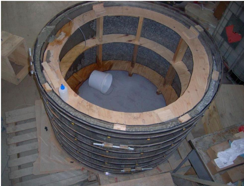
*Figure 2-6. The container with the inner cylinder used in Test 1 to 4.*
