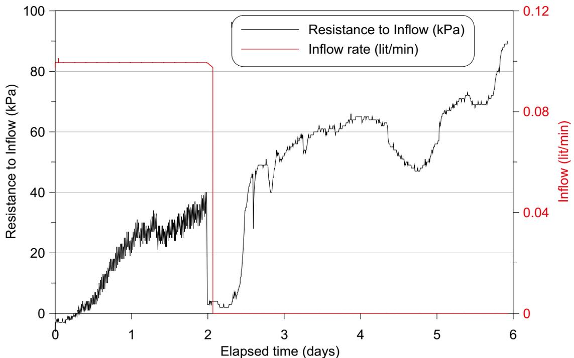
Figure 4-19. Resistance to inflow and inflow rate Test 5.
