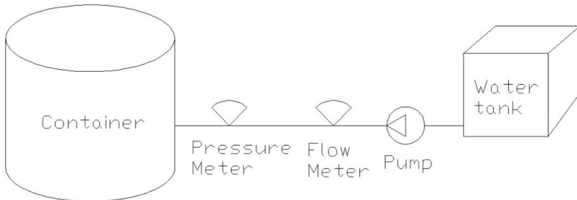
*Figure 2-3. Sketch of the test setup.*
