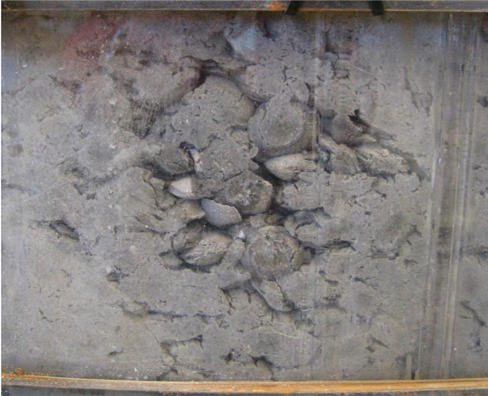
*Figure 4-10. Almost intact pellets surrounded by finer material can be seen after seven days.*
