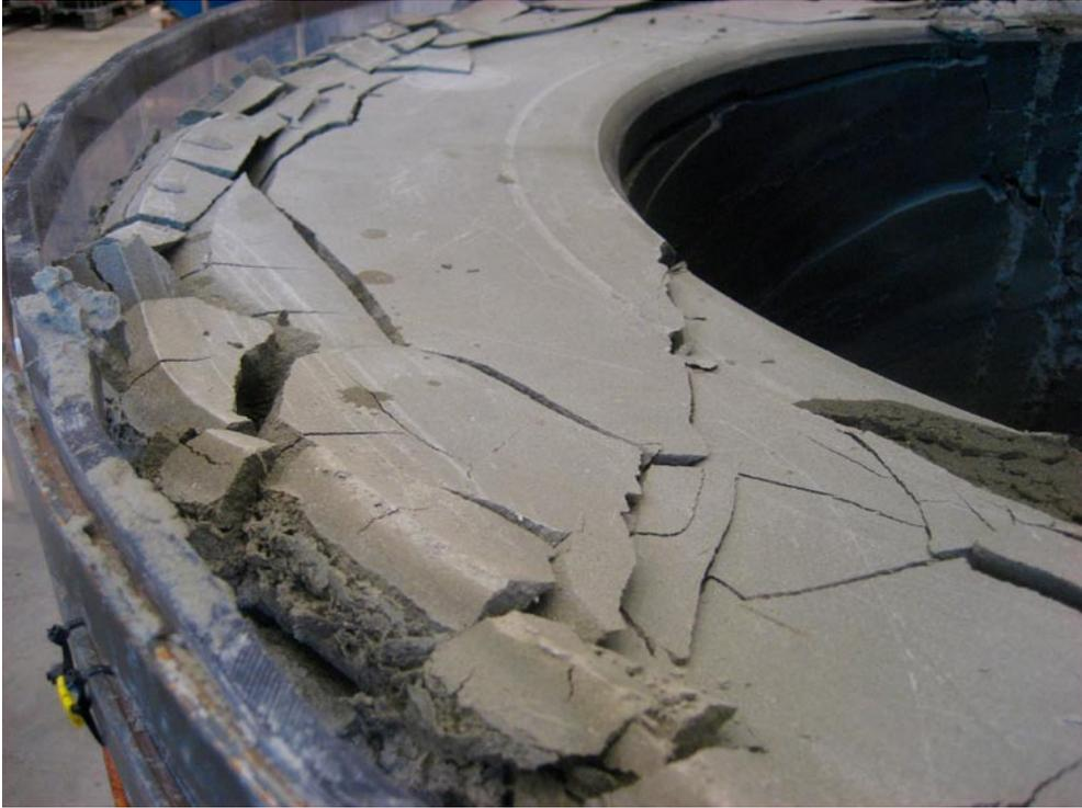
*Figure 4-34. Major cracks occurred in the uppermost ring.*
