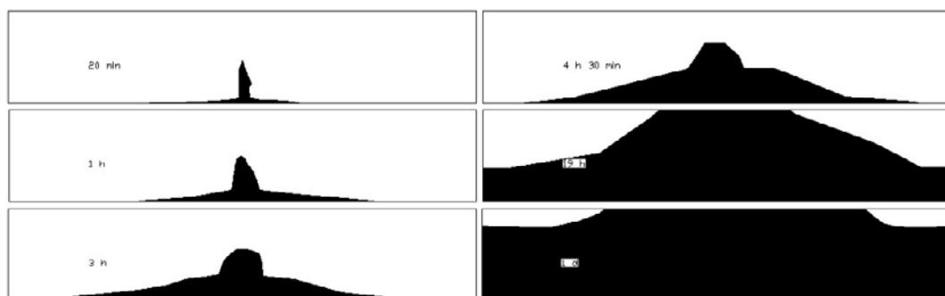
Figure 4-2. Wetting pattern in Test 1. The black area is wet and the side of the container is projected as on a flat piece of paper with the position of the water inlet in the midpoint.
