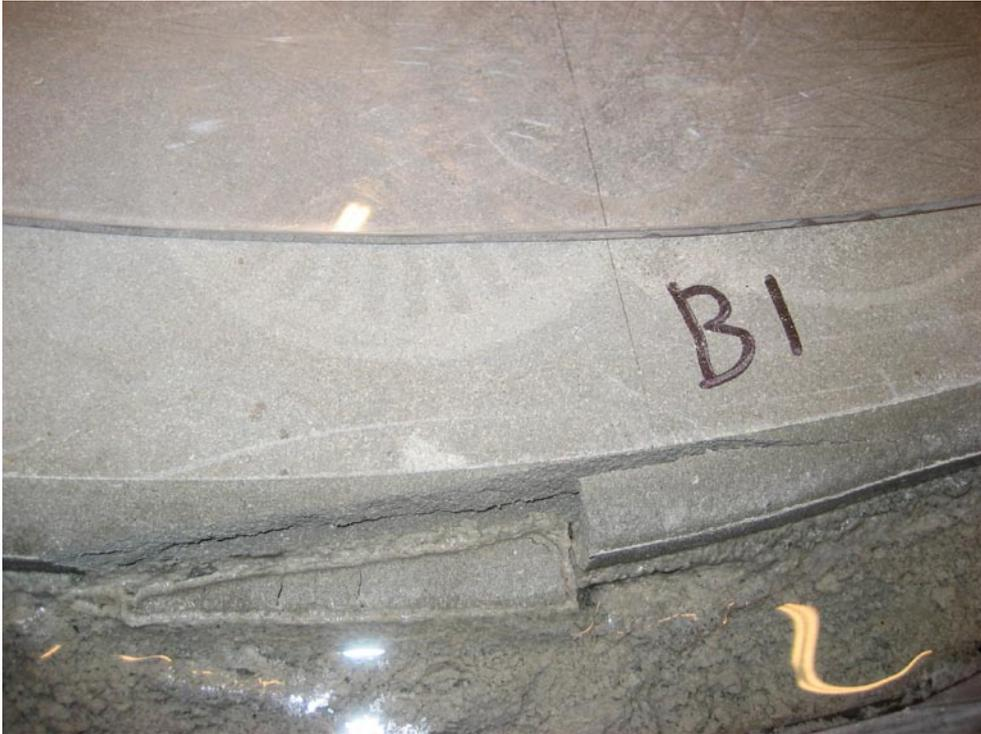
*Figure 4-22. Cracks on the outer side of the ring after about 24 h. Note that the plastic lid is visible above the text B1.*
