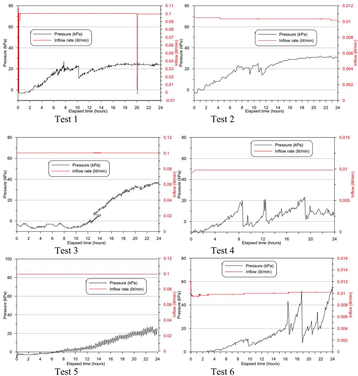
Figure 5-2. The inflow rates and pressures the first 24 h.
