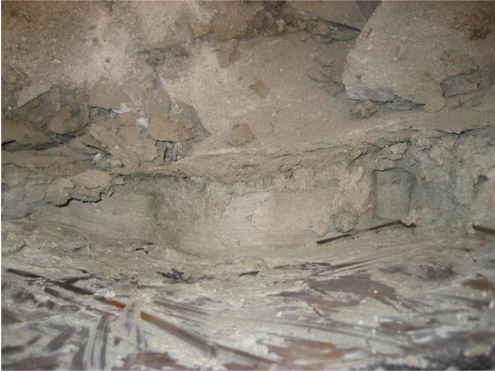
Figure 4-26. Bentonite ring, bentonite slurry and container wall during dismantling.
