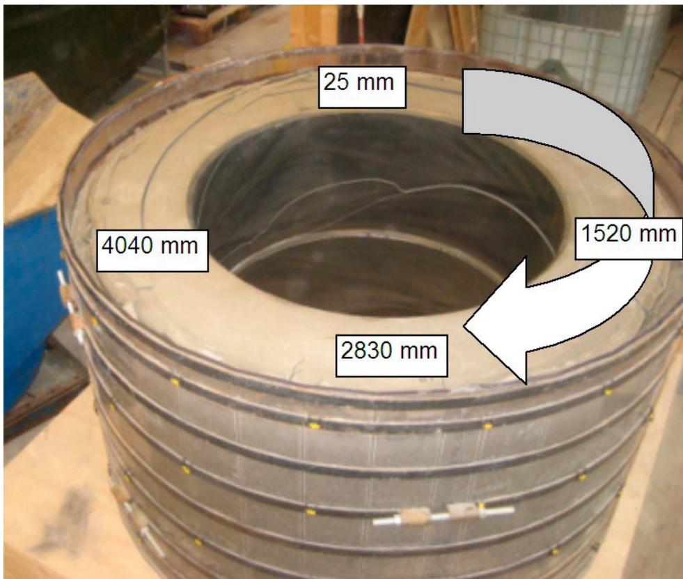
**Figure 4-28.** The positions of the samples are measured clockwise from the water inlet.
