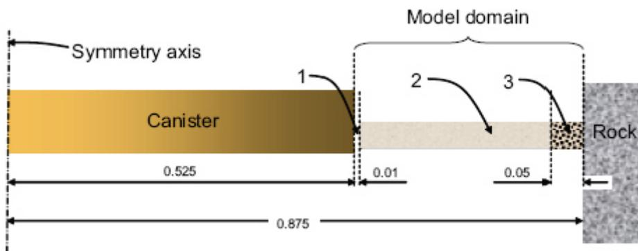
*Figure 2-1. A section of a deposition hole with canister, bentonite ring and pellets in the KBS3-V-concept /SKB 2008/.*
