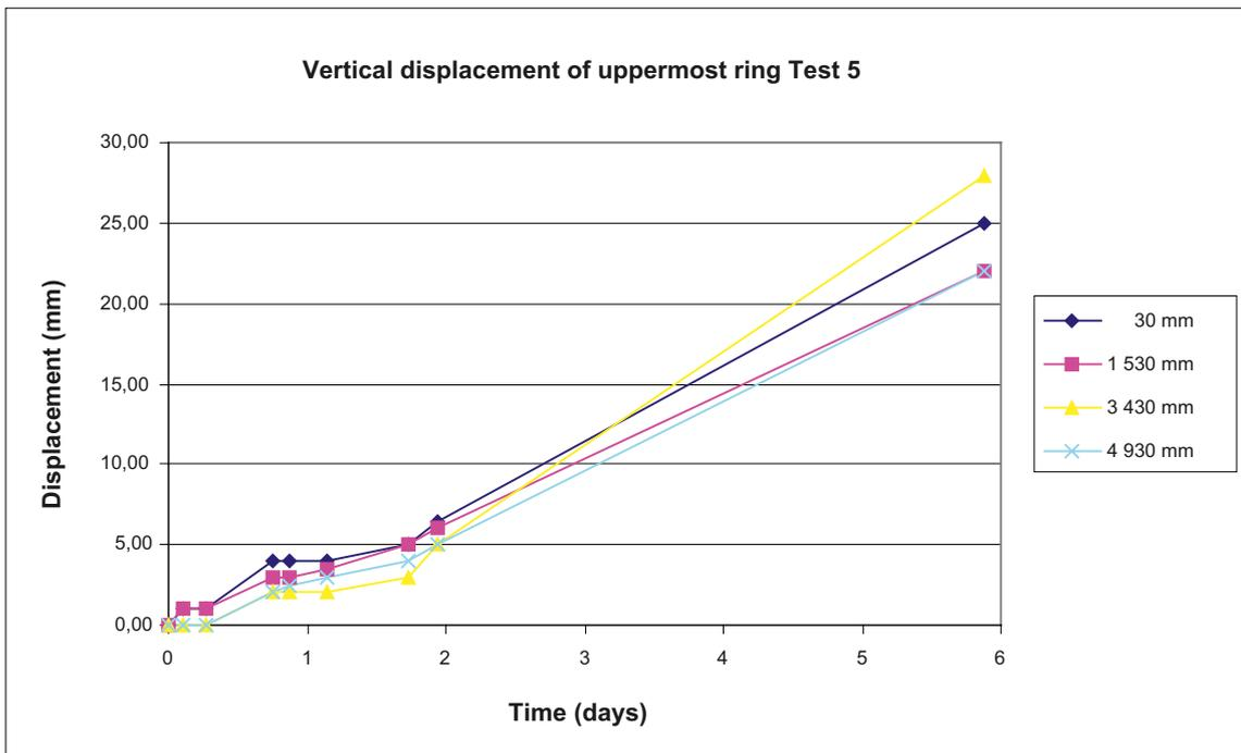
Figure 4-27. Vertical displacement of the uppermost ring in Test 5. The positions are measured clockwise from the water inlet around the circumference of the container with the water inlet at 0 mm.
