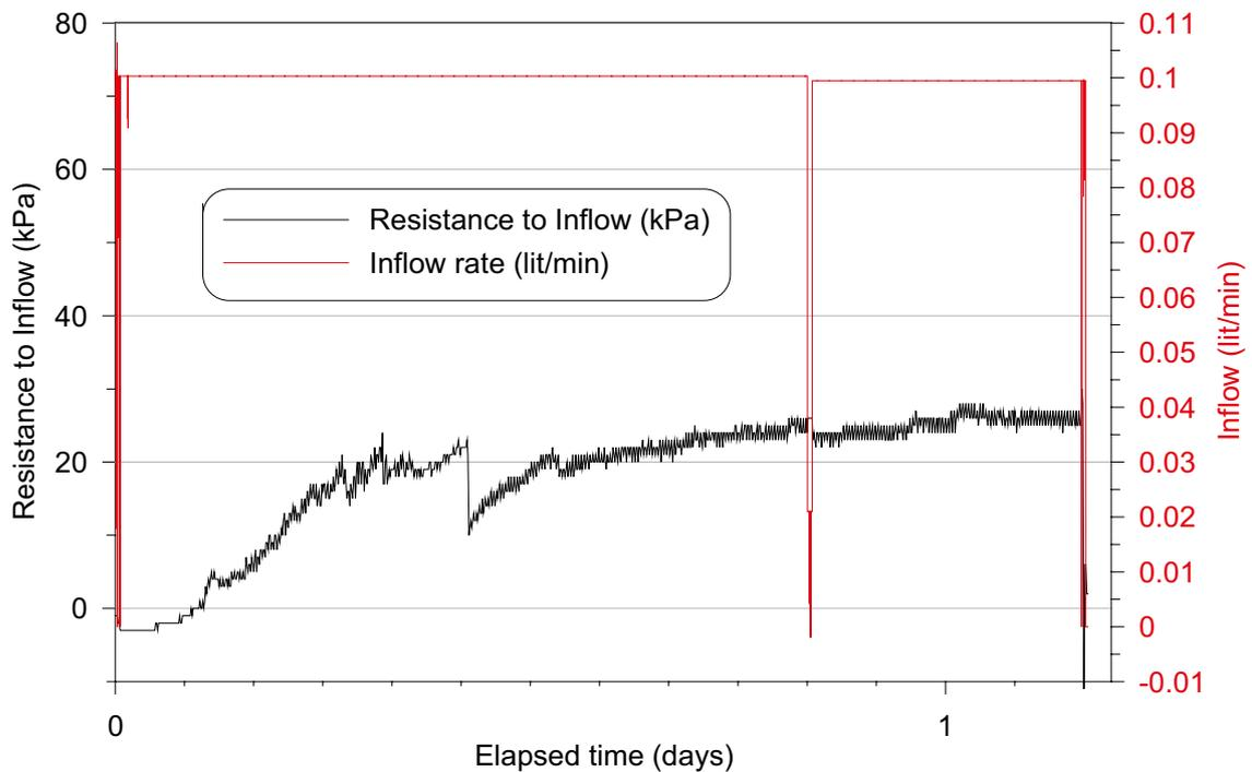
Figure 4-1. Resistance to inflow and inflow rate Test 1.
