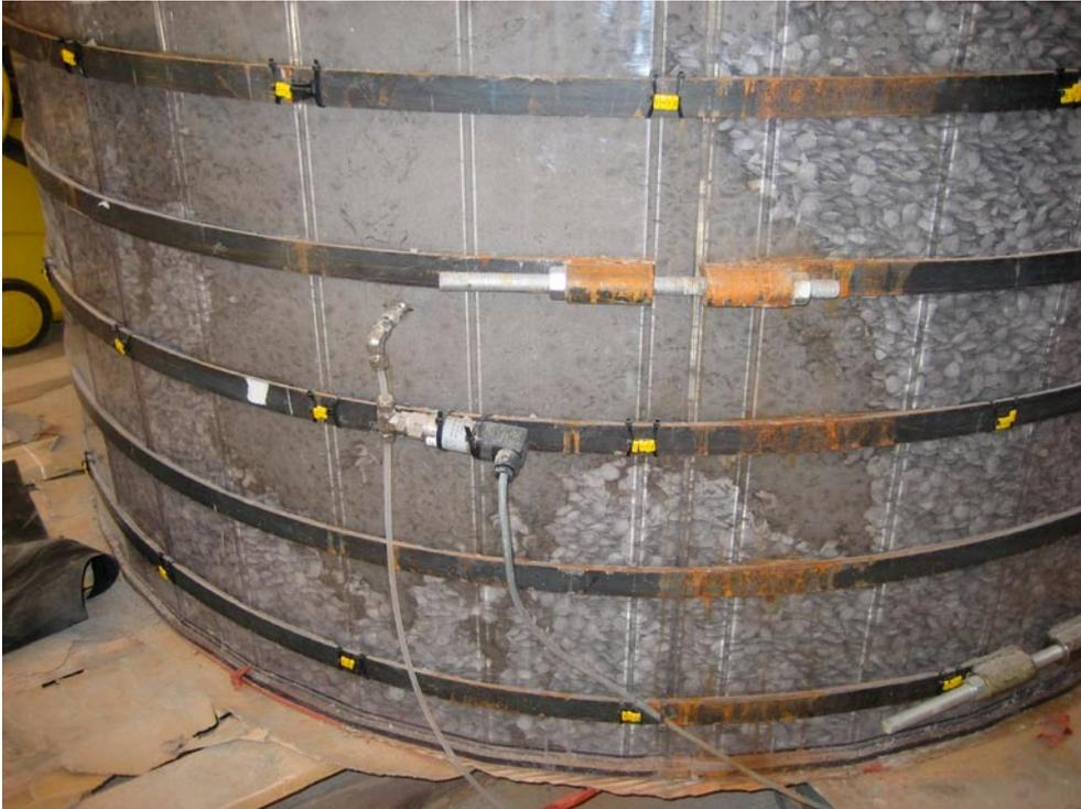
*Figure 2-9. Water inlet and pressure meter. The water pathway and the wetting of the pellets can be observed as darker areas through the container wall.*
