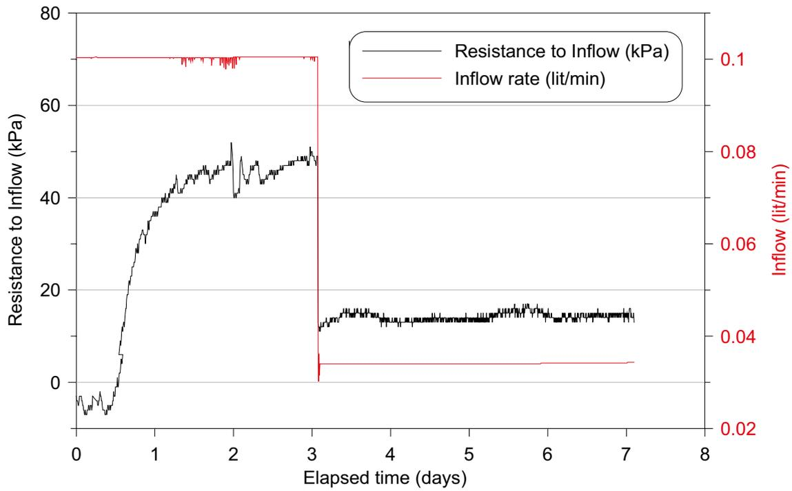
Figure 4-7. Resistance to inflow and inflow rate Test 3.
