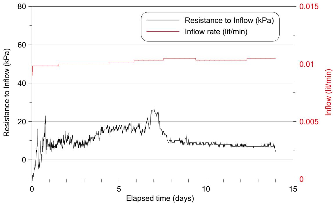
Figure 4-12. Resistance to inflow and inflow rate Test 4.
