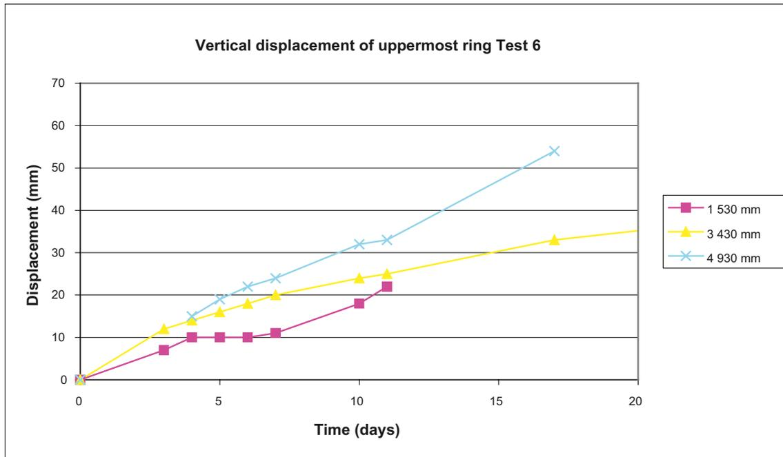
Figure 4-31. Vertical displacement of the uppermost ring in Test 6. The positions are measured clockwise from the water inlet around the circumference of the container with the water inlet at 0 mm.
