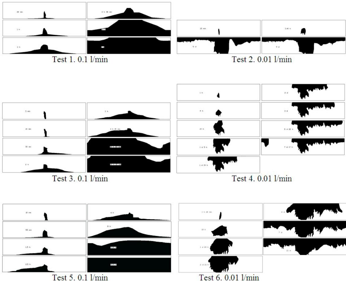
Figure 5-3. Wetting patterns for Test 1-6.
