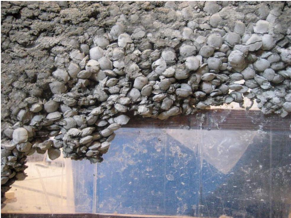
*Figure 4-39. Distinct difference between dry and wet pellets.*
