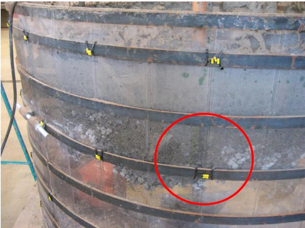
*Figure 4-41. Outside of the container with wet pellets.*
