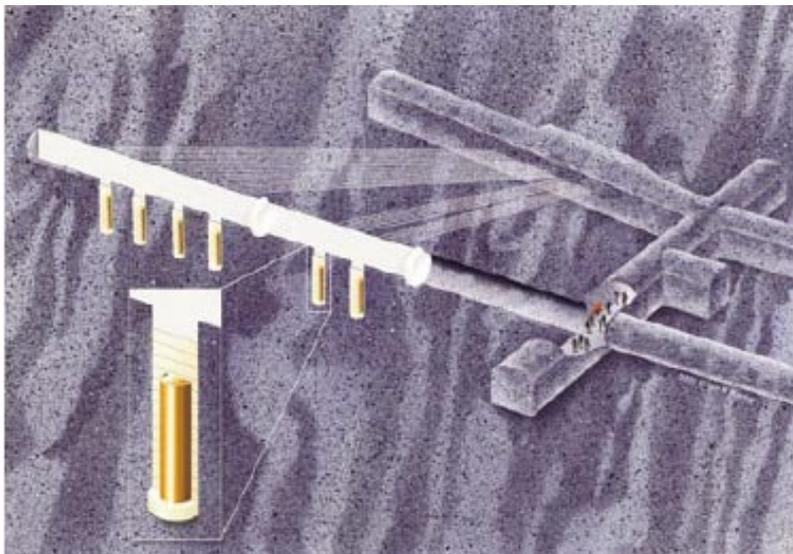
*Figure 1-1. Schematic view of storage of canisters in the KBS-3V concept /SKB 2008/.*
