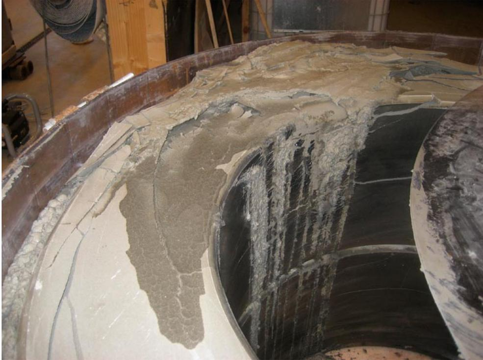
*Figure 4-32. Bentonite slurry on top of the ring.*
