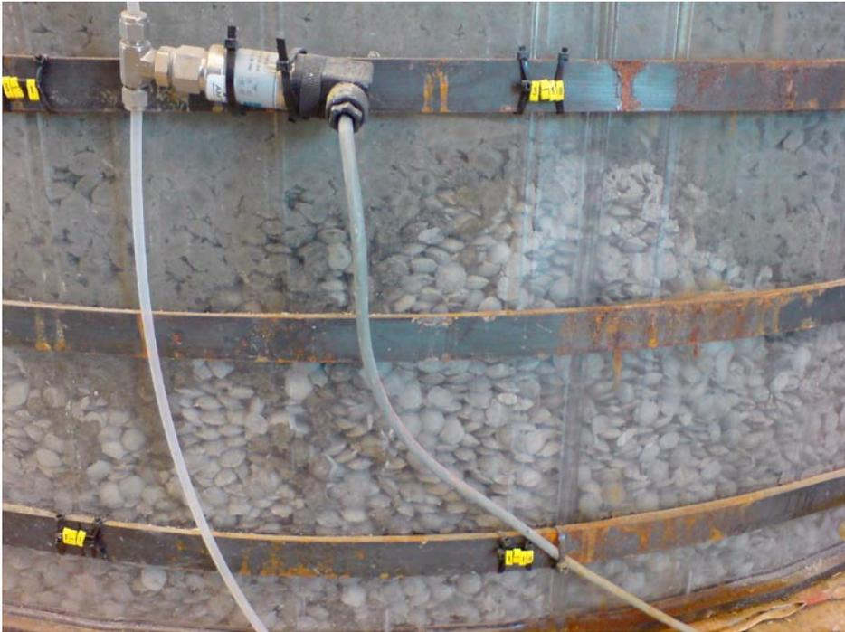
*Figure 4-15. Dry pellets below the inlet at the end of the test.*
