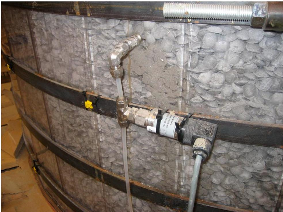
*Figure 2-4. Water inlet and pressure meter at the container.*
