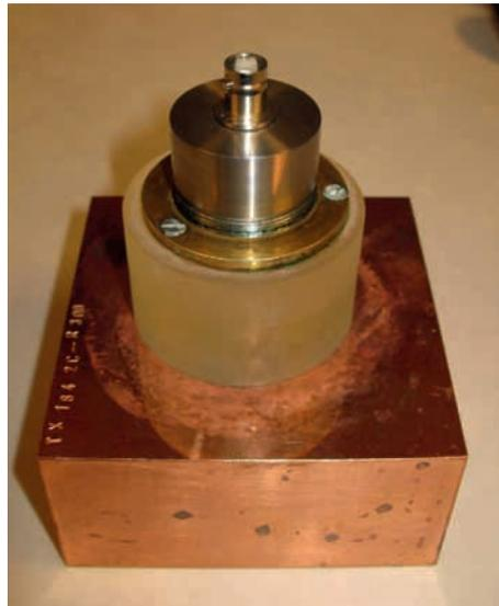
**Figure 2.4:** Buffer rod setup used for the attenuation evaluation.
