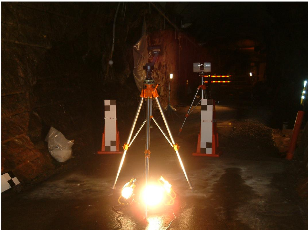
*Figure 14. The SpheroCam HDR high resolution camera mounted on a tripod with the ring of flood lights needed for illumination underneath. In the background the laser scanner on its second tripod.*
