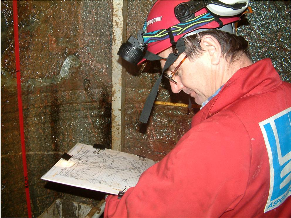
*Figure 21. Field mapping of deposition hole. The mapping is performed on plastic coated paper.*
