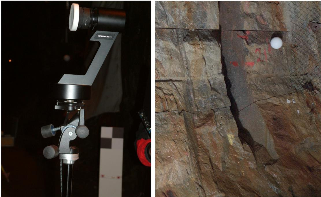
*Figure 6. To the left the high resolution line-camera, SpheroCam HDR To the right a colour scan showing a part of the TASQ tunnel wall.*
