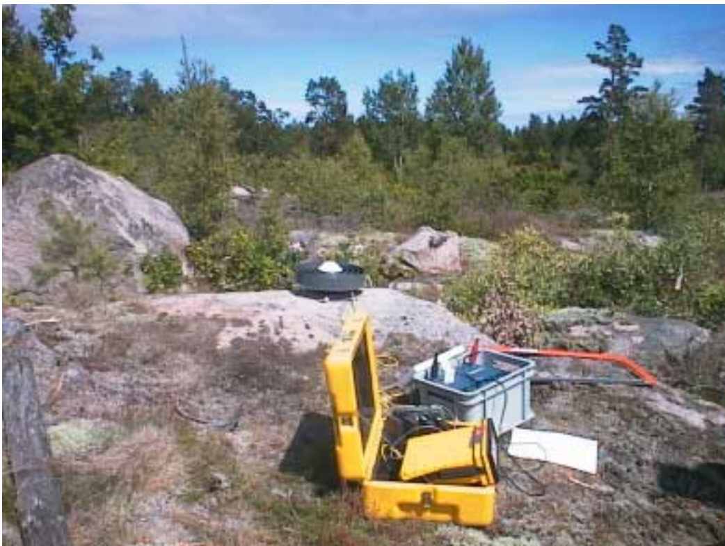
Figure 1-4. The chokering antenna with a Trimble GPS receiver at site Knip in June 2000.
