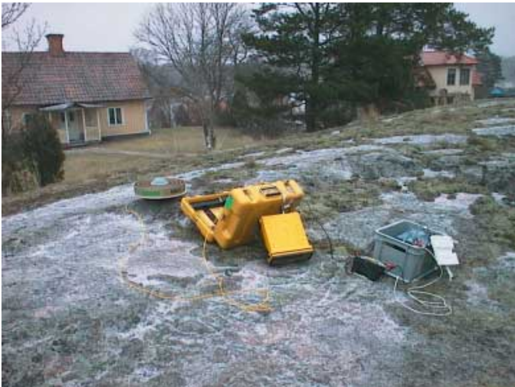
Figure 2-2. The receiver at the site Karr in the February campaign of 2002 was knocked down somehow and it lost eight-hour data.
