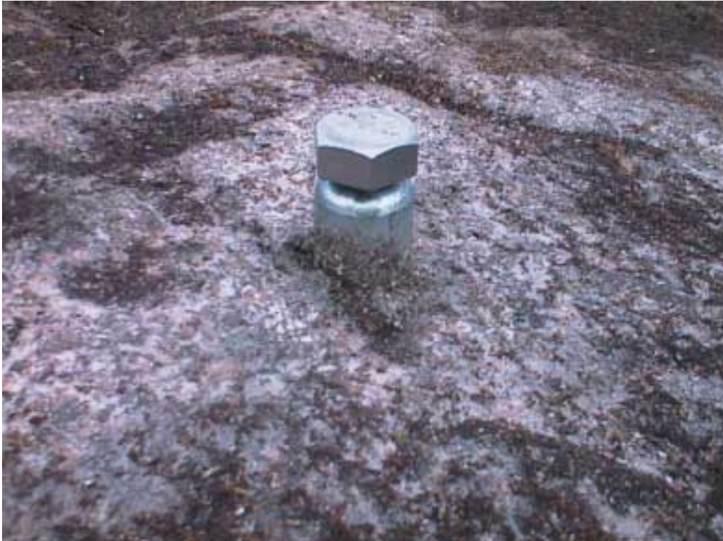
Figure 1-3. The steel screw components fixed to the rock.
