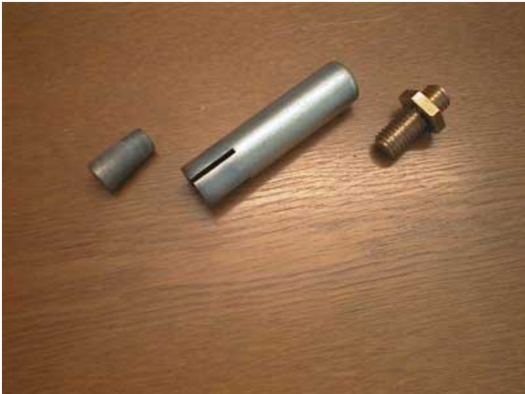
Figure 1-2. The steel components used to install an antenna on the ground.
