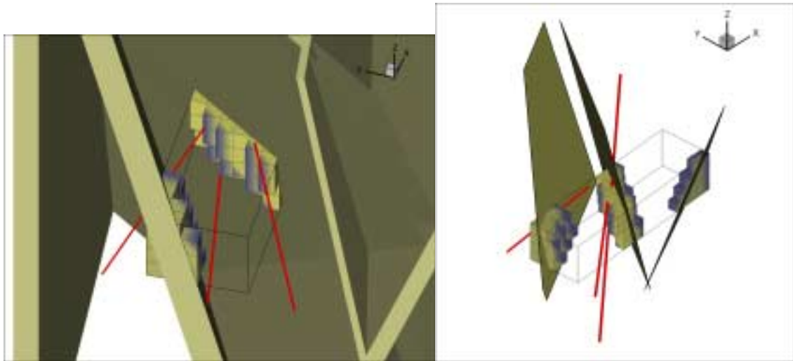
Figure 7-2. 3D views of the determination of the cubes intersected by deformation zones. A) Detail of the RVS model. B) Overview of the models with only "deformation zone unit" cubes enlightened. NB: deformation zones are then represented as planes with zero width.
