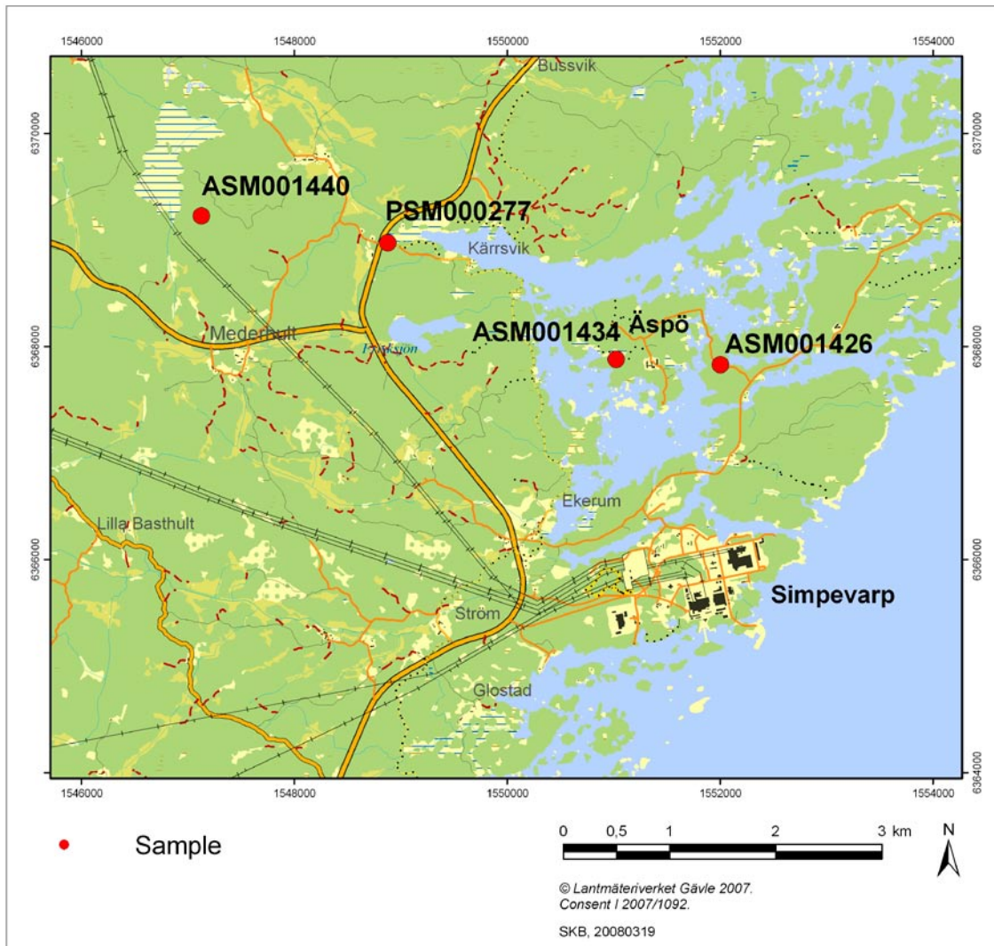
Figure 3-2. Location of the four sampled sites in Laxemar-Simpevarp. The properties of the sites are shown in Table 3-1. Site C (ASM001426) is sandy till, Site D (ASM001434) is clay gyttja, Site E (ASM001440) is peat and Site F (PSM000277) is clay gyttja.
