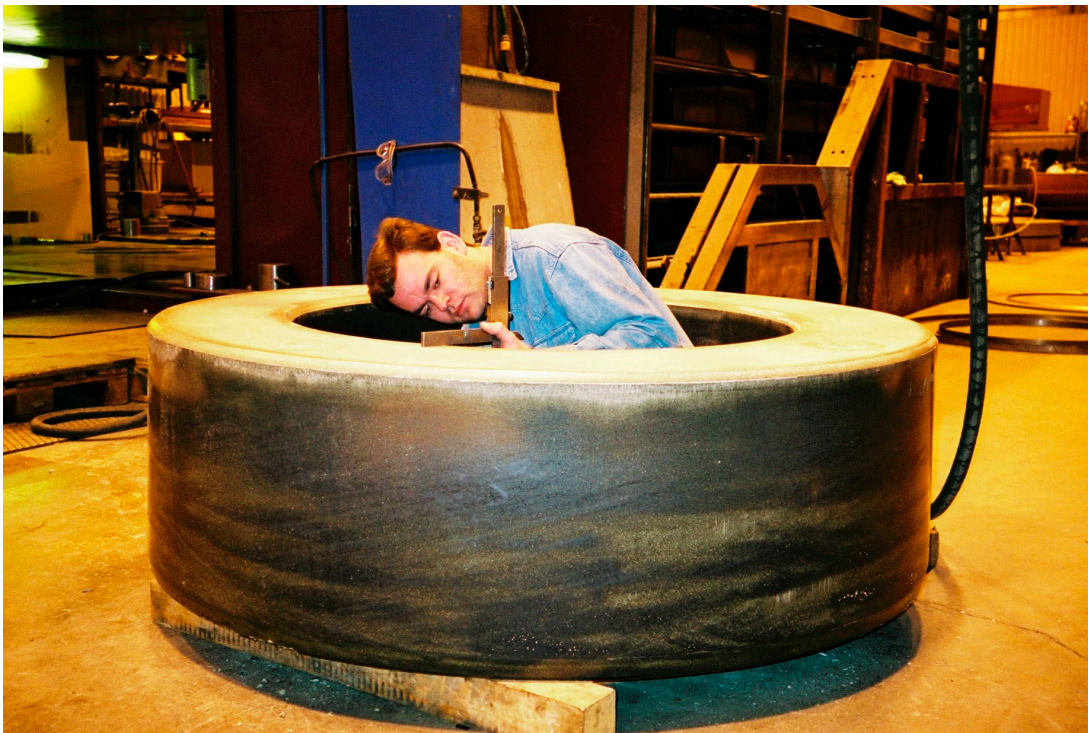
Figure 2-7. The height of the bentonite block is measured.
