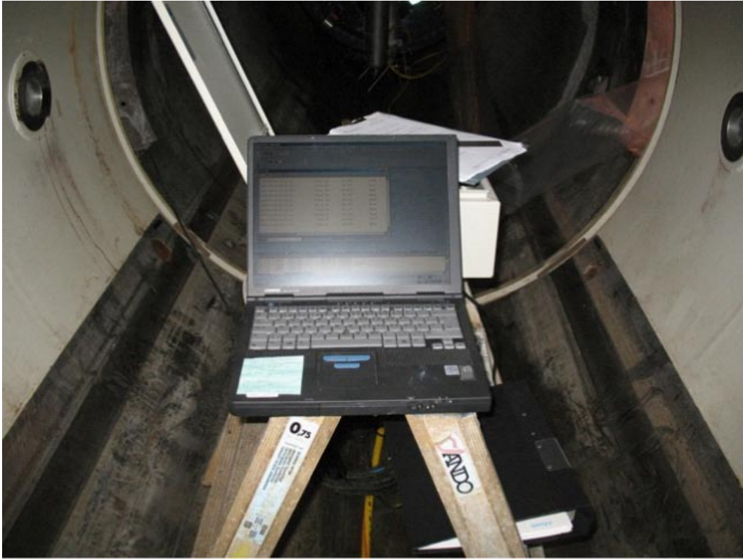
Figure 3-2. Logging during the ground water pressure build up test.
