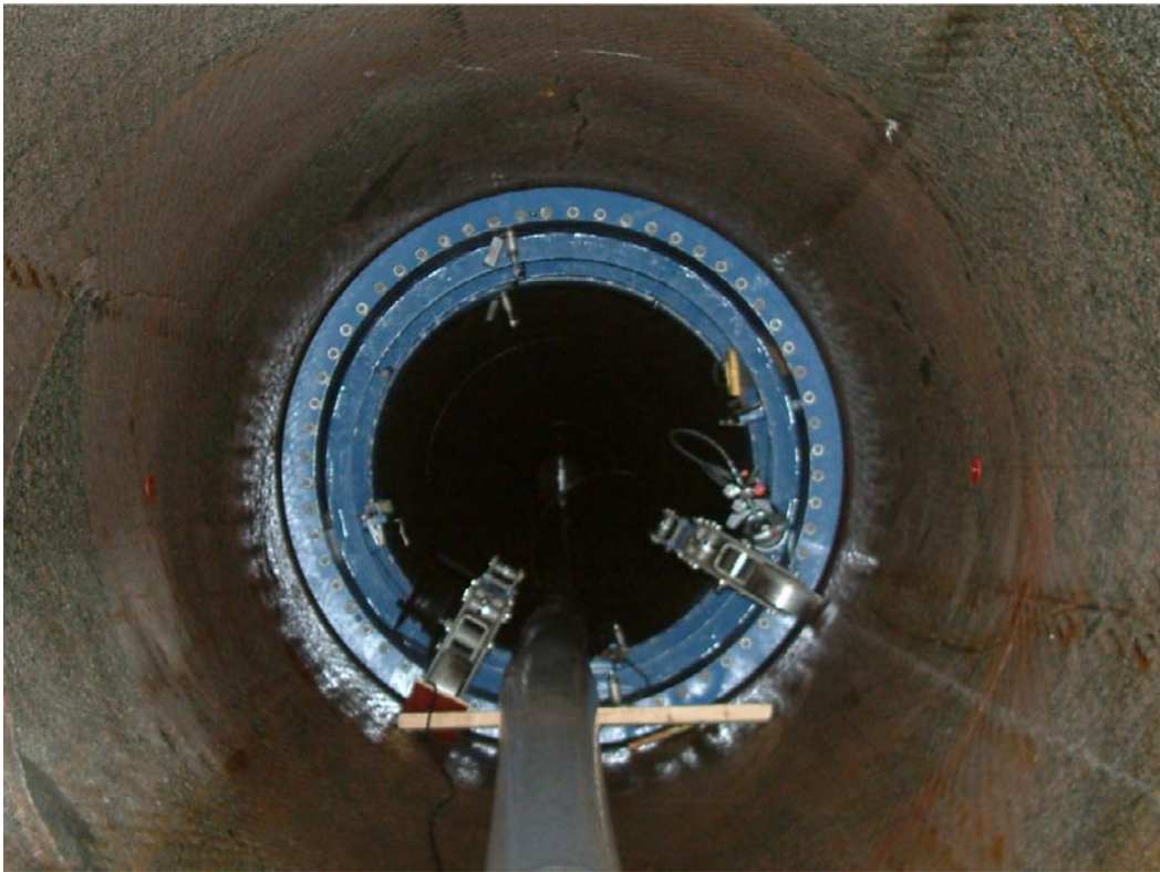
Figure 3-3. The Mega-Packer in the drift. The position of the wheels tells that there has been a rotation of about 15 degrees.
