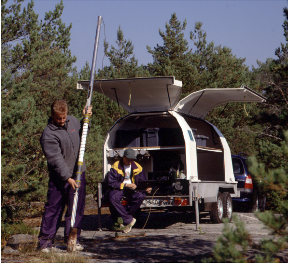
Figure 2-2. The Posiva difference flow meter. A spiral structure is installed within the yellow rubber disks.
